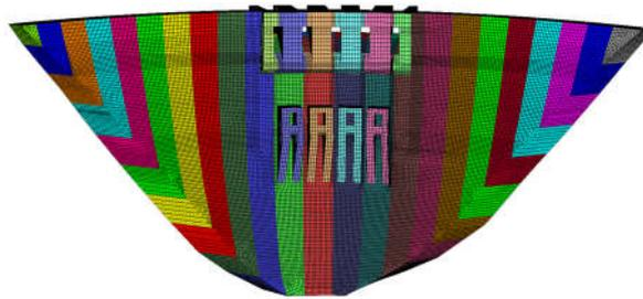
Figure 12. Finite element model of a high arch dam for seismic damage analysis
