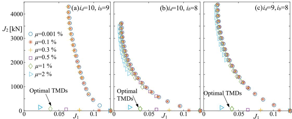
Figure 4. Pareto front for design problem  $D_2$  for three different topological configurations for the TMDI implementation (sub-plots) and six different mass ratios masses (curves for each subplot)
