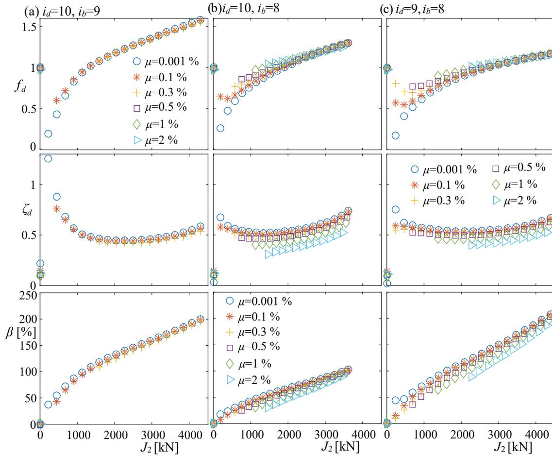
Figure 3. Optimal values for  $f_d$ ,  $\zeta_d$  and  $\beta$  along the Pareto front [design variables are plotted with respect to the corresponding value of  $J_2$ ]. Rows corresponds to three different topological configurations. Curves in each subplot correspond to different mass ratios.
