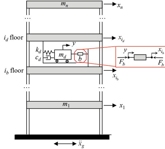
Figure 1. Tuned mass-damper-inerter (TMDI) equipped multi-storey frame structure.
