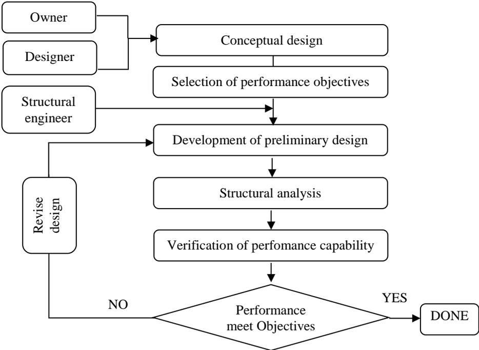
Figure 1. Flow chart of performance based seismic design
