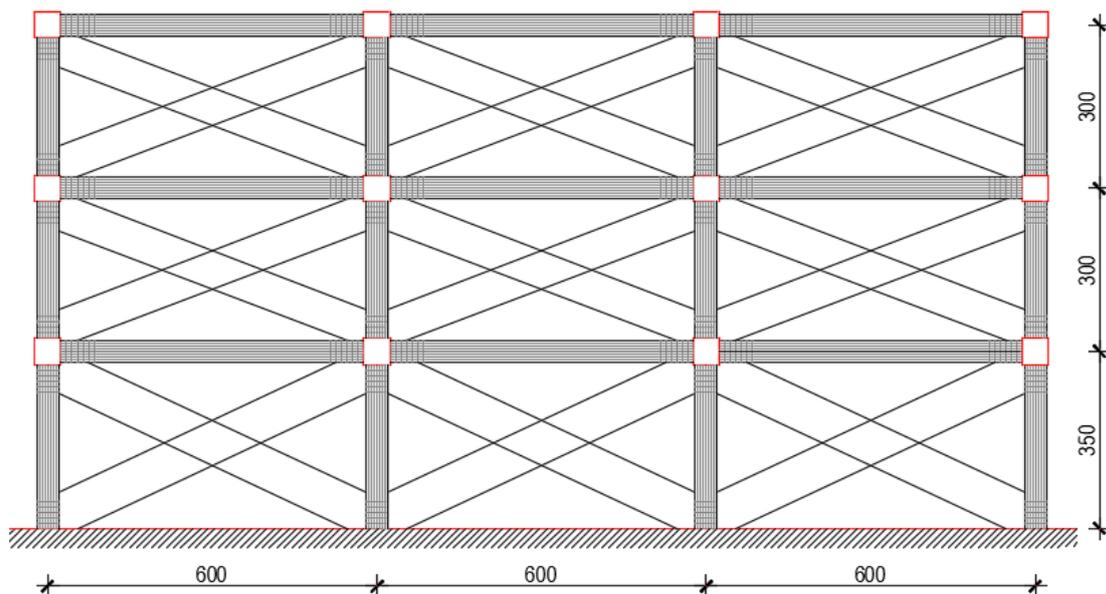
Figure 6. Numerical models for 3-storey building model with 6m bay length
