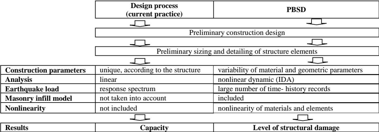
Figure 2. Comparison of current design practice and Performance-Based Seismic Design (PBSD)
