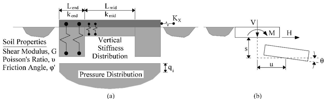
Figure 1. (a) Graphical representation of BNWF model and associated study parameters and (b) nomenclature for displacements and loads (Source: Harden and Hutchinson 2009)
