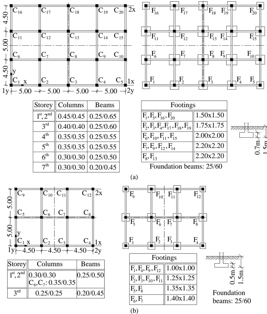
Figure 2. Plan-view, dimensions of the R/C members and foundation system of buildings SFxy-3 (a) and SFxy-7 (b)
