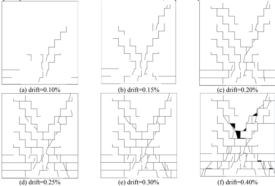
It can be observed that in general, the value of the  $FD^{XBCM}$  increases as the cracks grow with increasing drift ratios. This is due to the fact that  $FD^{XBCM}$  values are computed based on the position of the mask where the number of intersected boxes is maximum. Moreover, for a given mask size, by increasing the
