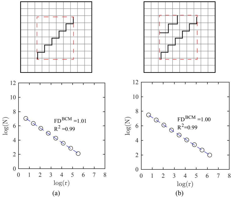
Figure 1. Crack maps and the corresponding  $FD^{BCM}$
