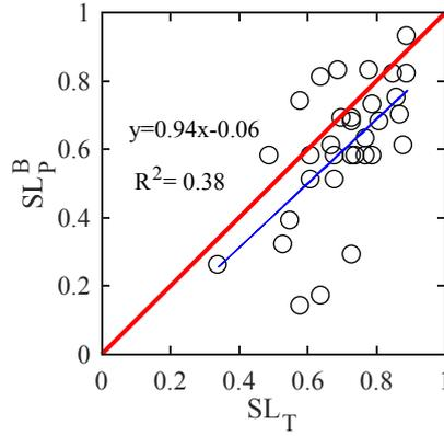
Figure 7. Graph of stiffness loss ratio obtained in the test and predicted by BCM
