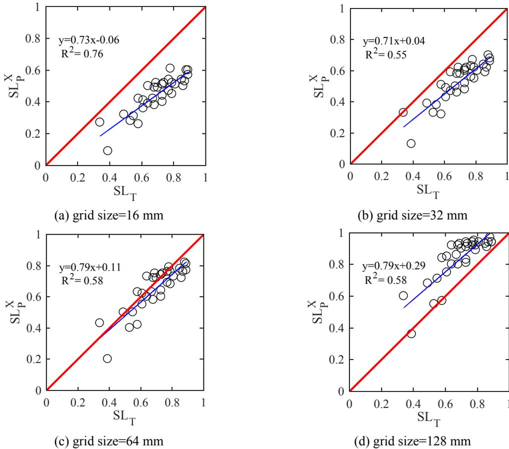
Figure 8. Graph of stiffness loss ratio obtained in the test and predicted by XBCM
