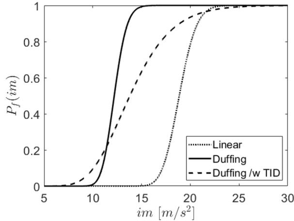
Figure 3. Fragility functions calculated for  $x_{cr} = 0.035$
