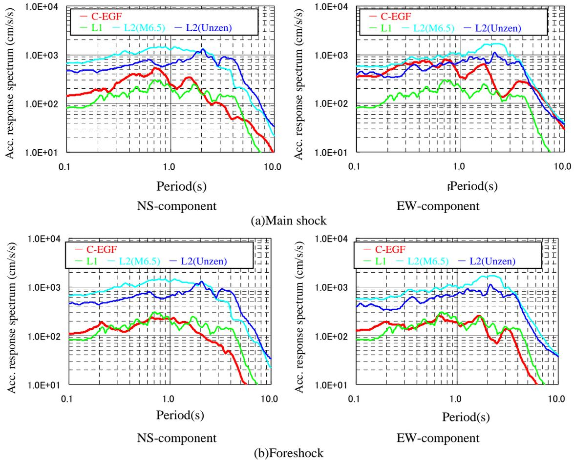
Figure 9. Comparison of Estimated and Design Strong Ground Motions (Acceleration response spectrum,  $h=5\%$ )
