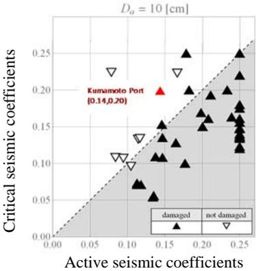
Figure 13. Comparison of Active and Critical Seismic Intensities <sup>added to Fukunaga et al. 2016</sup>, Gravity Quay Walls with water depth from -7.5m to -14.6m (Comparison of the Results of Verification of Damage in This Study and Other Facilities)
