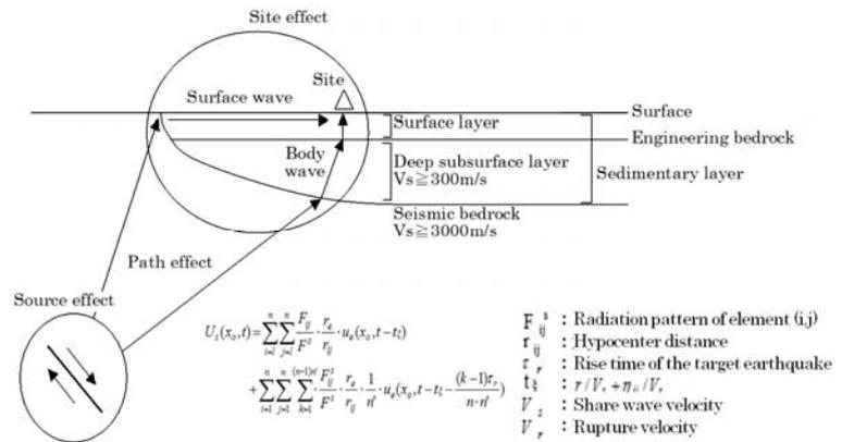
Figure 2. Conceptual Diagram of the C-EGF Method
