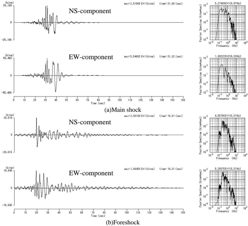
Figure 6. Estimation of Strong Ground Motions at Kumamoto Port (left: Velocity waveforms, right: Fourier spectra)
