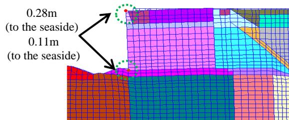
Figure 14. Part of Displacement Diagram of the -7.5m Quay Wall at Kumamoto Port
