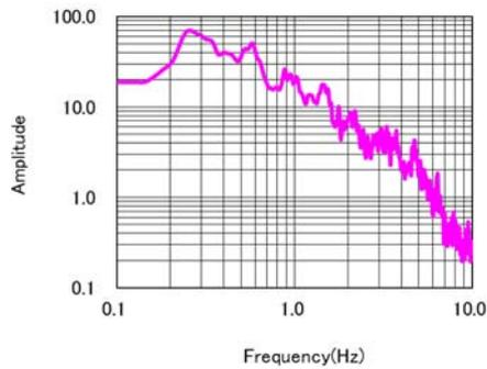
Figure 1. Site Amplification Factor of Kumamoto Port (Seismic Bedrock to Engineering Bedrock)
