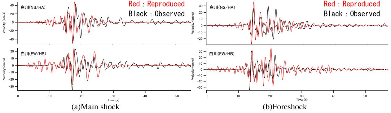
Figure 4. Reproduced and Observed Velocity Waveforms at Shirakawa (Oshima) Observatory
