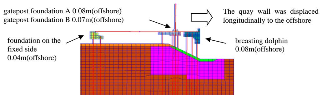
Figure 15. Part of Displacement Diagram of the -5.0m Quay Wall at Kumamoto Port
