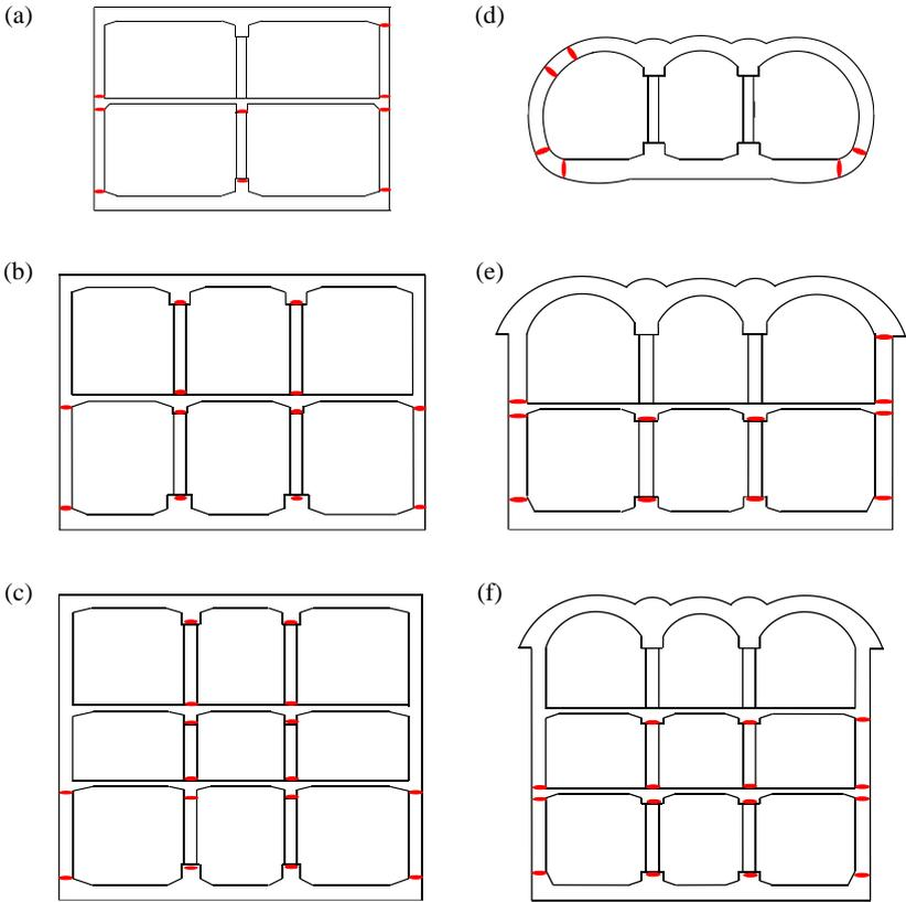
Figure 1. Typical underground structures and the plastic hinges developed in pushover analysis
