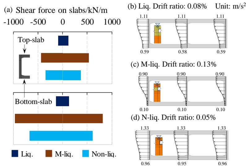
Figure 4. Shear forces and acceleration on the structure in three different soil profiles
