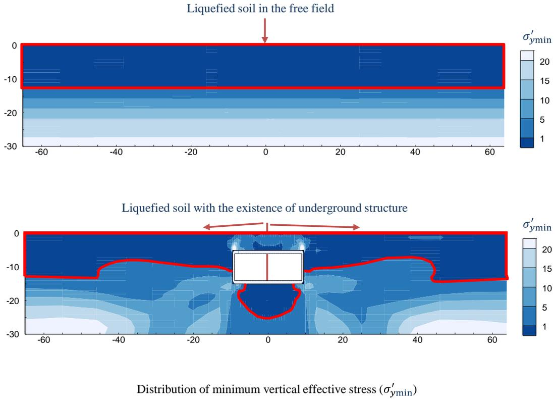
Figure 5. Distribution of minimum effective stress during shaking without and with underground structure
