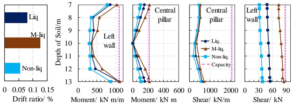
Figure 3. Drift ratio and bending moment of the structure in three different soil profiles
