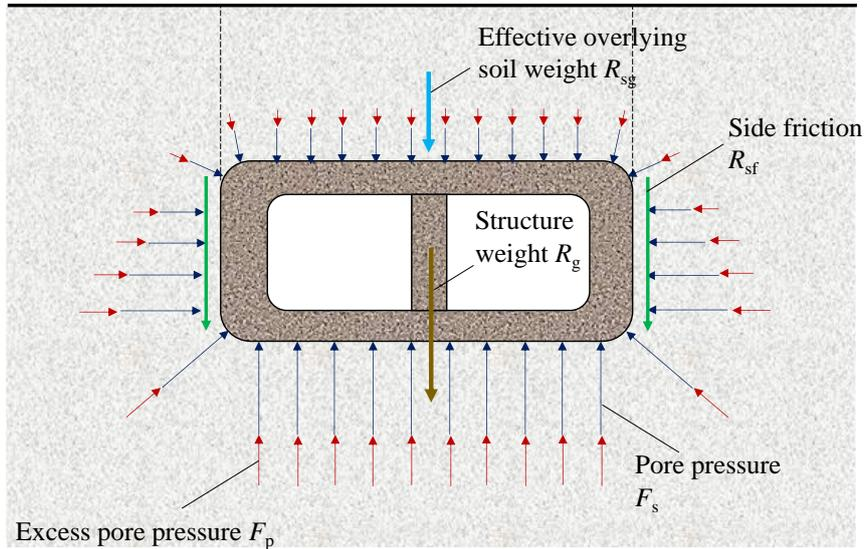
Figure 6. Diagram of uplifting forces and downward forces acting upon underground structures
