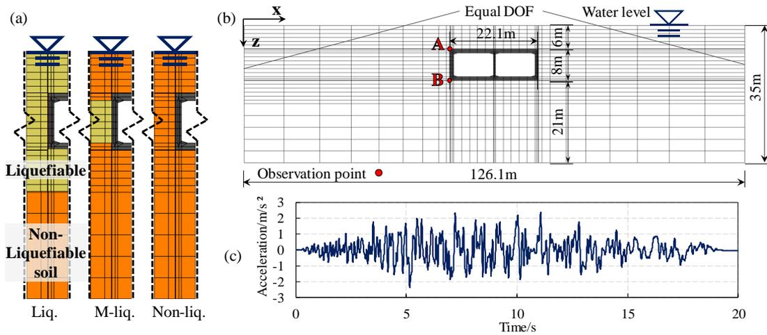
Figure 2. Soil profile, FEM mesh, and input ground motion
