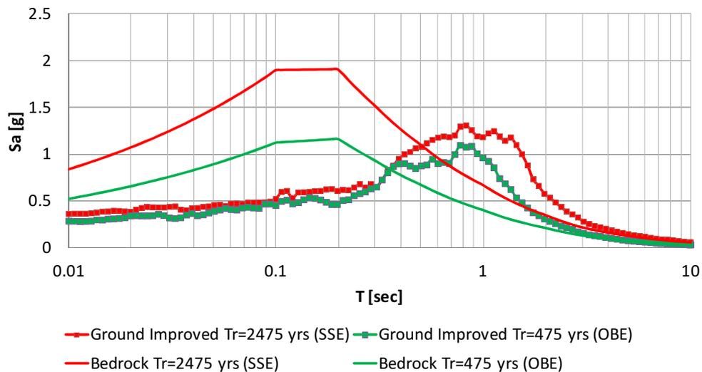
Figure 2. Horizontal response spectra at 5% damping
