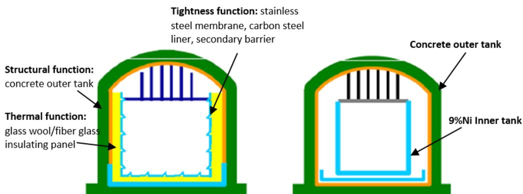
Figure 1. Conceptual simplified representation of membrane tank (left) and full containment tank (right).
