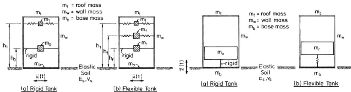
Figure 3. Spring-mass analogy for horizontal motion (left) and vertical motion (right) – after Priestley et al. 1986
