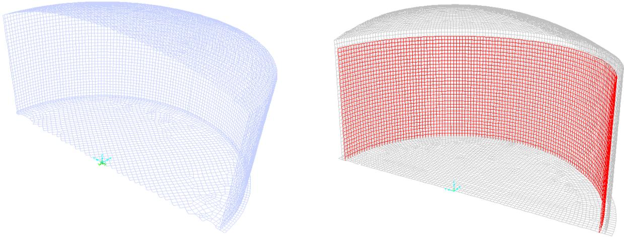
Figure 4. Finite element model: membrane tank (left) and full containment tank (right). In grey are shown the concrete elements and in red the steel elements
