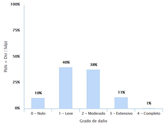
Figure 9. Example of expected damage results for a return period of 975 years.
