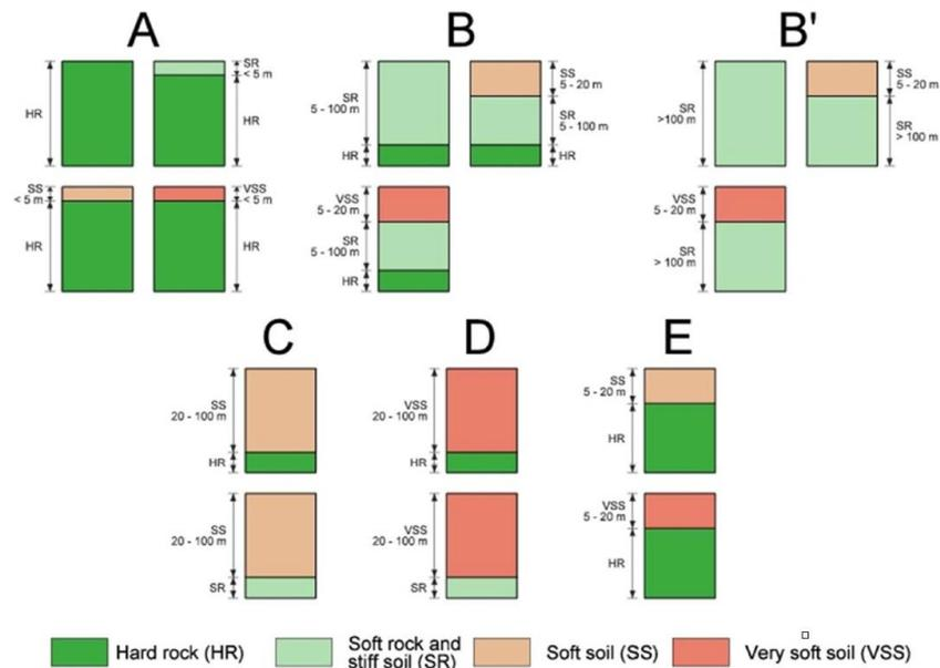
Figure 4. Soil classes identified in the seismic mesozonation study of Catalonia.
