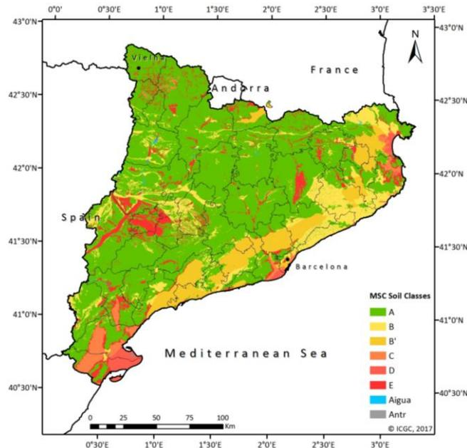
Figure 3. Seismic mesozonation map of Catalonia (MSC), scale 1:100M
