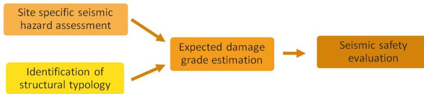
Figure 1. Summary of the seismic safety evaluation.
