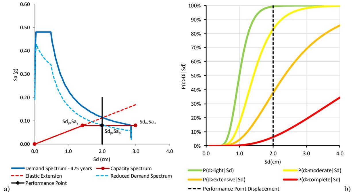
Figure 6. a) Determination of the performance point using the capacity spectrum method and b) Example of the fragility curves used to obtain the damage probability distribution.
