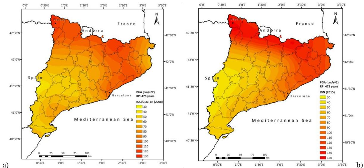
Figure 2. Comparison between the PGA maps for a return period of 475 years from both (a) the IGC and GEOTER (2008) PSHA study and (b) the new PSHA evaluation for Spain from IGN (2015).
