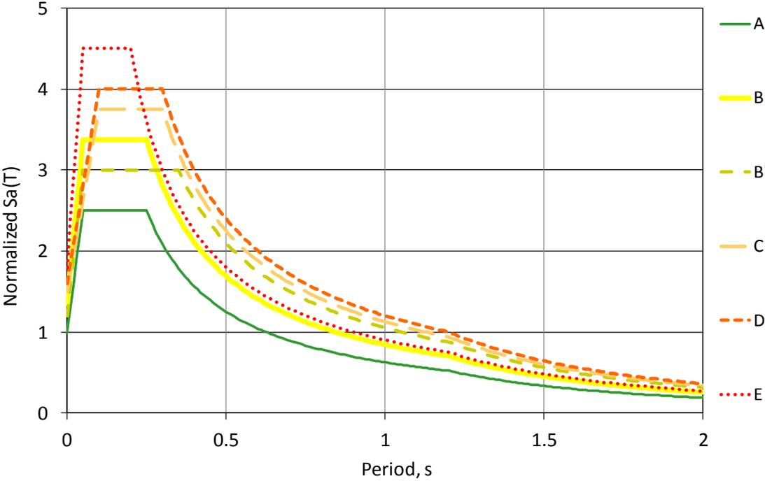
Figure 5. Normalized acceleration response spectra for each mesozonation soil class (Colas et al., 2012).
