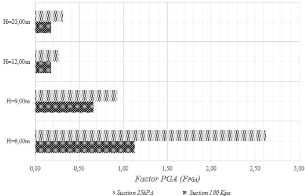
Figure 7.  $F_{PGA}$  values for each of the thicknesses modeled in the given matrix suction conditions
