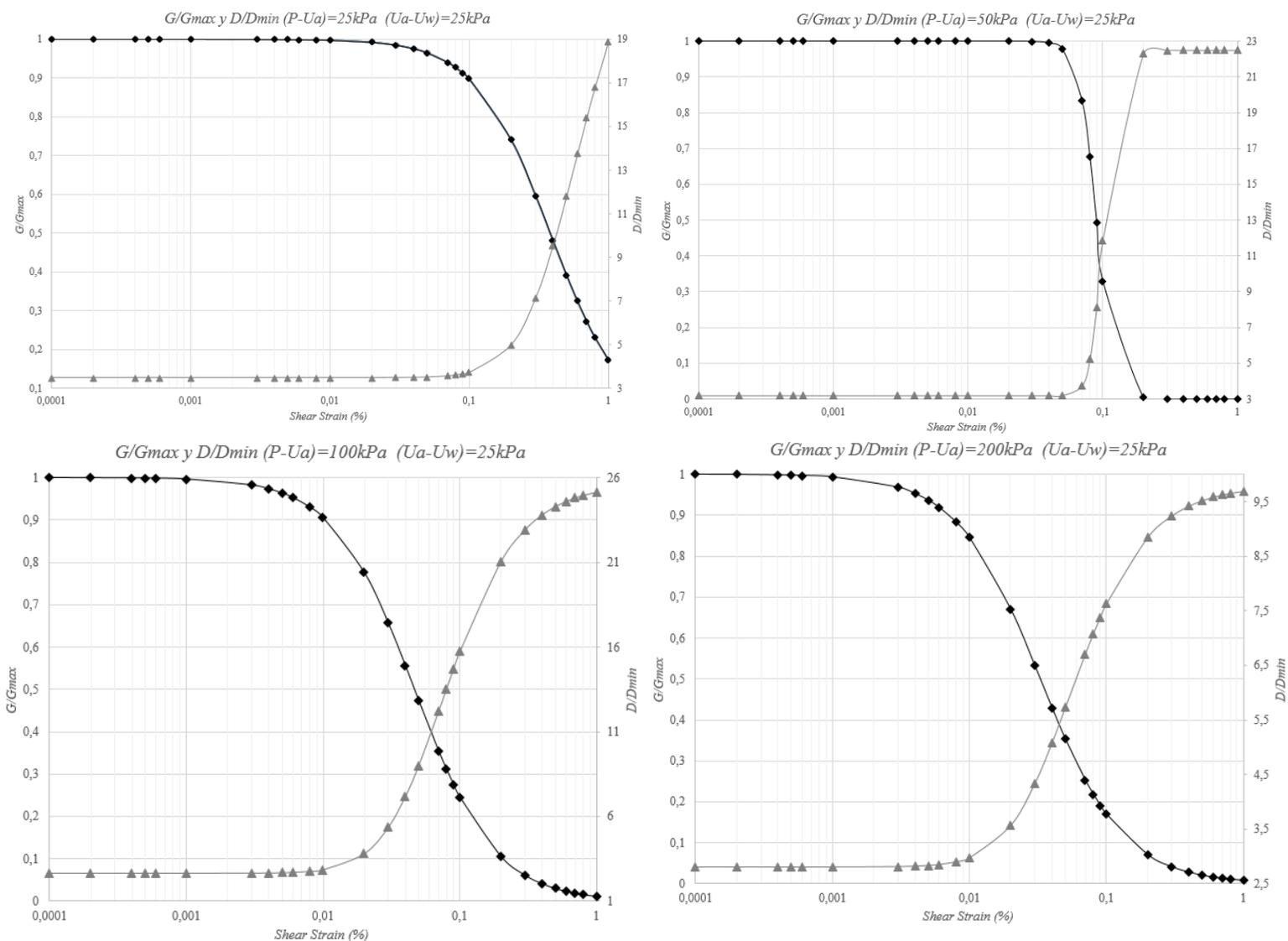
Figure 1. Graphics of  $G/G_{max}$  y  $D/D_{min}$  obtained by the empirical equations raised by (PINO 2013)
