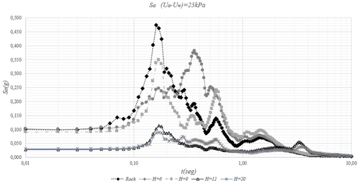
Figure 4. Acceleration spectrum obtained for a soil profile submitted to a constant matrix suction of 25kPa.
