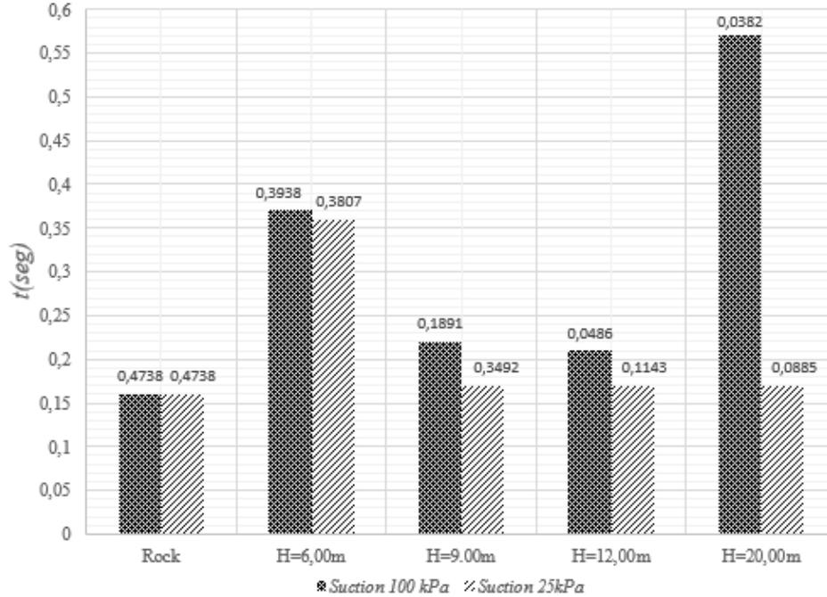
Figure 6. Instant of time in which the spectral peak acceleration is generated for each of the analyzed thickness and suctions matrix established.
