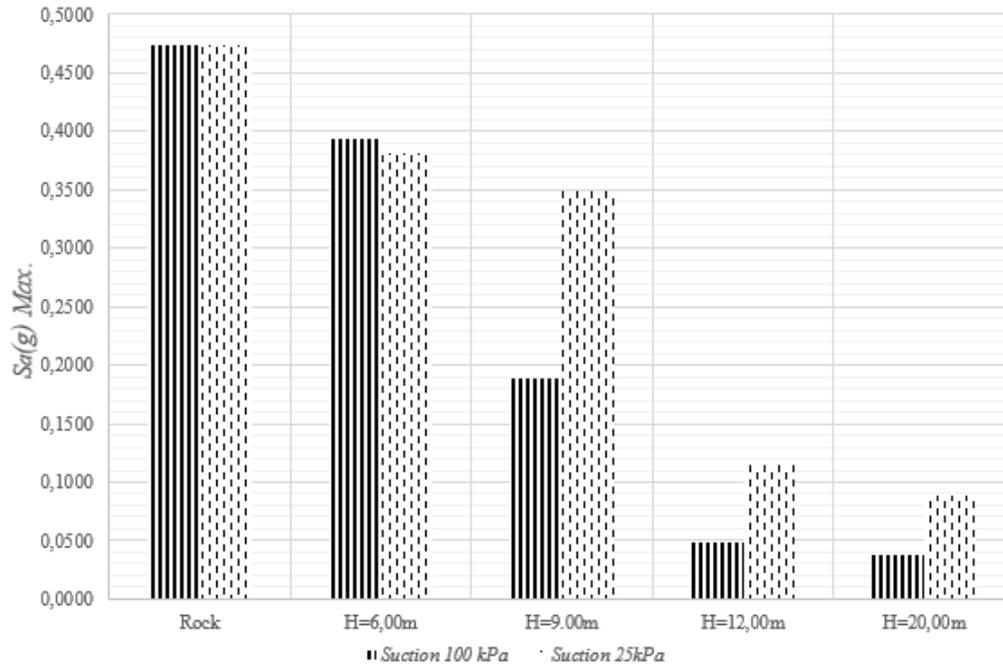
Figure 5. Variation in the dissipation of energy in each of the thicknesses in relation to the change in the matrix suction of the material.
