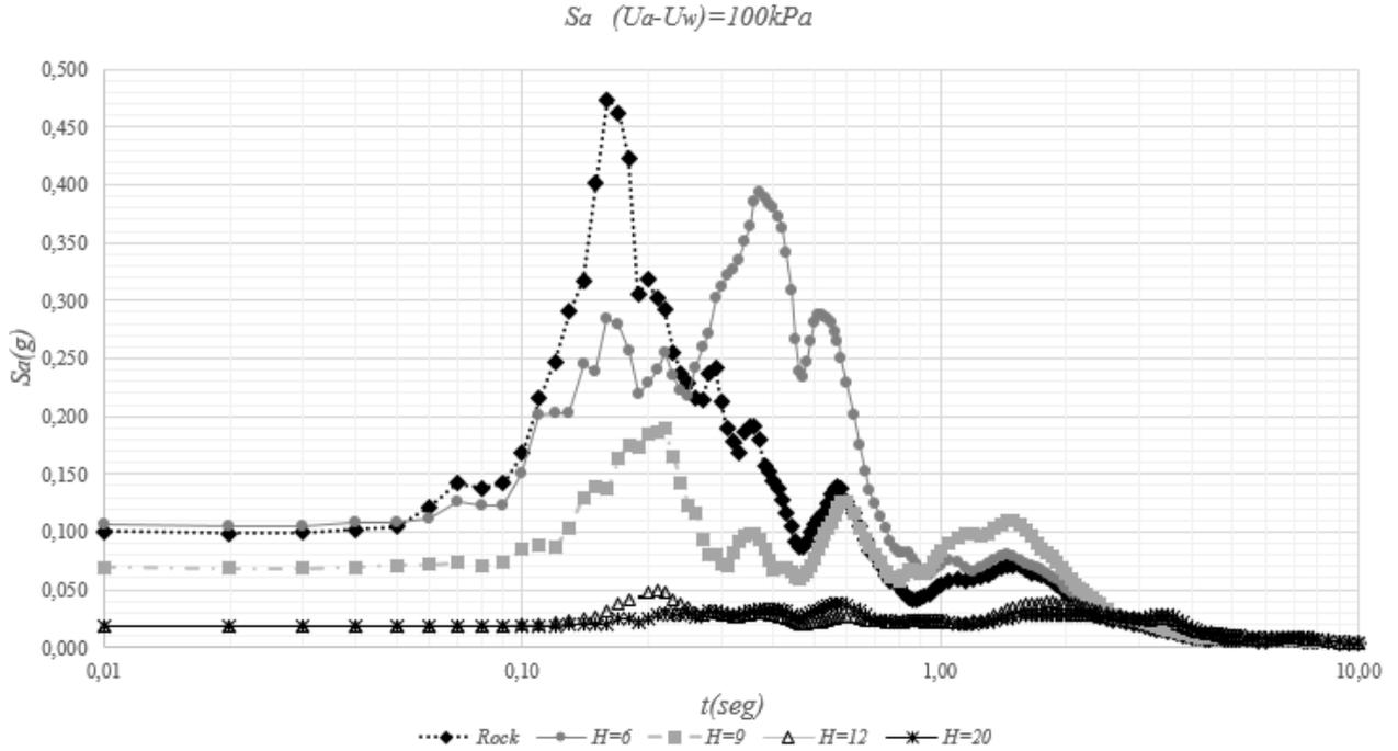
Figure 3. Acceleration spectrum obtained for a soil profile submitted to a constant matrix suction of 100kPa.
