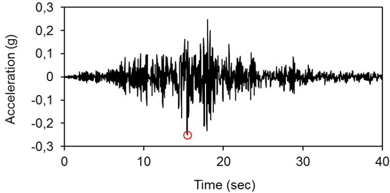
Figure 2. Accelerogram corresponding to earthquake KYUSHO-JAPON.
