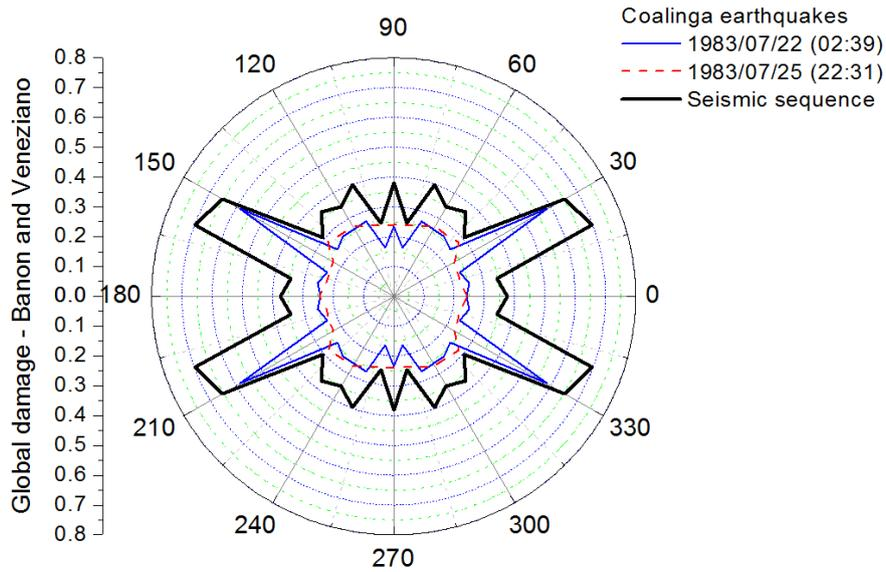
Figure 6. Banon-Veneziano (1982) damage index for various incident angles
