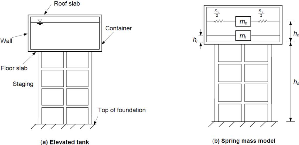
Figure 2: Simulation of elevated water concrete tank (adopted from Jaiswal et al., 2004)
