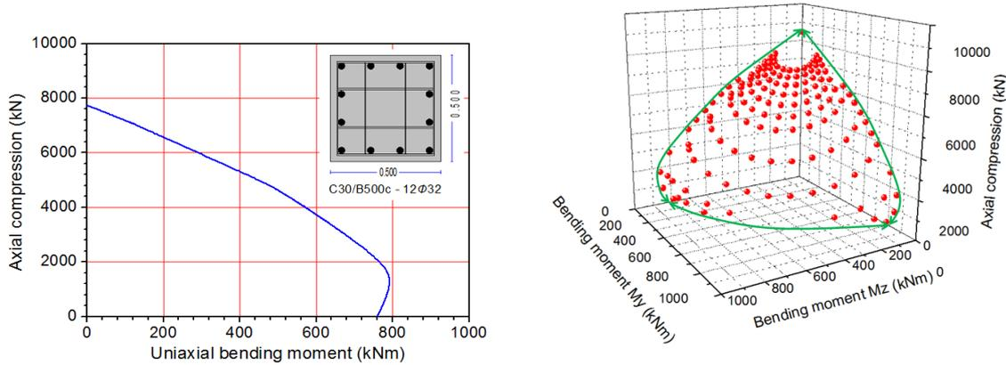
Figure 3: Bending moment - axial force interaction diagrams for columns
