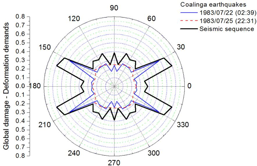
Figure 7. Cosenza et al. (1993) damage index for various incident angles
