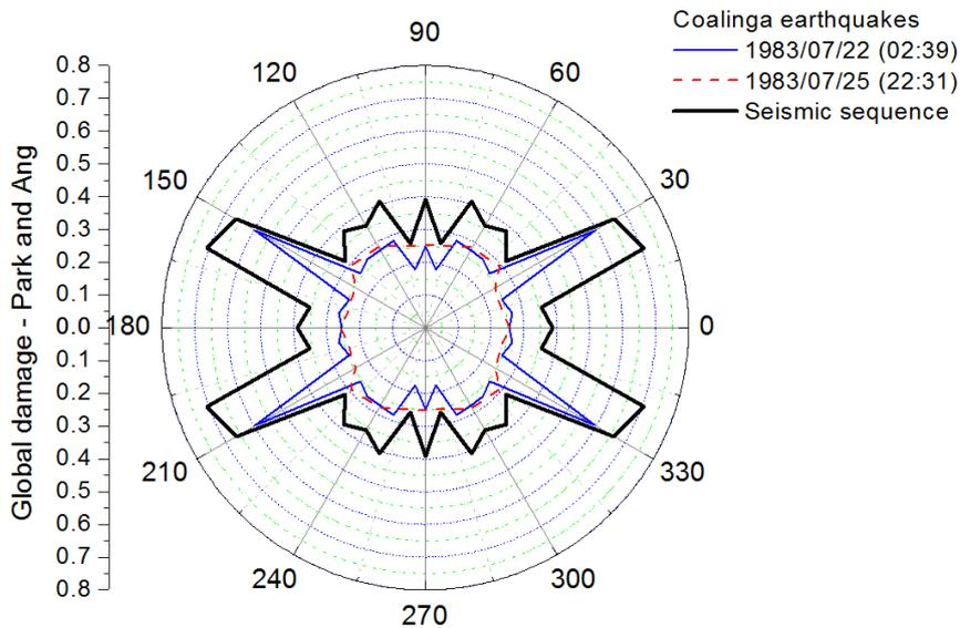
Figure 5. Park-Ang (1985) damage index for various incident angles
