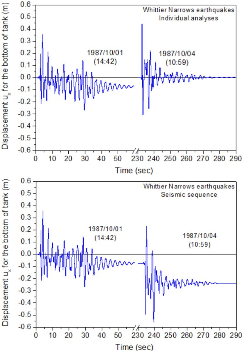
Figure 4. Horizontal displacement of the bottom of tank - Whittier Narrows earthquakes (1987)
