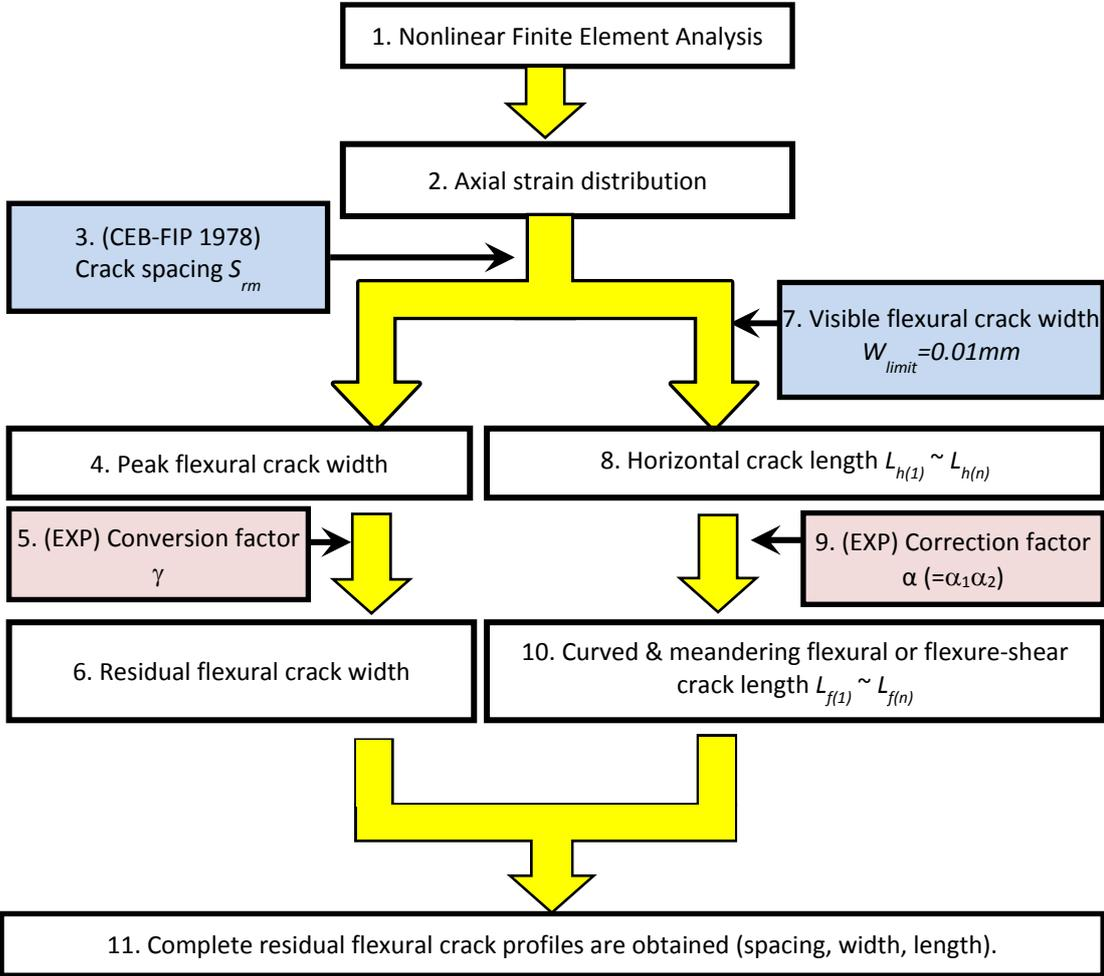
Figure 3. Flow chart how to obtain complete residual flexural crack profiles
