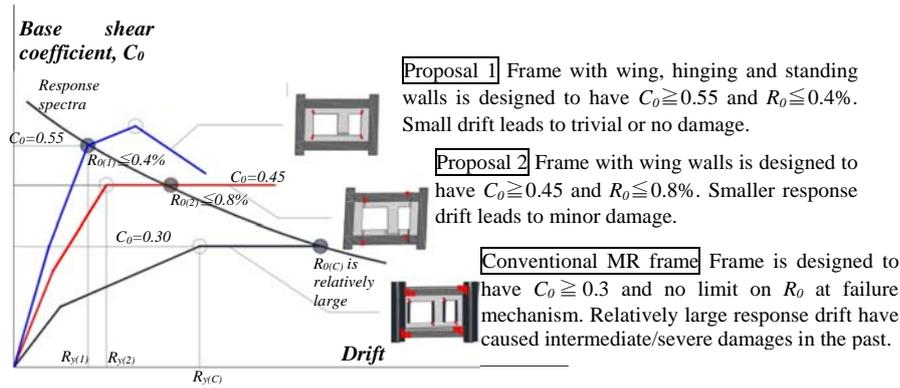
Figure 9. Design philosophy of reinforced concrete buildings for less damage (Fukuyama et al. 2015)
