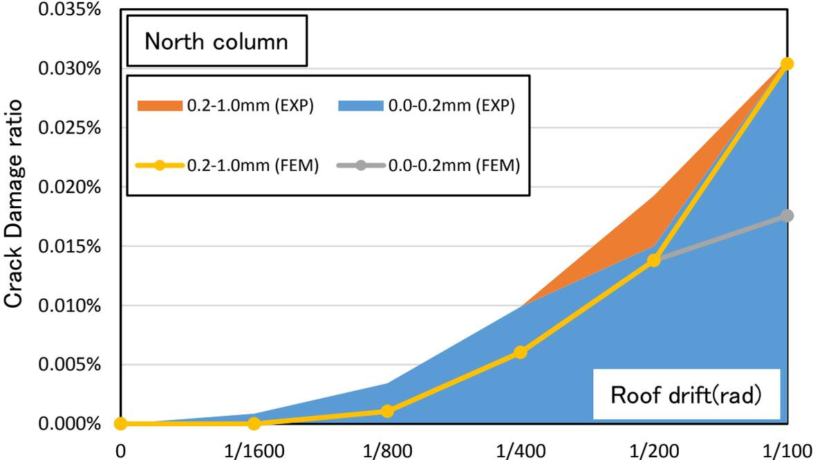
Figure 8. Comparison of experimental and computational variations of crack area damage ratio (North column)
