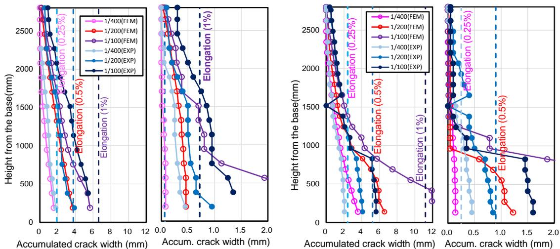
(a) North column (peak) (b) North column (residual) (c) North Wing wall (peak) (d) North Wing wall (residual)
