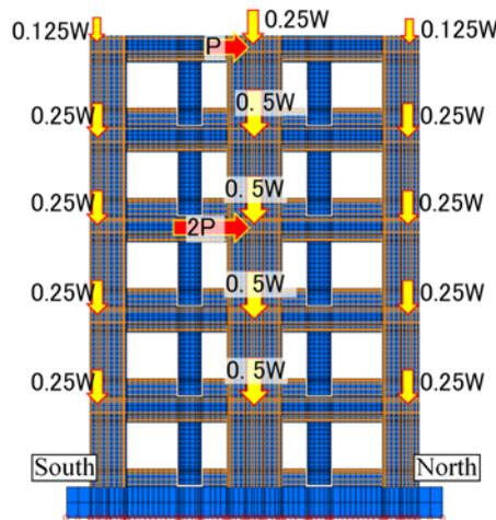
Figure 4. Finite element mesh and loading condition in 2D finite element analysis (Kitamura 2017)
