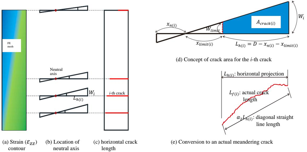
Figure 7. Calculation of crack length
