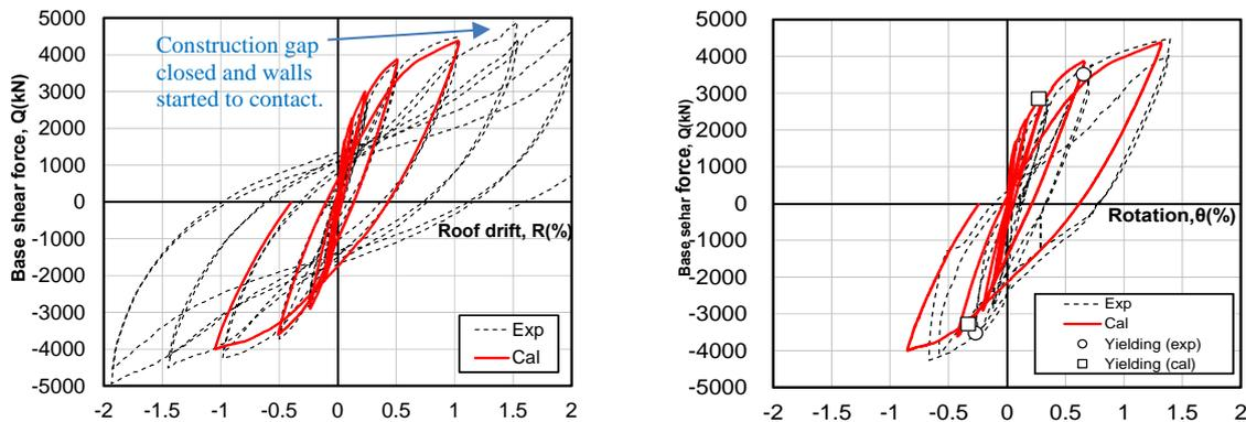
(a) Base shear force – roof level drift ratio relation
