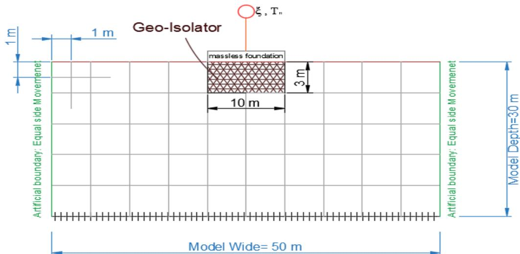
Figure 3. Schematic Modeling of Geo-Isolator FE Modeling
