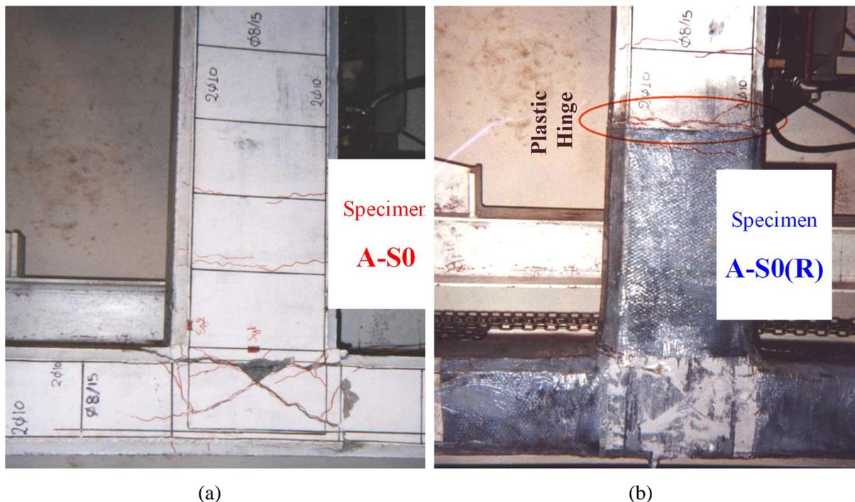
Figure 4. Damage modes and crack patterns of the tested beam-column joint specimens of group A: (a) Original specimen A-S0, (b) Rehabilitated specimen A-S0(R)
