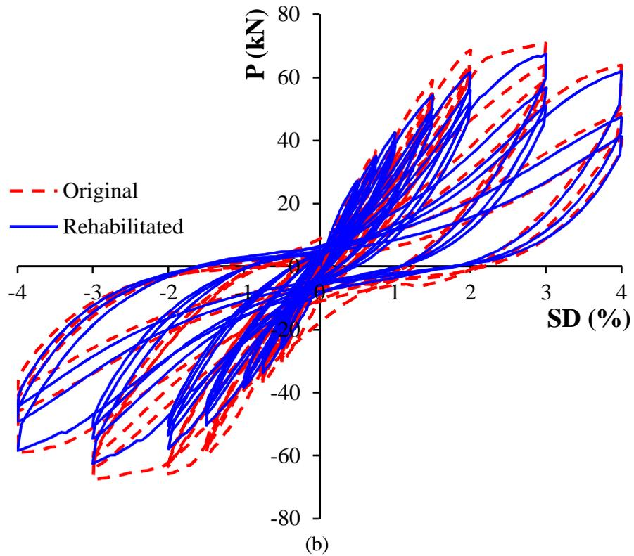
Figure 3. Hysteretic response diagrams of the tested specimens: (a) beam-column joint specimens of group A, (b) beam-column joint specimens of group B
