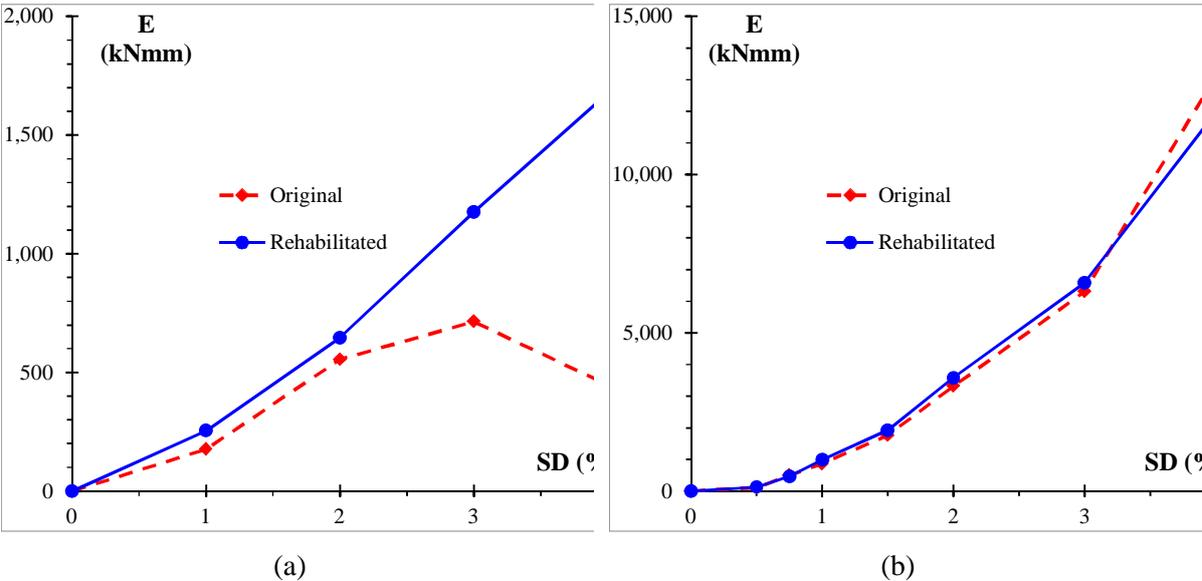
Figure 7. Energy absorption of the tested specimens: (a) Beam-column joint specimens of group A, (b) Beam-column joint specimens of group B
