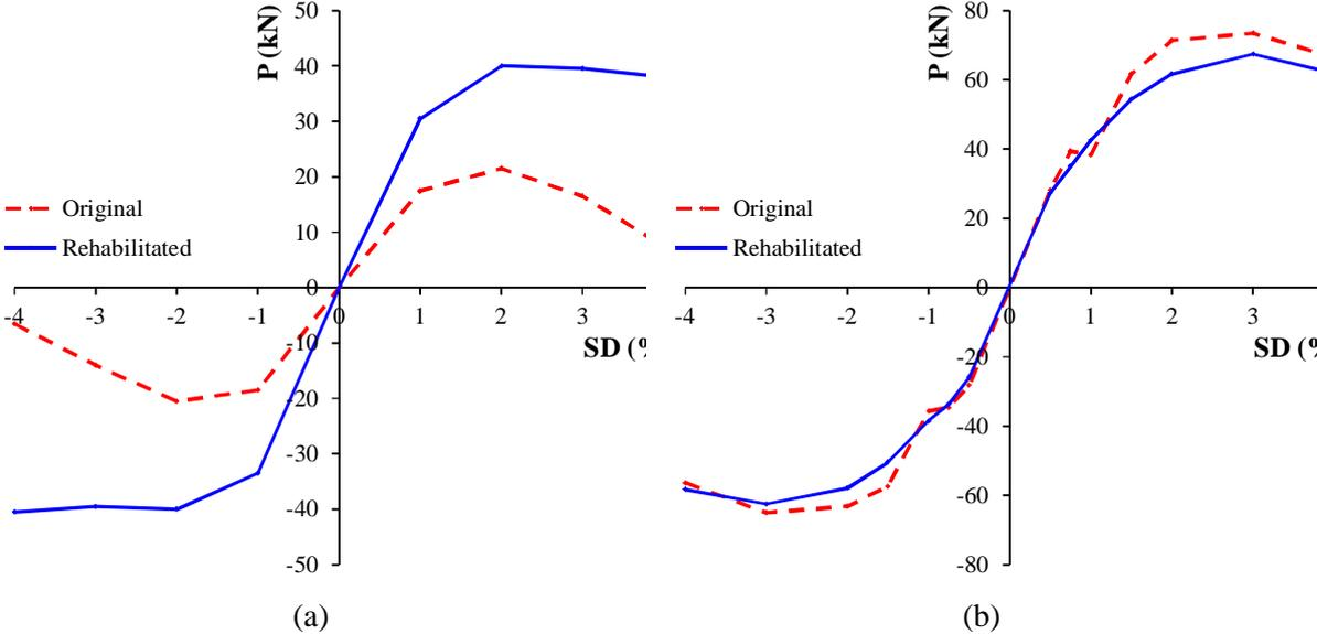
Figure 6. Envelope curves of observed maximum loads of the hysteretic response of the tested specimens: (a) Beam-column joint specimens of group A, (b) Beam-column joint specimens of group B
