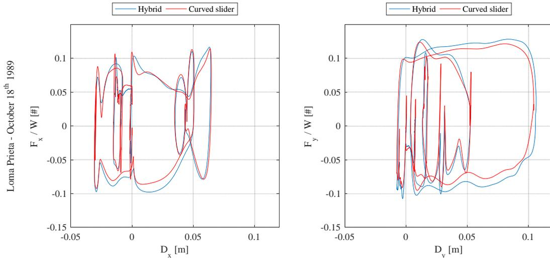
Figure 7. DCSS-D260 ( $W = 1751$  kN): Hybrid vs. Experimental earthquake simulation
