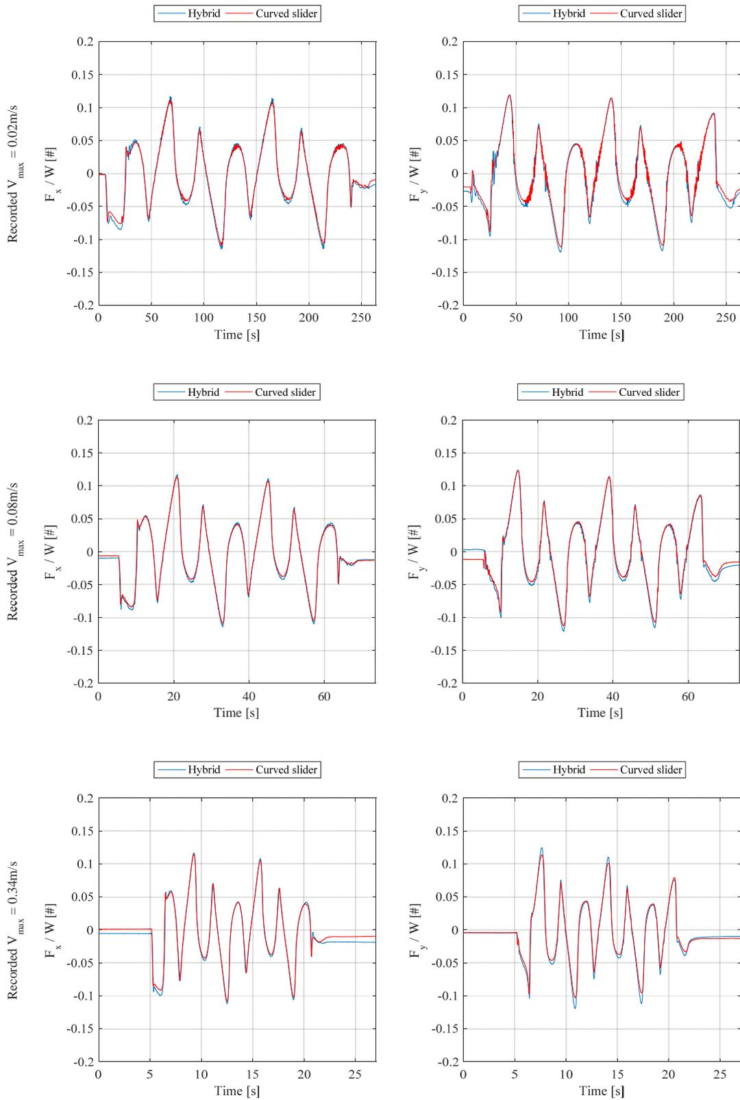
Figure 5. DCSS-D260 ( $W = 2388 \text{ kN}$ ): Hybrid vs. Experimental CTV orbits response
