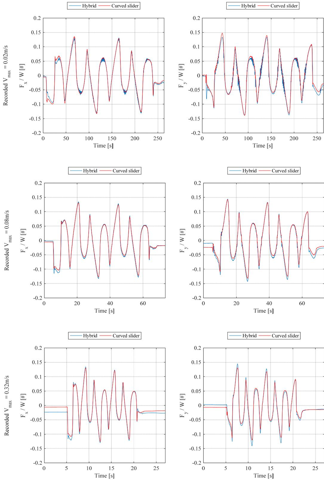
Figure 4. DCSS-D260 ( $W = 1751 \text{ kN}$ ): Hybrid vs. Experimental CTV orbits response
