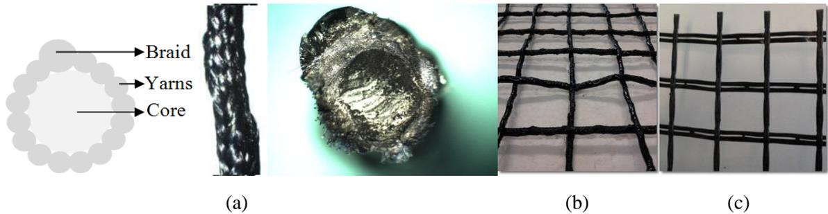
Figure 3 Details of braided rods and meshes; (a) cross section of a braided mesh [20]; (b) designed mesh; (c) commercial mesh
