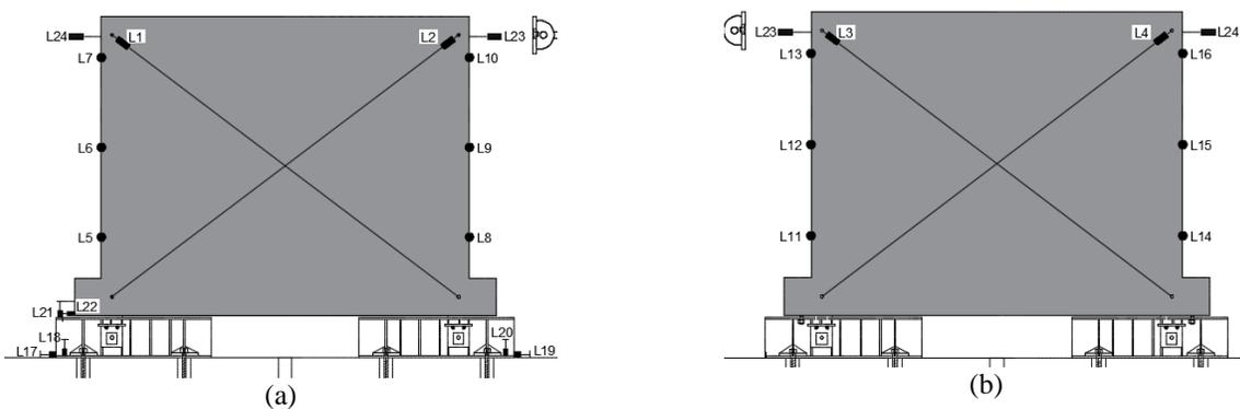
Figure 8 Instrumentation of the specimen for in-plane loading; (a) external leaf (b) internal leaf
