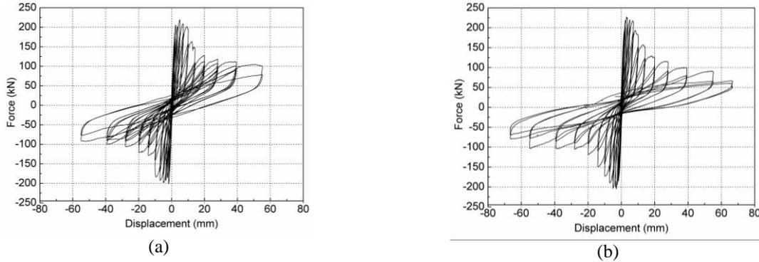
Figure 11 Force-displacement diagram (a) specimen SIF(CTRM)-I-B; (b) specimen SIF(DTRM)-I-B
