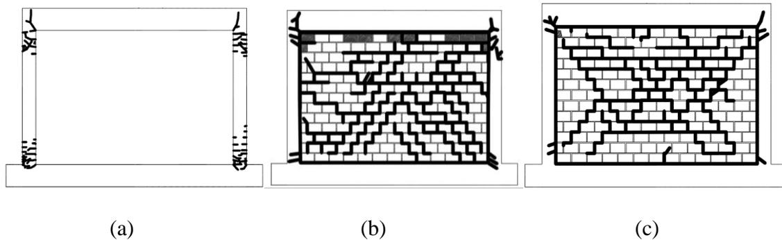
Figure 12 Final cracking pattern of the bare frame; (b) specimen SIF-I-A at end of the test; (c) specimen at lateral drift of 1%;
