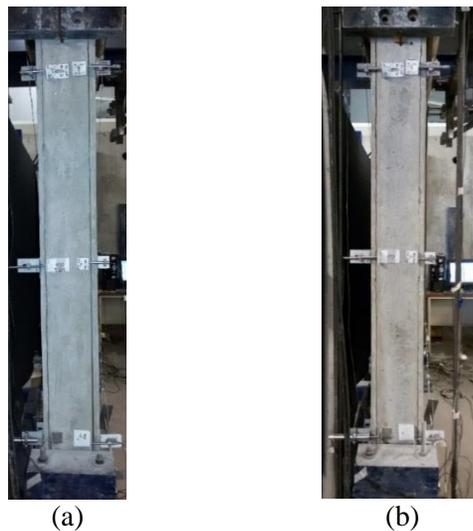
Figure 14 Detachment of the reinforced mortar layer from the rc frame (a) specimen strengthened with commercial mesh at lateral drift of 0.27% b) (a) specimen strengthened with developed mesh at lateral drift of 0.20%
