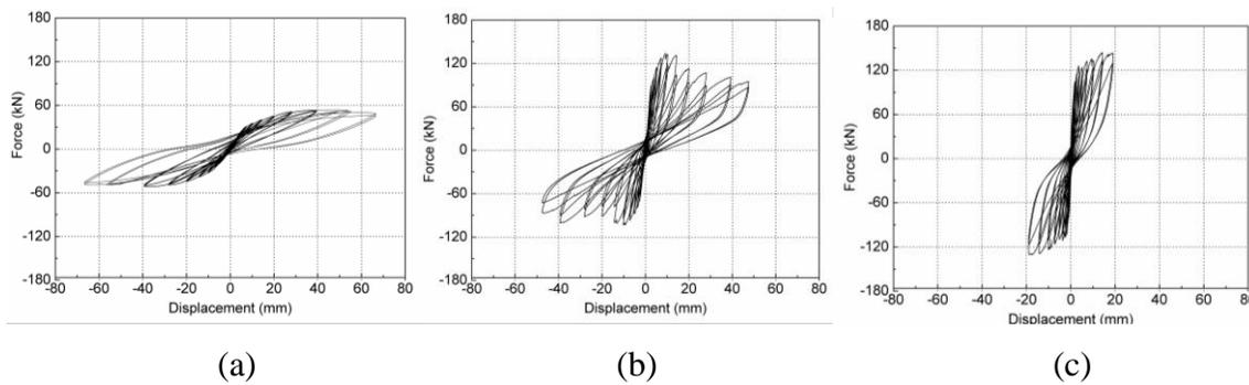
Figure 10 Force-displacement diagram; (a) bare frame; (b) specimen SIF-I-A; (c) specimen SIF-I(1%)-B
