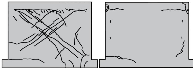
Figure 13 Cracking pattern in the rendering mortar at the end of the test; (a) specimen SIF(CTRM)-I-B; (b) specimen SIF(DTRM)-I-B
