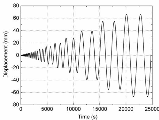
Figure 9 Displacement protocol for in-plane testing
