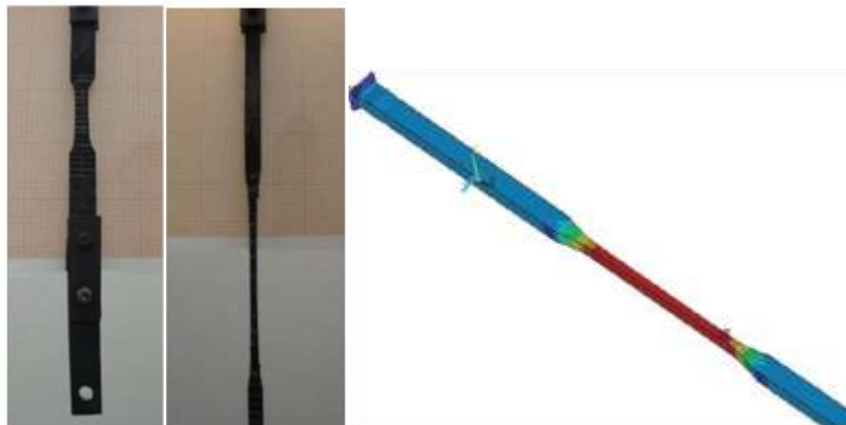
Figure 3. Test specimen before and after in experimental test and with ANSYS simulation
