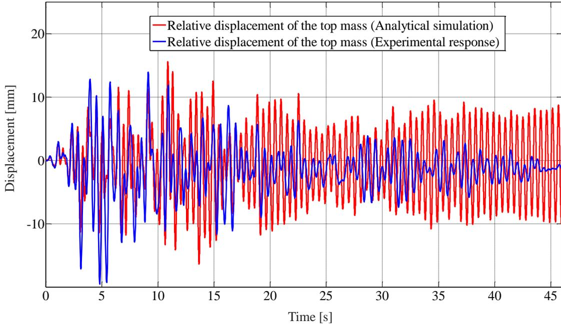
Fig. 11. Response of the specimen with 4 mm, 480 MPa coupons to the 75% 1994 Northridge ground motion excitation: displacement time history responses of the isolated superstructure (analytical simulation and experimental response)
