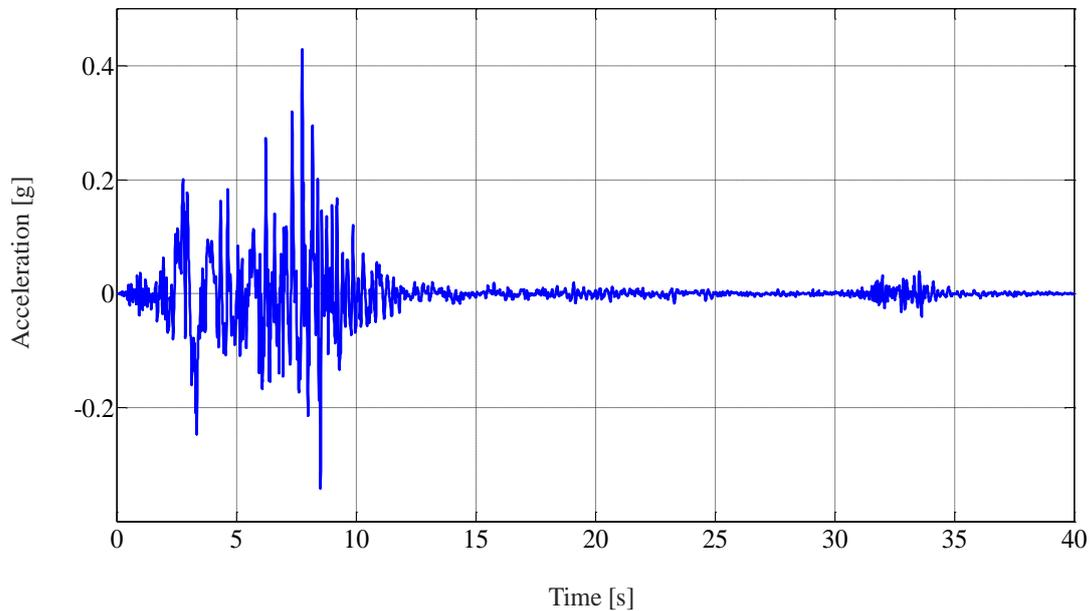
Fig. 7. 35%-scaled 1971 San Fernando ground motion excitation
