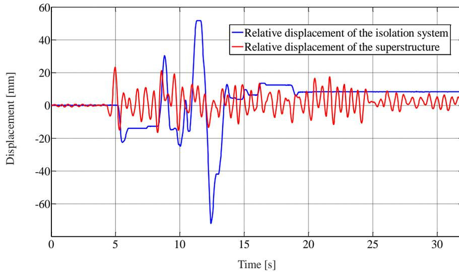
Fig. 5. Displacement time history response of the isolation system and the isolated superstructure to the 32.5% 1978 Tabas ground motion
