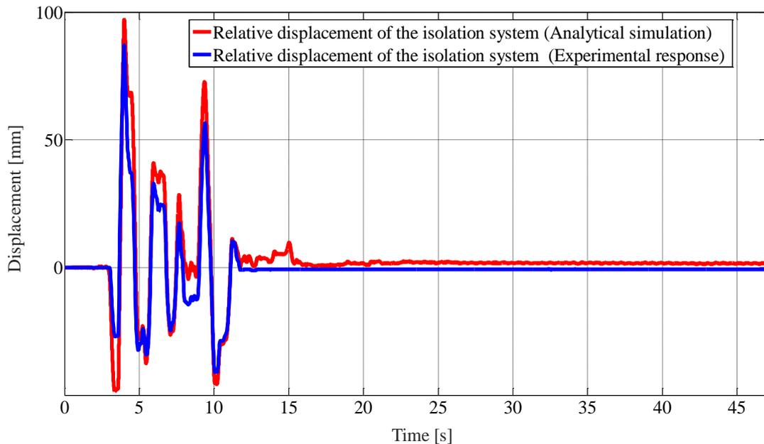
Fig. 10. Response of the specimen with 4 mm, 480 MPa coupons to the 75% 1994 Northridge ground motion excitation: displacement time history responses of the isolation system (analytical simulation and experimental response)
