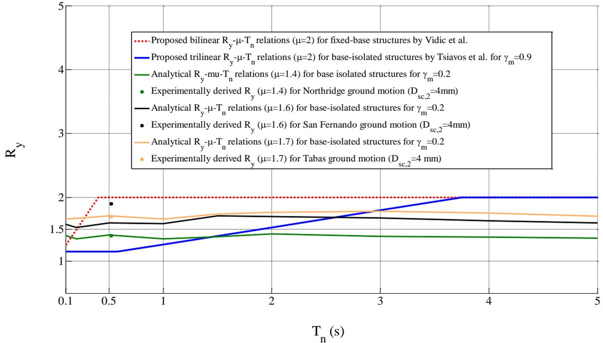
Fig. 12. Comparison of the analytically and experimentally derived  $R_y-\mu-T_n$  relations
