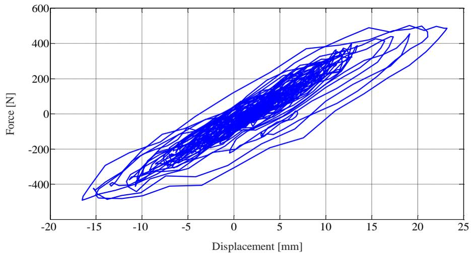
Fig. 6. Force-Displacement response of the isolated superstructure to the 32.5% 1978 Tabas ground motion
