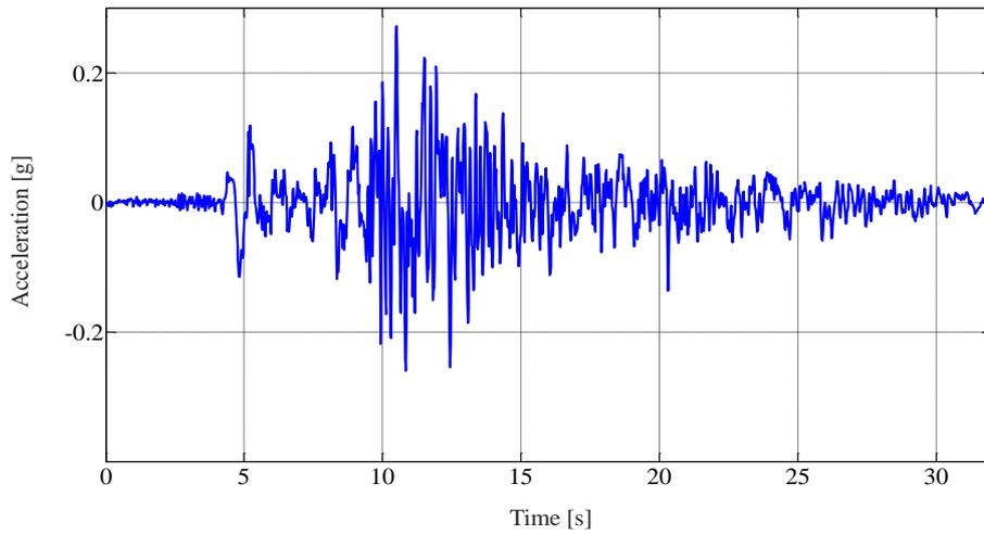
Fig. 4. 32.5%-scaled 1978 Tabas ground motion excitation
