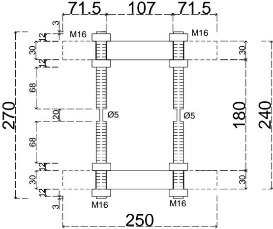
Figure 3. Elevation view of the 2 steel coupons (Dimensions in mm, Steel quality S275)
