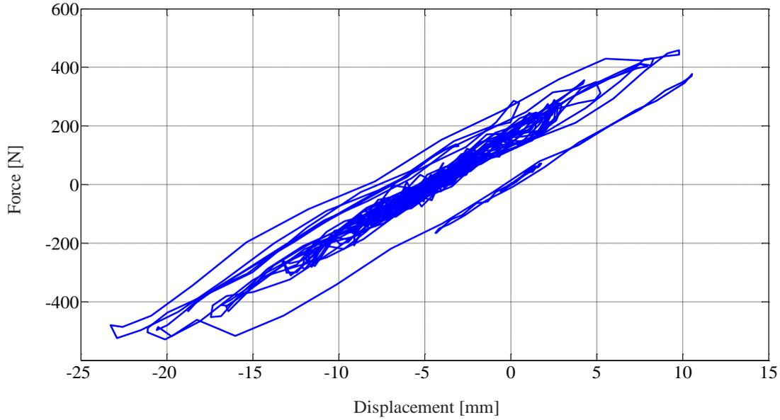
Fig. 9. Force-Displacement response of the superstructure to the 35% 1971 San Fernando ground motion
