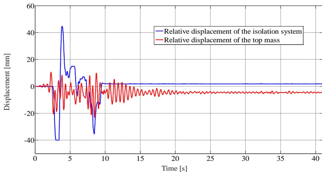
Fig. 8. Displacement time history response of the isolation system and the isolated superstructure to the 35% 1971 San Fernando ground motion
