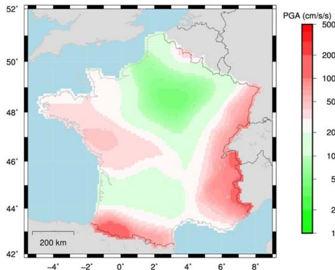
Figure 10. Hazard map for mean PGA at 475 years return period.
