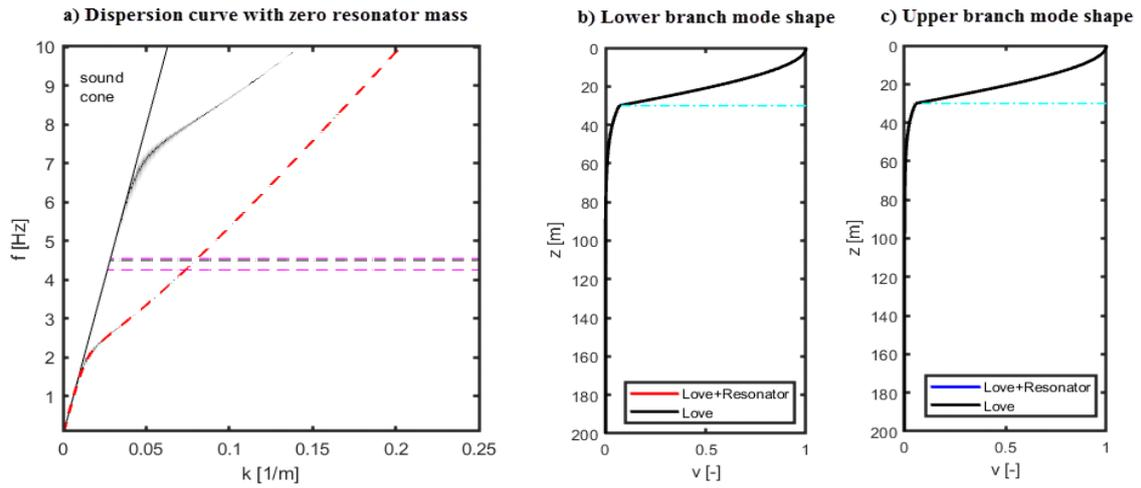
Figure 2. (a) Dispersion curve with zero mass (b) Mode shape of  $f=4.25$  Hz from lower branch (c) Mode shape of  $f=4.55$  Hz from upper branch
