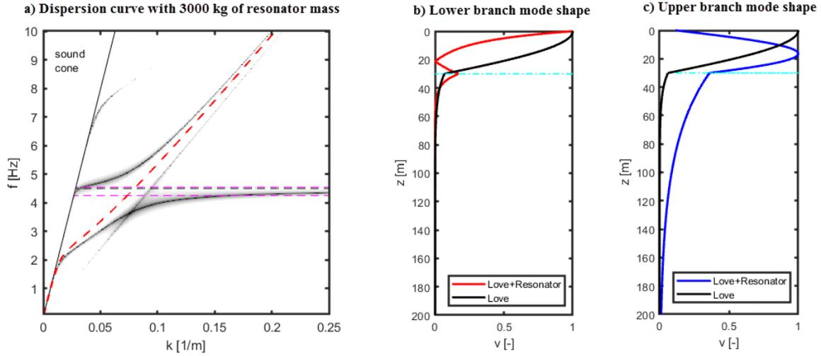
Figure 5. (a) Dispersion curve for resonator mass equals to 3000 kg (b) Mode shape of  $f=4.25$  Hz from lower branch (b) Mode shape of  $f=4.55$  Hz from upper branch
