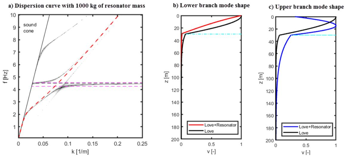
Figure 3. (a) Dispersion curve for resonator mass equals to 1000 kg (b) Mode shape of  $f=4.25$  Hz from lower branch (c) Mode shape of  $f=4.55$  Hz from upper branch
