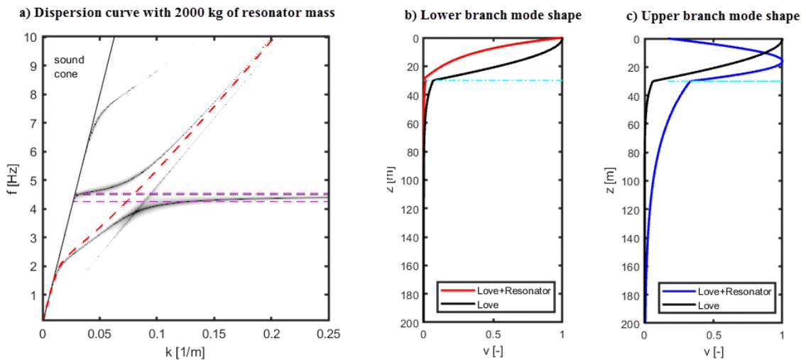
Figure 4. (a) Dispersion curve for resonator mass equals to 2000 kg (b) Mode shape of  $f=4.25$  Hz from lower branch (c) Mode shape of  $f=4.55$  Hz from upper branch
