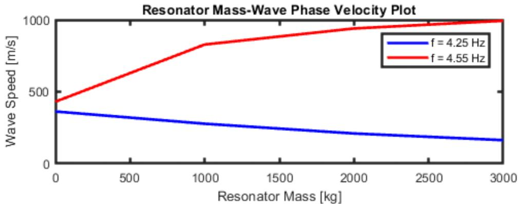
Figure 6. Effect of resonator mass on the Love wave phase speed
