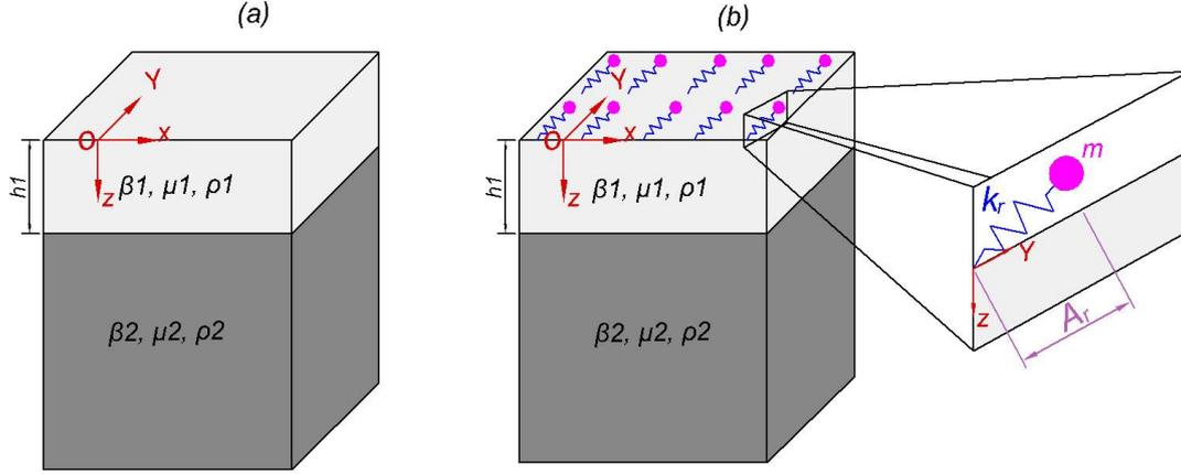
Figure 1. (a) Schematic of layer on half-space require for propagation of the Love wave; (b) interaction with a metabarriers
