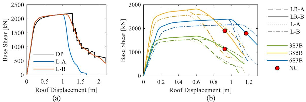
Figure 4. (a) Pushover curves for MRF 6S3B using distributed (DP) and lumped plasticity models (L-A, L-B) and (b) pushover curves with indication of NC point for LR-B models.
