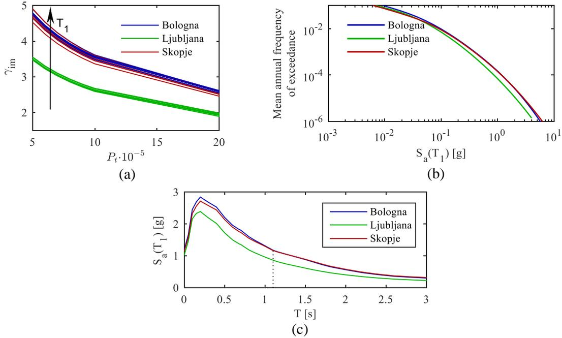
Figure 5. (a) risk-targeted safety factors  $\gamma_{im}$  for all three sites and for different values of target collapse risk, (b) the hazard curves ( $T_1=1.10s$ ) and (c) hazard uniform spectra for Bologna, Ljubljana and Skopje
