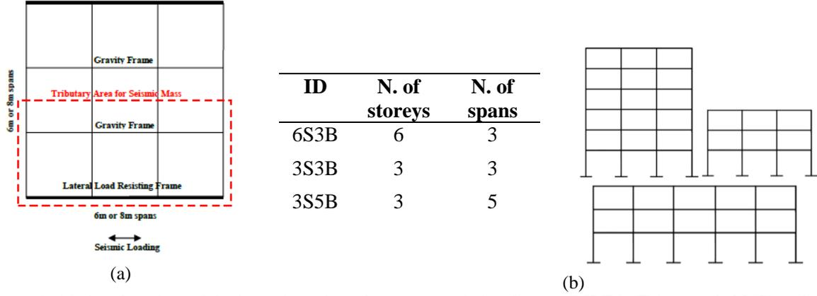
Figure 1. (a) the plan view of the investigated steel moment resisting frames (MRFs) (Tsitos et al. 2017) and (b) the corresponding elevation view for three different configurations of the geometry of MRFs.
