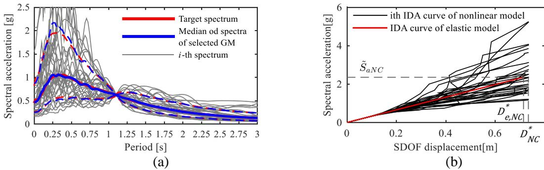
Figure 6. (a) acceleration spectra of the selected ground motions, the target spectrum for ground motion selection and the median value of the spectral accelerations of selected ground motions and (b) IDA curves using the nonlinear and elastic SDOF model
