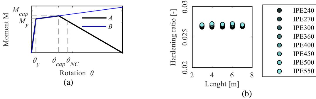
Figure 2. (a) Moment-rotation relationship for inelastic rotational hinges and (b) hardening ratios for different sections and lengths.
