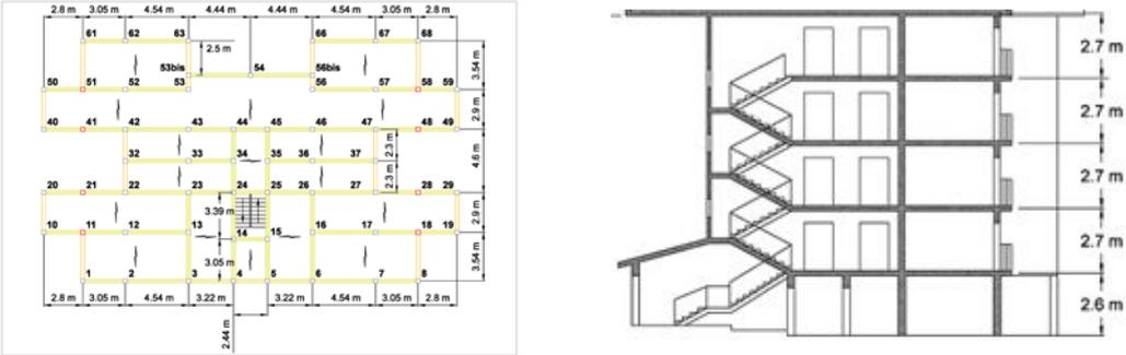
Figure 6. Surveyed building a) Floor plan with the frame distribution and double arrows indicating the orientation of unidirectional slabs b) Cross section of a module.
