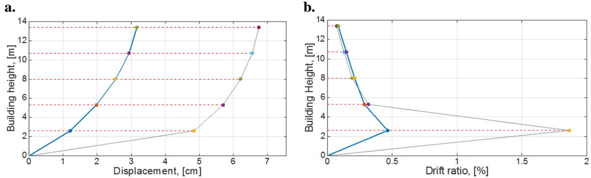
Figure 10. a) Lateral displacement and b) Inter storey drift ratio. Corresponding to two stages: Performance point stage (solid line) and Ultimate capacity stage (dashed line).
