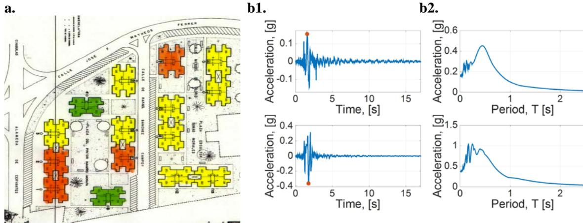
Figure 2. a) Damage distribution in the 15 buildings of San Fernando neighbourhood; b) the Lorca (Spain) 2011 earthquake: b1) Registered E30N and N30W accelerograms signals; b2) Response spectra.
