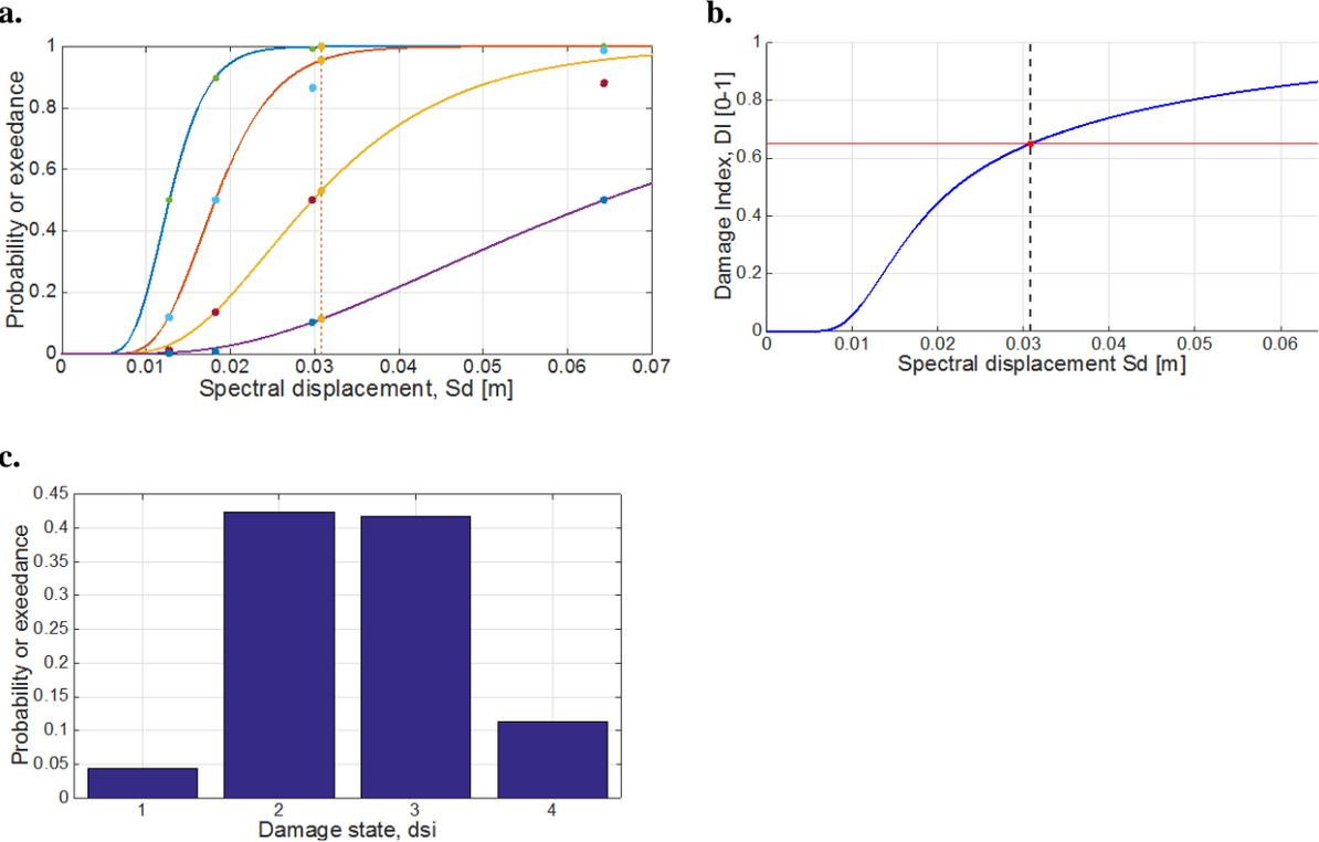
Figure 9. a) Fragility curves for the modelled building in the +Y direction; b) Damage index DI for the Lorca 2011 earthquake; c) Corresponding DPM for the performance point.
