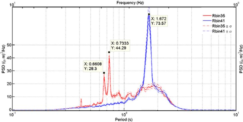
Figure 5. PSD calculated for bin 35 and 41. Two periods outstanding from the 35 bin: 0.661 s and 0.733 s while for bin 41 a higher single value is present: 1.67 s.
