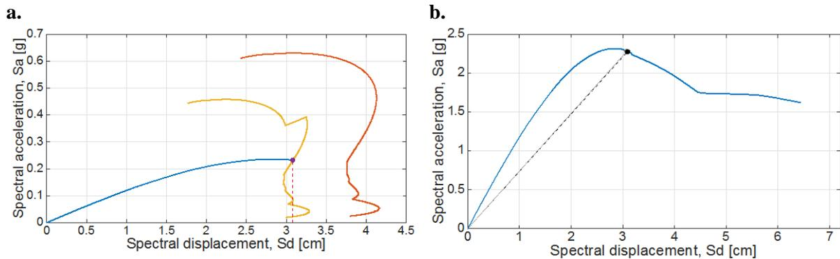
Figure 8. a) Evaluation of the performance point applying the iterative procedure A described in the ATC-40 (1996). b) Determination of the effective period corresponding to the performance point -solid line- and period of the experimental RAR measurement -dashed line-.
