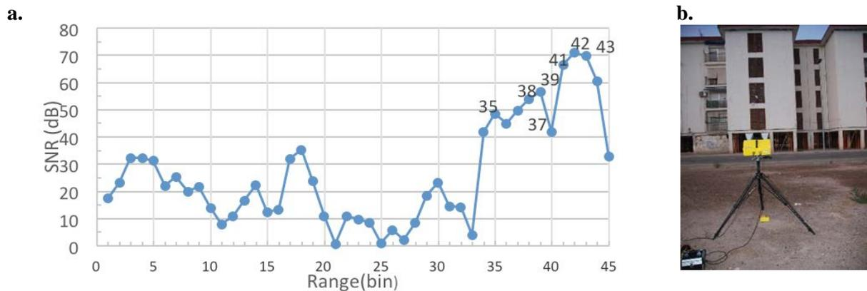
Figure 4. a) Range profile acquired in front of the building. The analysed radar bins are pointed out; b) The RAR equipment measuring the front façade of the building (Source: the authors).
