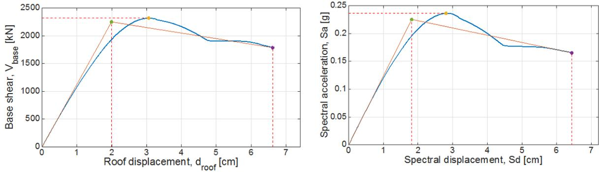
Figure 7. Capacity curve and capacity spectrum and their corresponding bilinear representations for the Y direction.
