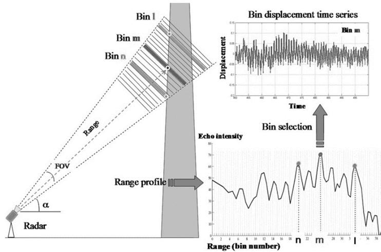
Figure 3. Scheme of the standard procedure aimed at retrieving displacement time series from the radar acquisition. The radar collects an amplitude profile as a function of the range, sampled at regular spatial steps, the radar bins. A displacement time signal is obtained from the interferometric phase of the echo of the selected bin.
