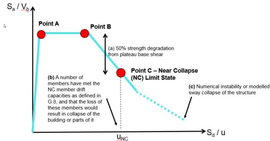
Figure 10. Global Near-Collapse (NC) limit state acceptance criteria (NZSEE, 2016).
