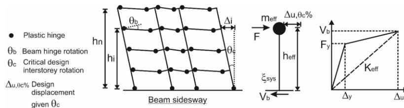
Figure 9. Conversion of MDOF system to an equivalent SDOF system (NZSEE, 2016).
