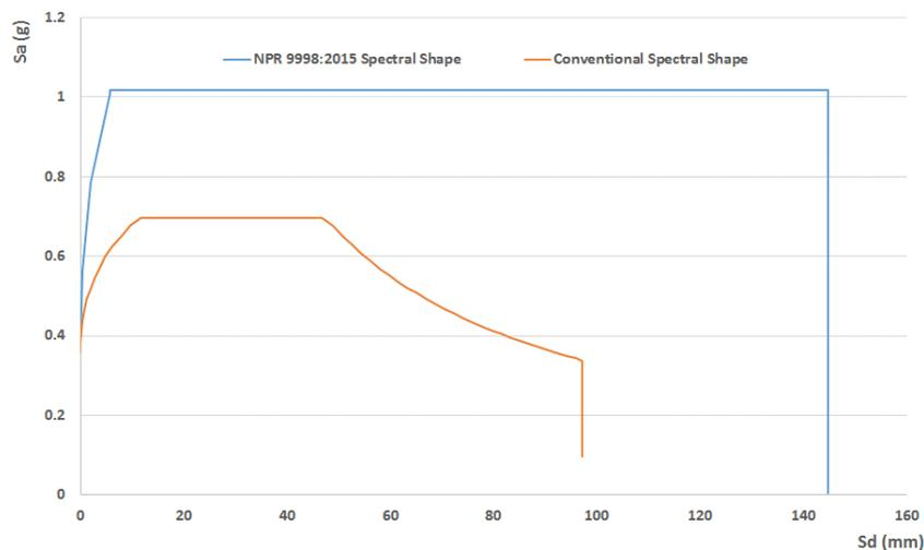
Figure 4. Comparison of NPR 9998:2015 and conventional spectral shapes.
