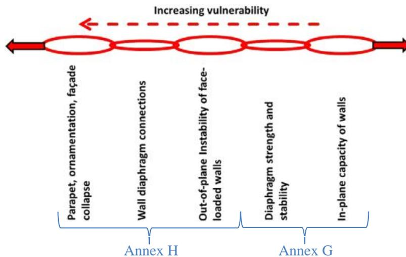
Figure 7. Hierarchy of URM building component vulnerability, demonstrated by way of the capacity ‘chain’ schematic (NZSEE, 2016).
