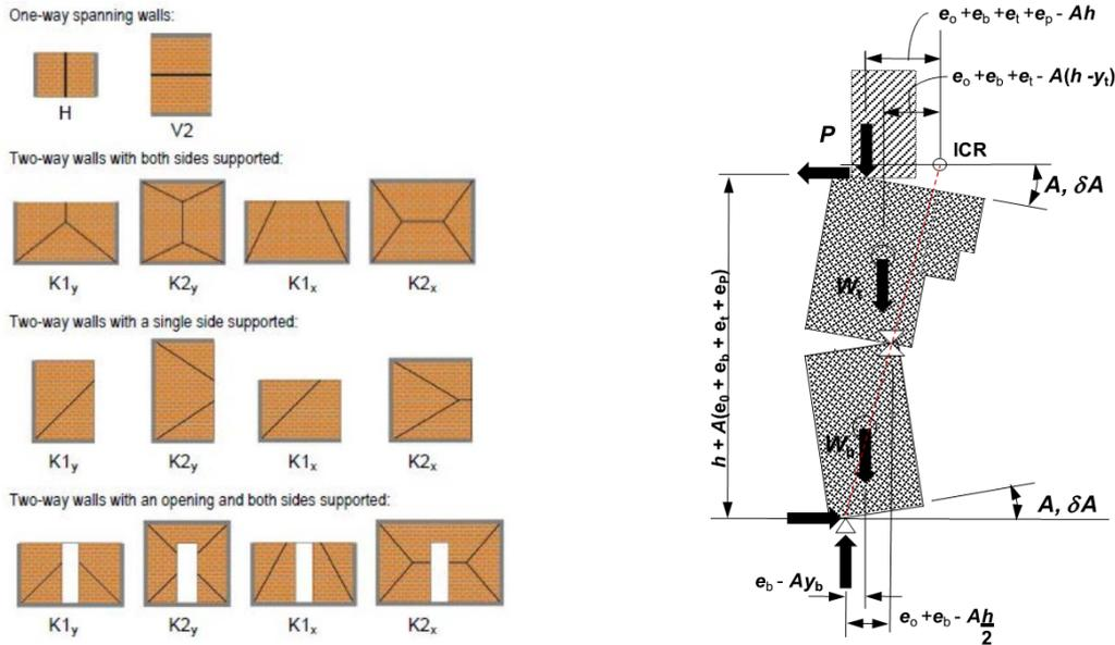
(a) Idealised cracking patterns for masonry walls. (b) One-way spanning wall out-of-plane mechanism.
