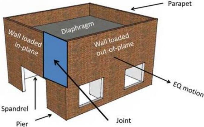
Figure 5. Building schematic displaying in-plane and out-of-plane loading.
