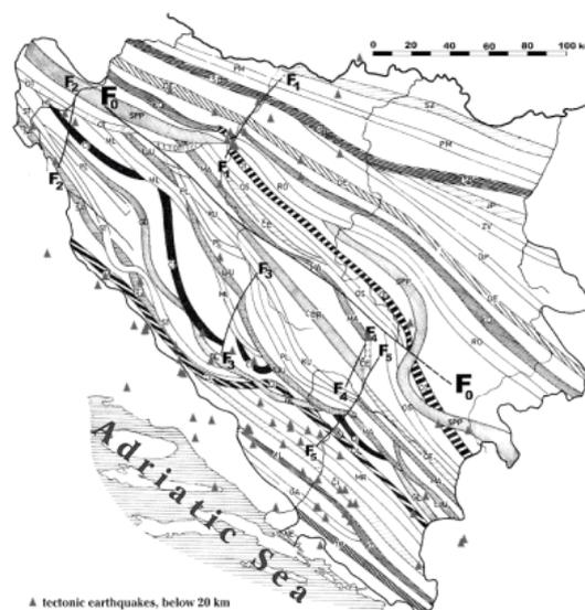
Figure 2. Main deep thrusts (to 25 km): Sarajevo fault (FoFo), Gradiška fault (F1F1), Bihać fault (F2F2), Livno fault (F3F3), Jablanica fault (F4F4) and Mostar fault (F5F5) (Papeš 1988)
