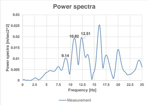
Figure 8. Measured frequencies
