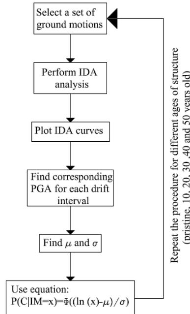
Figure 4. Fragility curve procedure in current study
