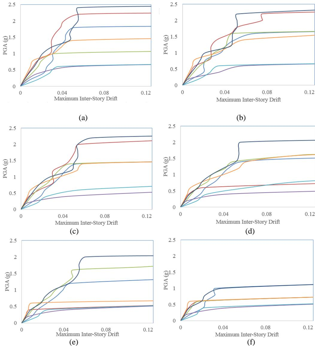
Figure 3. IDA curves for RC frame (a) pristine, (b) 10years, (c) 20 years, (d) 30 years, (e) 40 years, (b) 50 years.
