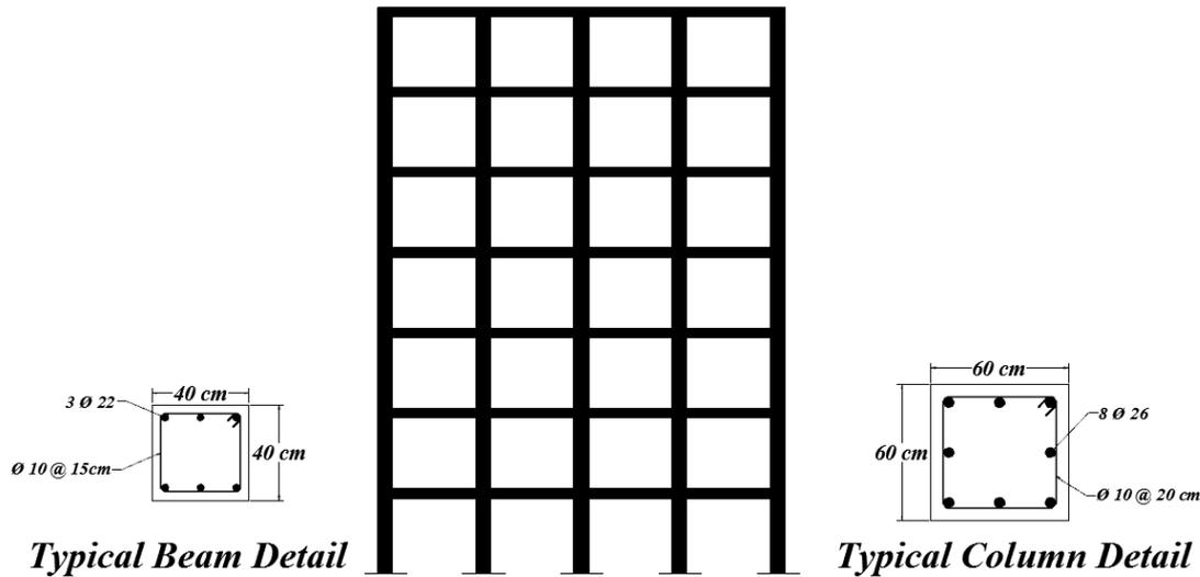
Figure 2. Schematic view of the RC frame and section details
