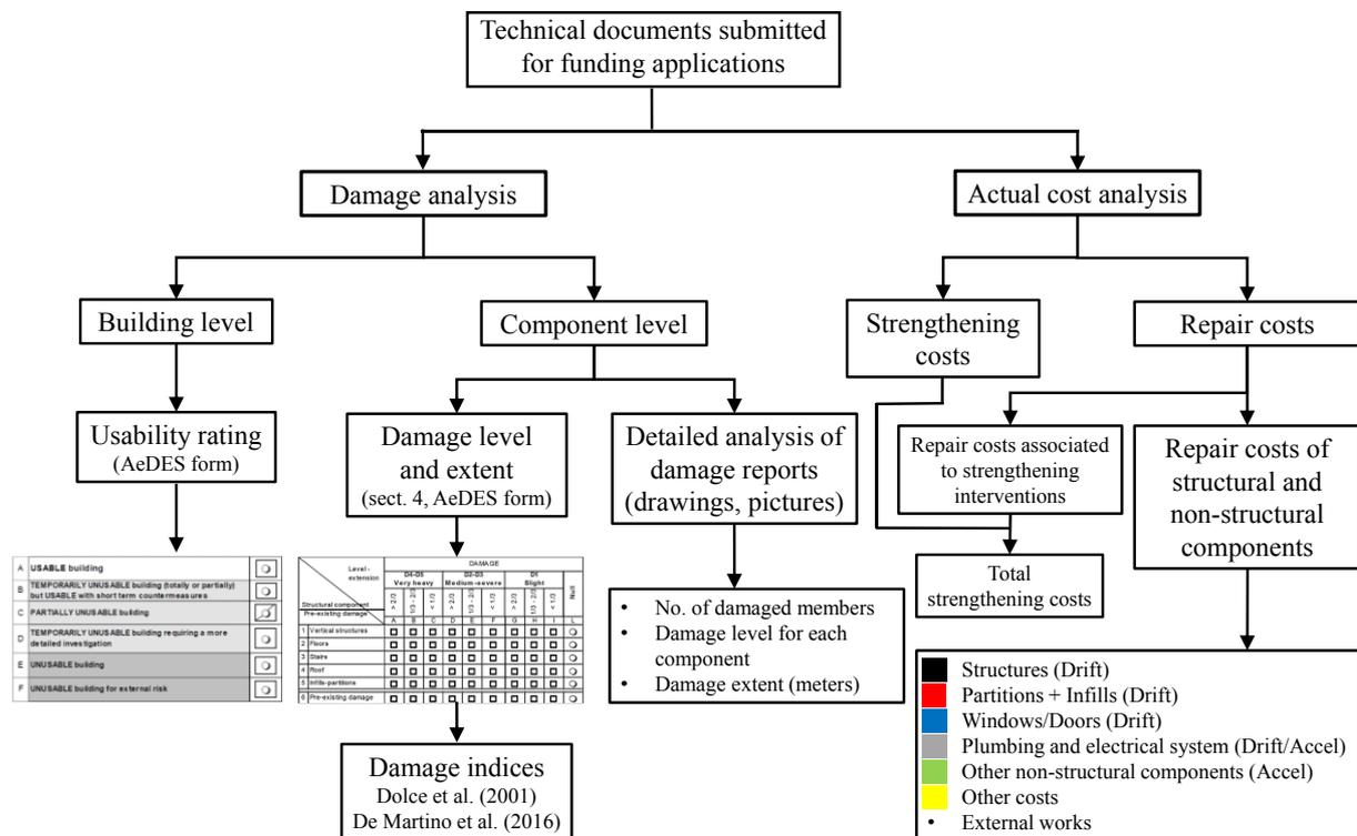
Figure 2. Methodology for damage and actual cost analysis.
