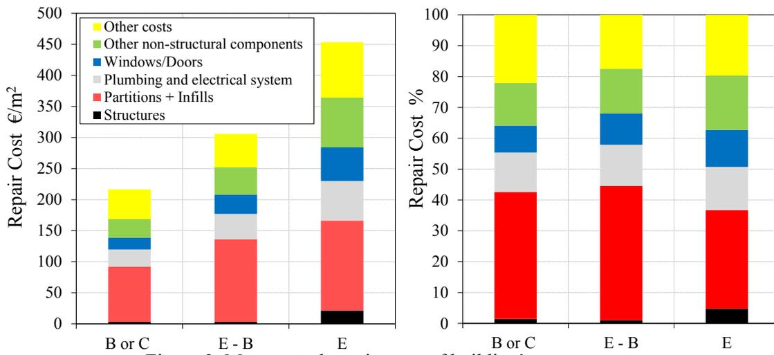
Figure 3. Mean actual repair costs of building's components.
