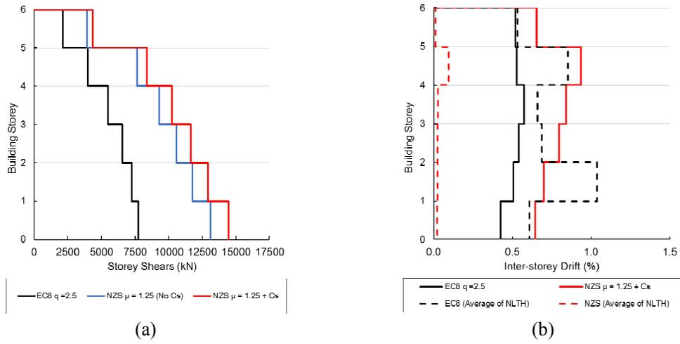
Figure 5. Comparison of (a) storey shears and (b) inter-storey drifts for MRSA for EC8 and NZS
