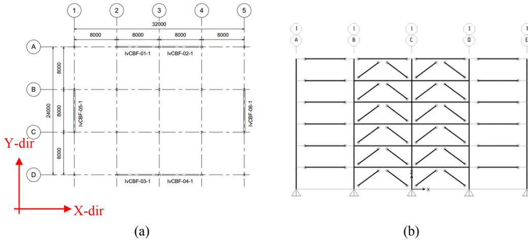
Figure 3. Reference building (a) typical floor plan and (b) x-dir brace layout for 6-storey building
