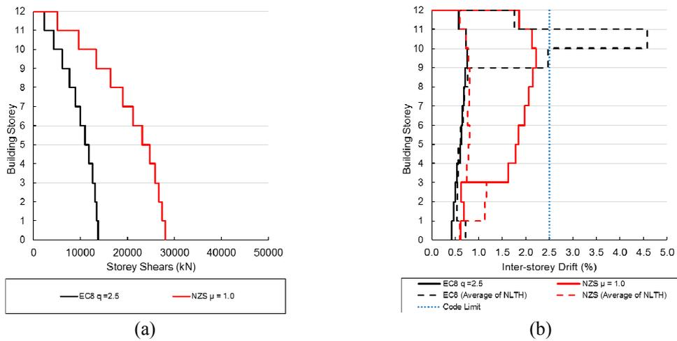
Figure 6. Comparison of (a) storey shears and (b) inter-storey drifts for MRSA for EC8 and NZS
