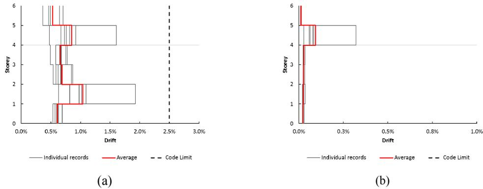
Figure 8. Comparison of inter-storey drifts of NLTH analysis for (a) EC8 and (b) NZS – 6 storey building
