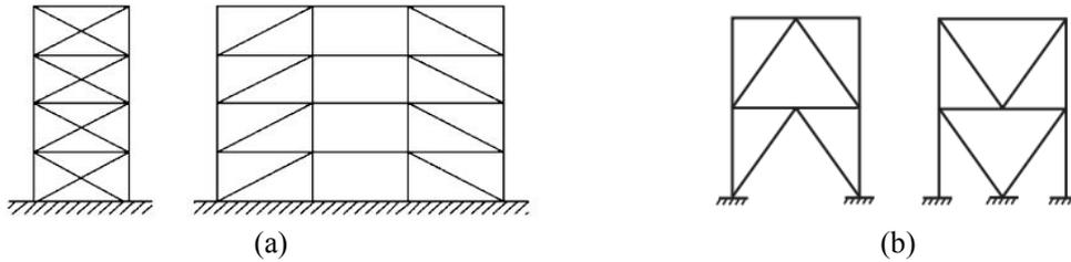
Figure 1. Typical concentric braced frames, (a) concentric bracing and (b) V-bracings
