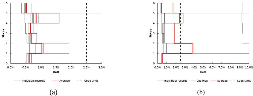
Figure 10. EC8 drifts from NLTH analysis for 6 storey building with (a) no degradation and (b) degradation
