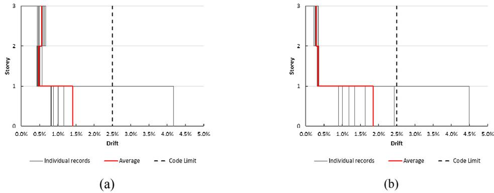
Figure 7. Comparison of inter-storey drifts of NLTH analysis for (a) EC8 and (b) NZS – 3 storey building
