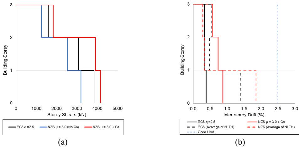
Figure 4. Comparison of (a) storey shears and (b) inter-storey drifts for EC8 and NZS
