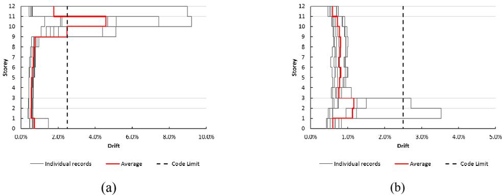
Figure 9. Comparison of inter-storey drifts of NLTH analysis for (a) EC8 and (b) NZS – 12 storey building
