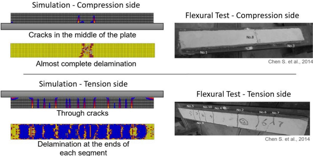
Figure 4. Simulation results and test result comparison on the failure modes of cementitious SFRM coated steel plates under flexural loading
