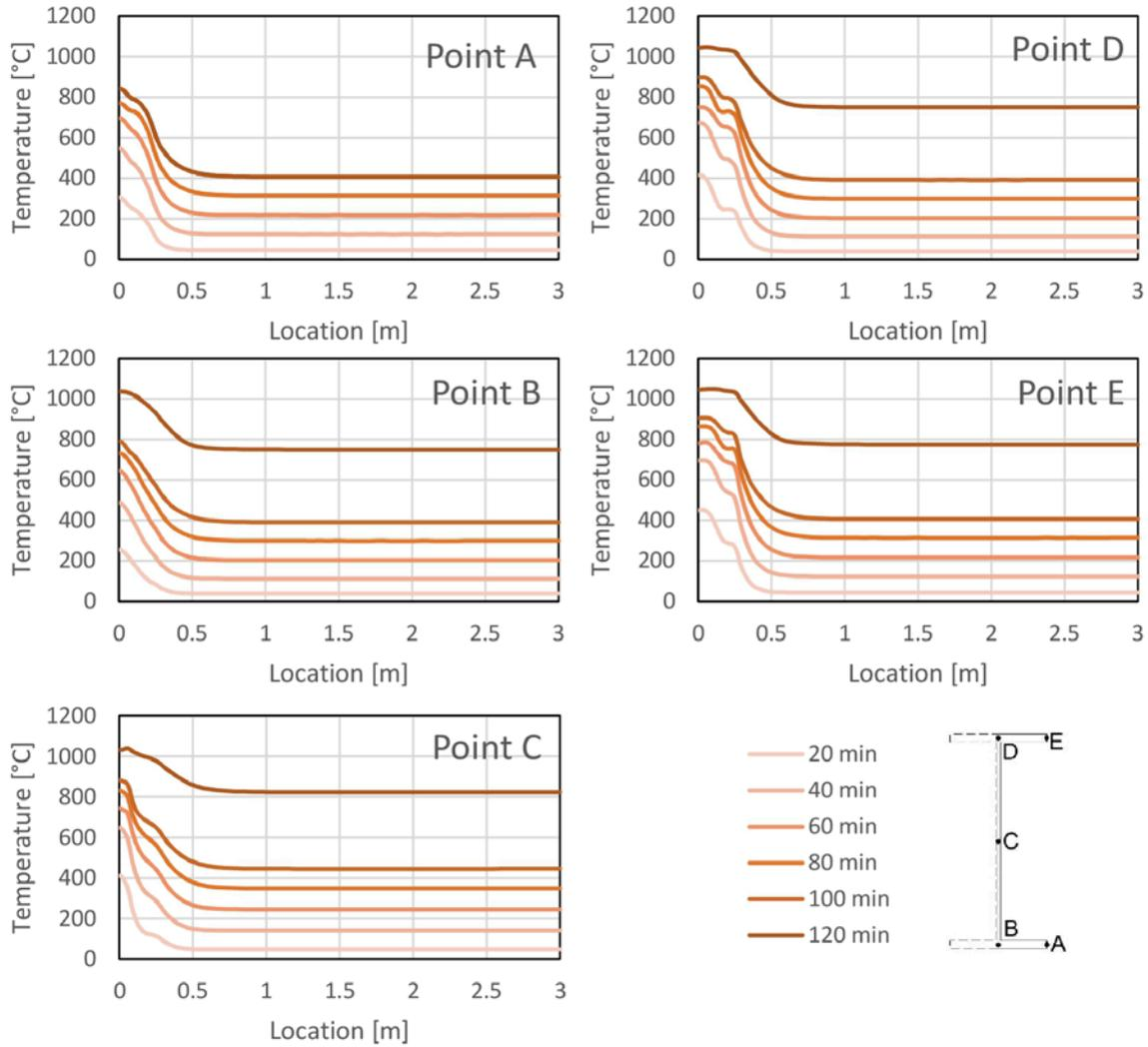
Figure 10. Temperature distribution along the length of the steel beam with the partially damaged SFRM coating
