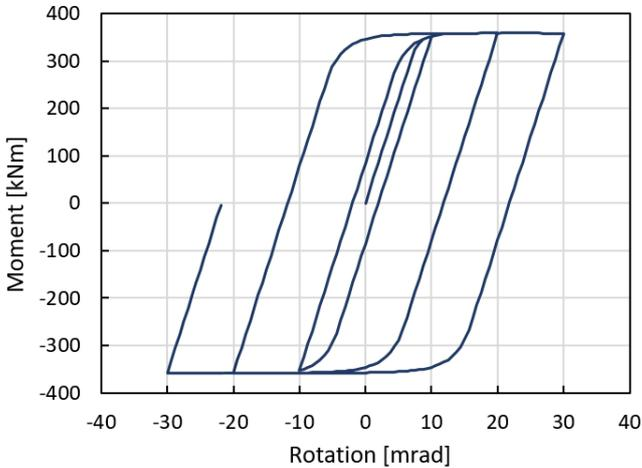
Figure 6. Moment - Rotation curve applied on IPE400 beam
