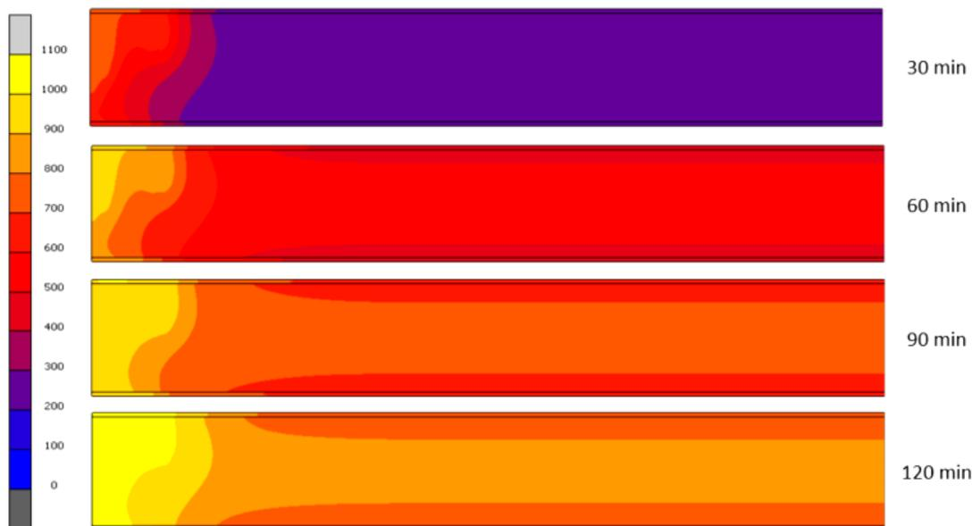
Figure 12. Temperature distribution along the length of the steel beam with the partially damaged SFRM coating.
