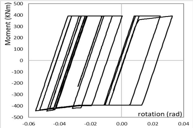
Figure 3. The moment rotation curve for joint 1 of the steel frame
