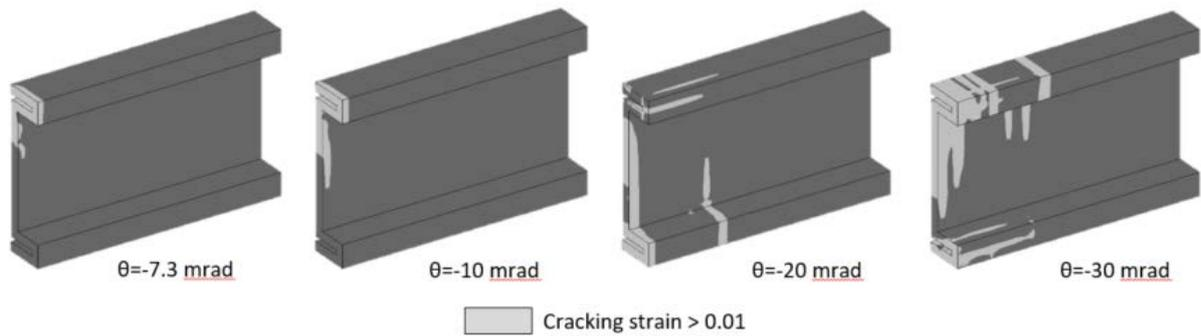
Figure 8. Evolution of SFRM coating damage (cracking strain) against imposed rotation
