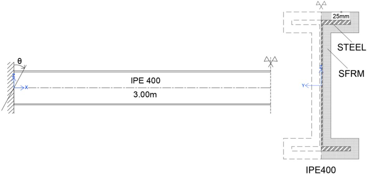
Figure 5. Structural model and cross section
