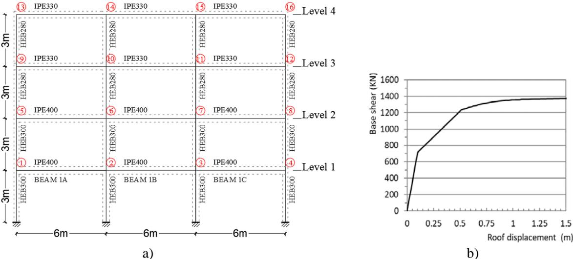
Figure 1. a) The static pushover curve for the steel frame, b) The static pushover curve for the steel frame
