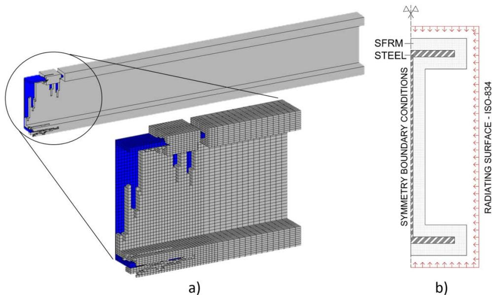
Figure 9. a) Model of the beam with partially damaged SFRM coating at the area of the plastic hinge, b) Thermal model and boundary conditions
