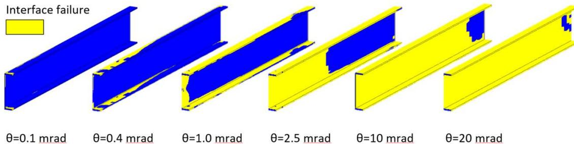
Figure 7. Evolution of interface failure against imposed rotation
