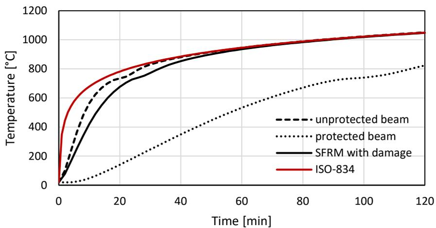
Figure 11. Maximum temperature-time history for the protected, unprotected and partially damaged beam
