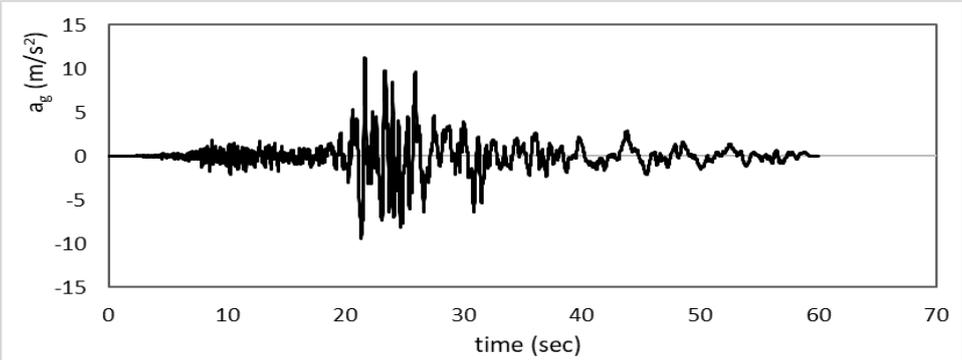
Figure 2. The accelerogram used for the non-linear time- history analysis
