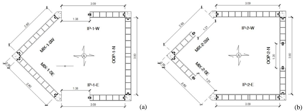
Figure 2. Infills distribution at storey 1 (a) and storey 2 (b) of the model building (dimensions in m).
