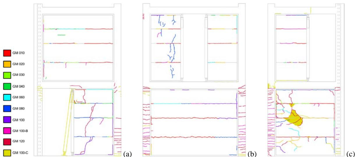
Figure 5. Cracking pattern of outer side of the E (a), N (b) and S-E (c) façades of the model.
