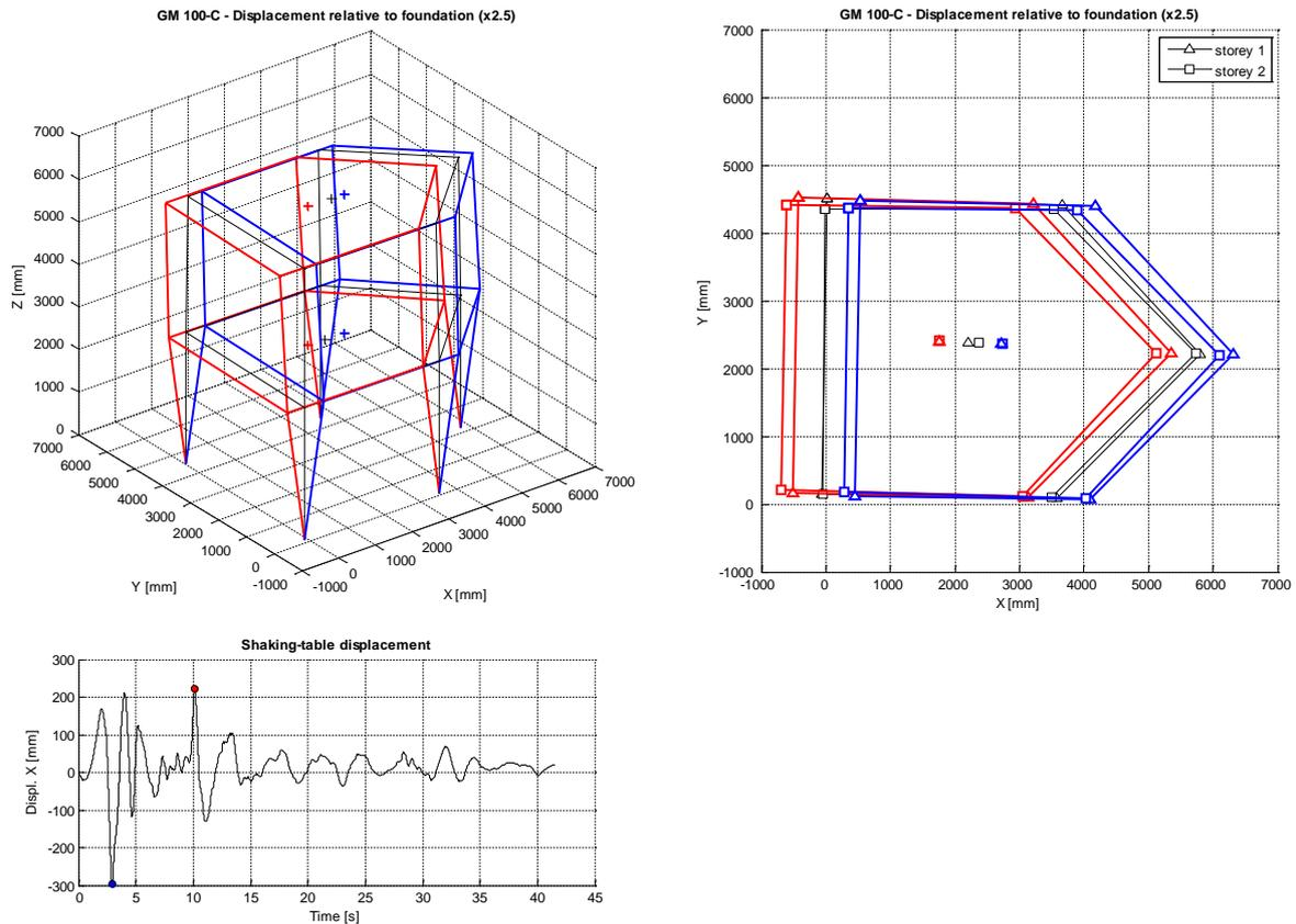
Figure 10. GM 100-C: Deformed shape of the model building at maximum (red lines) and minimum (blue lines) displacement of the shaking table.
