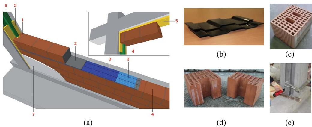
Figure 1. (a) Details of the innovative masonry infill with sliding joints: 1.(c) C-shape units; 2. mortar bed-joints; 3.(b) sliding joints; 4.(d) clay units; 5. interface joints; 6.(e) shear keys; 7. plaster.
