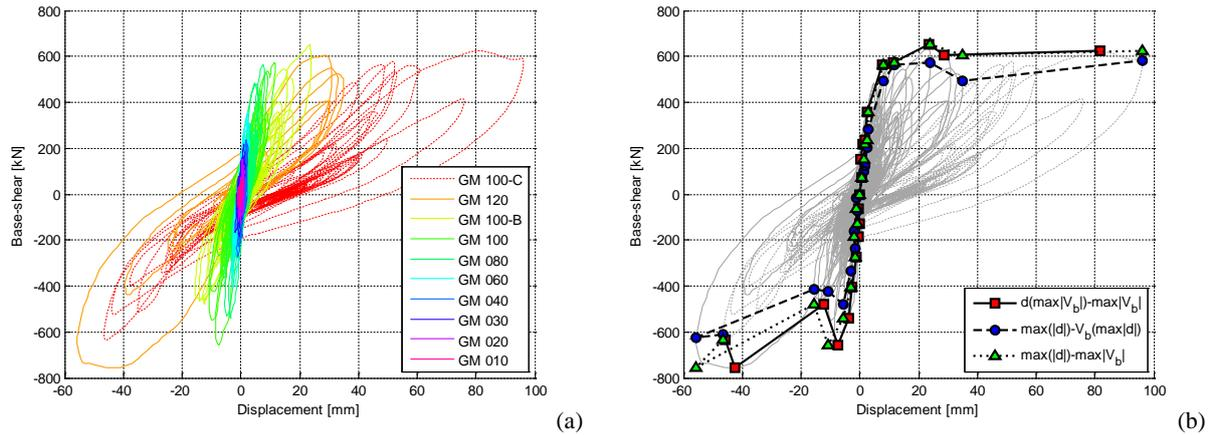
Figure 8. Total hysteretic response of the model building (a) and corresponding envelopes (b).
