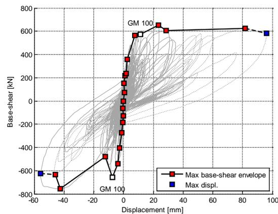
Figure 9. Maximum base-shear envelope of the total hysteretic response of the model building.
