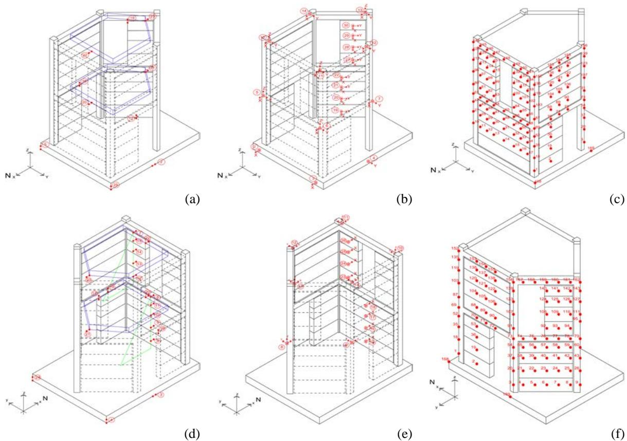
Figure 3. Scheme of the disposition of the instrumentation on the model building: potentiometers (a, d); accelerometers (b, e); optical passive target markers (c, f).
