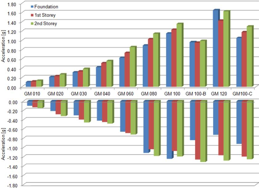
Figure 7. Maximum/Minimum accelerations recorded at each level of the model building.
