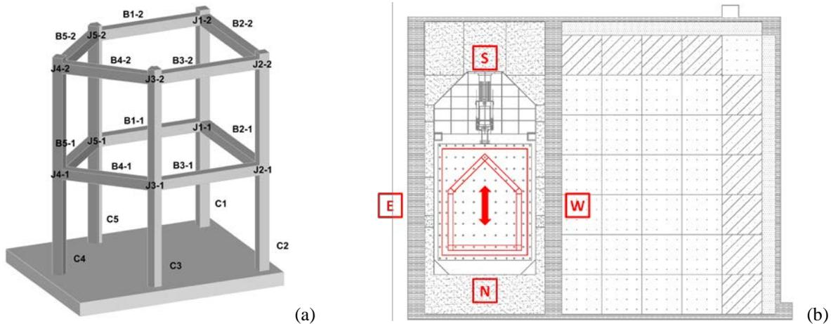
Figure 1. (a) 3D-sketched of the RC structure, with identification of beams (B), columns (C) and joints (J); (b) Plan view of the EUCENTRE laboratory and position of the shake-table and of the model building.
