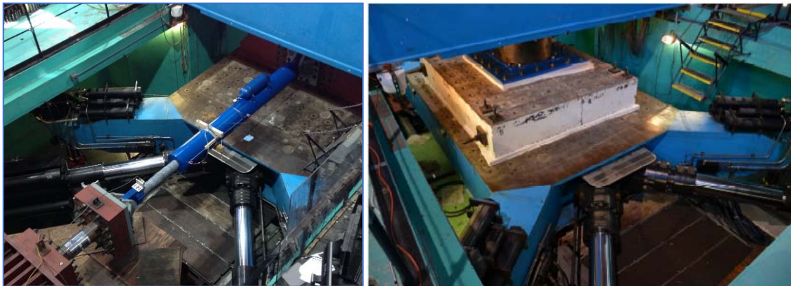
Figure 8: Tests on FD (left) and HDRB (right) at San Diego
