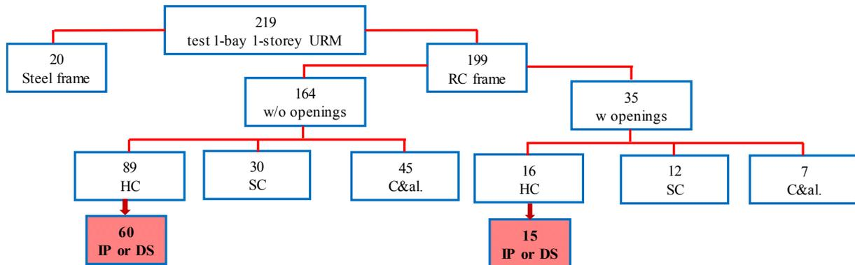
Figure 1. Collected database from literature (URM = Unreinforced masonry infills; HC = hollow clay bricks; SC = solid clay bricks; C&al. = concrete blocks or other material; DS = description of Damage State evolution available; IP = In-Plane response available (i.e. corresponding experimental bare frame available)
