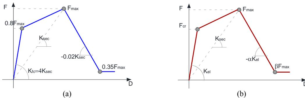
Figure 2. Force-displacement envelopes for infills according to models by Bertoldi et al. (1993) (a) and Panagiotakos and Fardis (1996) (b)
