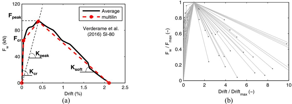
Figure 1. Example of evaluation of the experimental response of infill panel for test “SI-80” by Verderame et al. (2016) - analysed parameters (a); multi-linearized experimental responses of the investigated infills (b).
