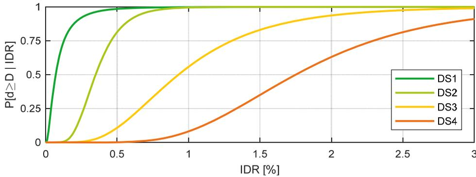
Figure 4. Proposed fragility function curves for hollow clay brick solid infill panels
