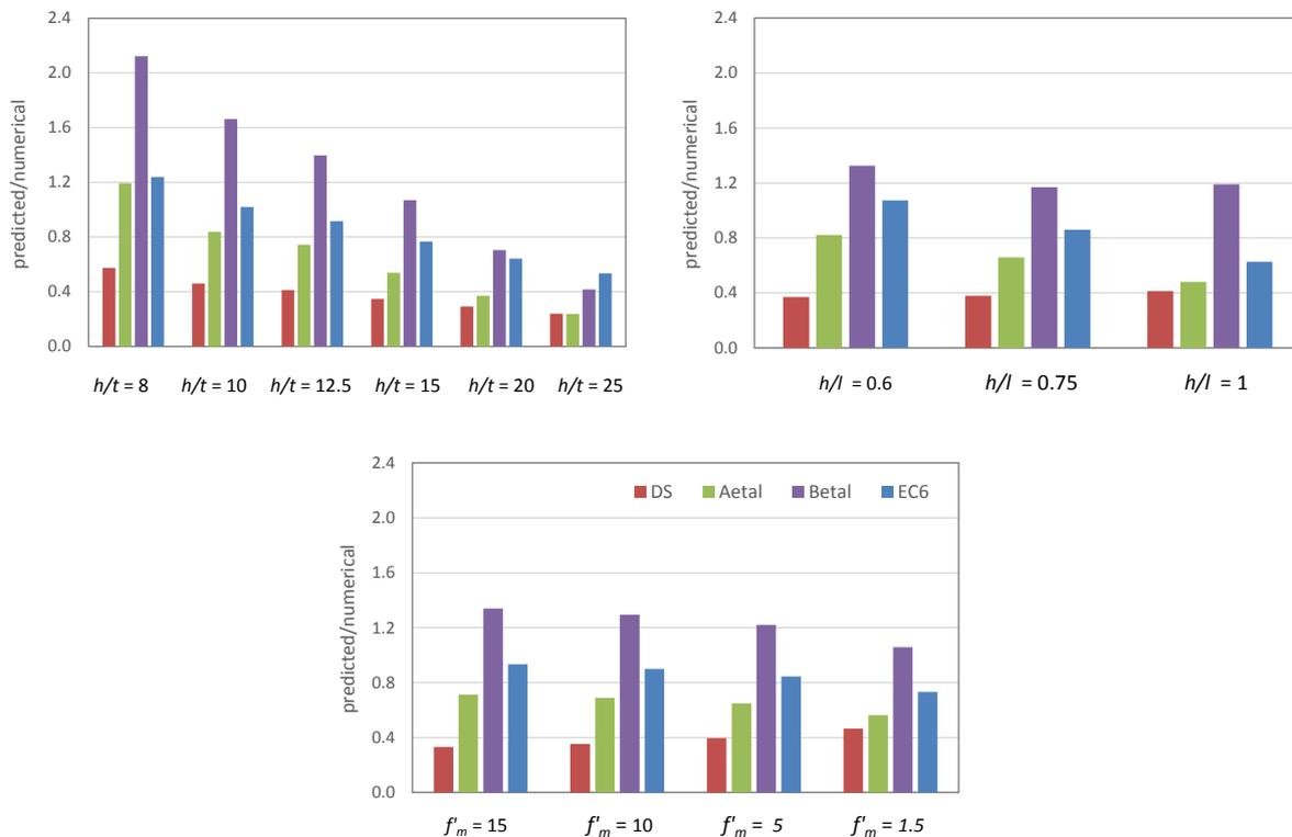
Figure 5. Mean ratio between the predicted and numerical strength. Data are grouped according to slenderness ratio ( $h/t$ ), height/length ratio ( $h/l$ ) and masonry compressive strength ( $f'_m$ ). DS = Dawe and Seah (1989), Aetal = Angel et al. (1994) and Abrams et al. (1996), Betal = Bashandy et al. (1995), EC6 = Eurocode 6 (2005).
