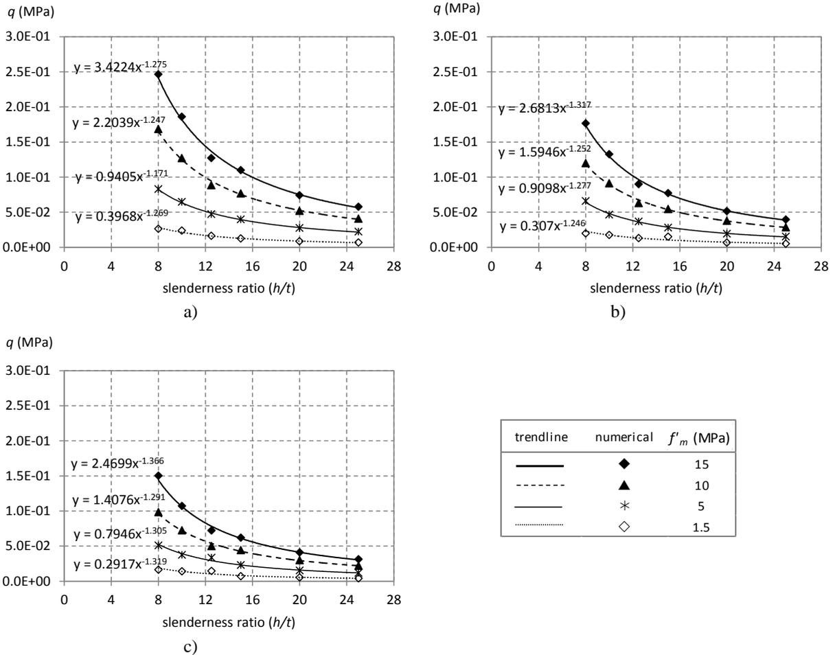
Figure 3. Out-of-plane strength: a)  $h/l = 1$  (panel  $3 \times 3$  m<sup>2</sup>); b)  $h/l = 0.75$  ( $3 \times 4$  m<sup>2</sup>); c)  $h/l = 0.6$  ( $3 \times 5$  m<sup>2</sup>). Trend-lines are also reported, where  $y$  represents the strength per unit area,  $q$ , and  $x$  is the height/thickness ratio,  $h/t$ .
