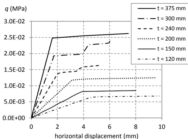
Figure 2. Out-of-plane pressure versus horizontal displacement with varying infill thickness, infill characteristics:  $h = 3$  m,  $f'_m = 1.5$  MPa.
