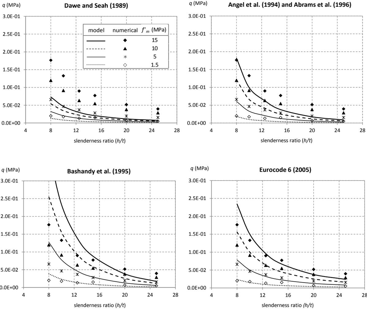
Figure 4. Out-of-plane strength, panel dimensions  $3 \times 4 \text{ m}^2$ , comparison between numerical values (present study) and analytical models (Table 2).
