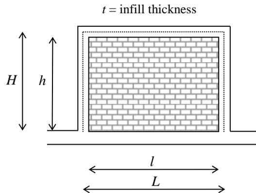
Figure 1. One-bay one-storey infilled frames.
