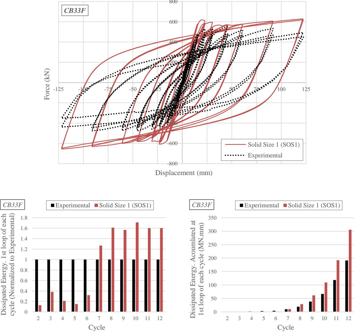
Figure 3. CB33F specimen simulation. Solid size 1 model.
