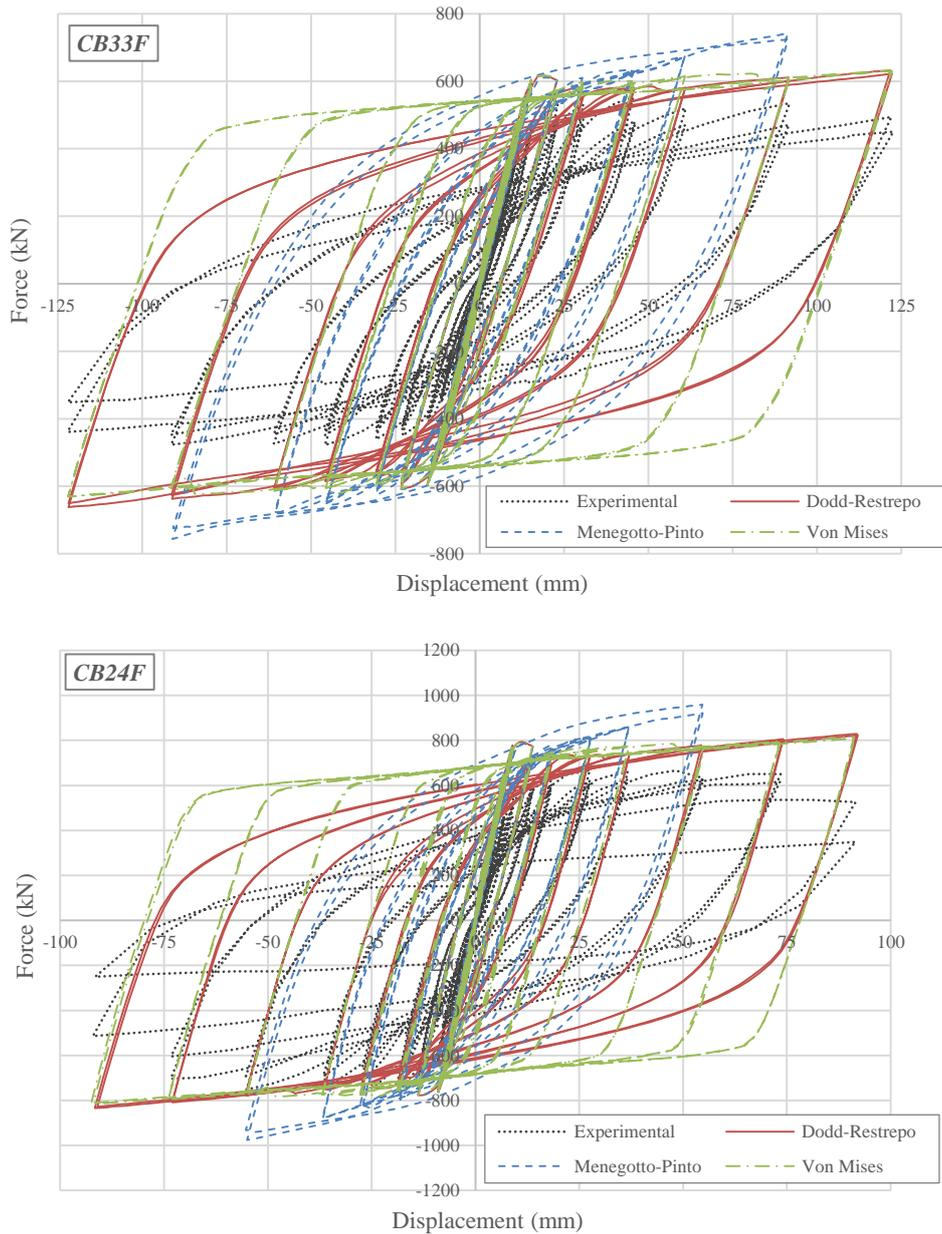
Figure 6. Comparison of reinforcing steel models for CB33F and CB24F specimens. Shell Size 1 model (SHS1).
