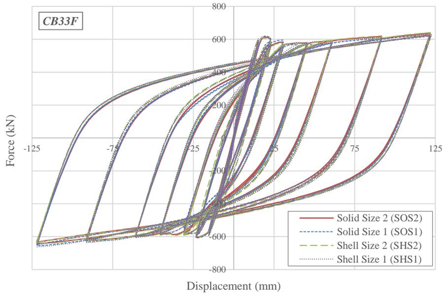
Figure 5. CB33F results with different mesh types and sizes.
