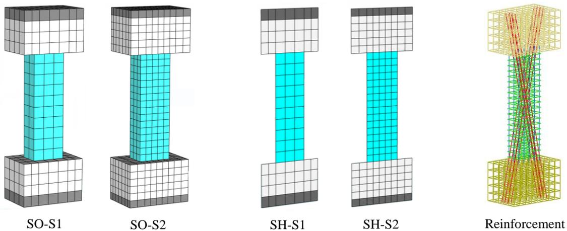
Figure 2. Model mesh definitions illustrated for CB33F specimen.
