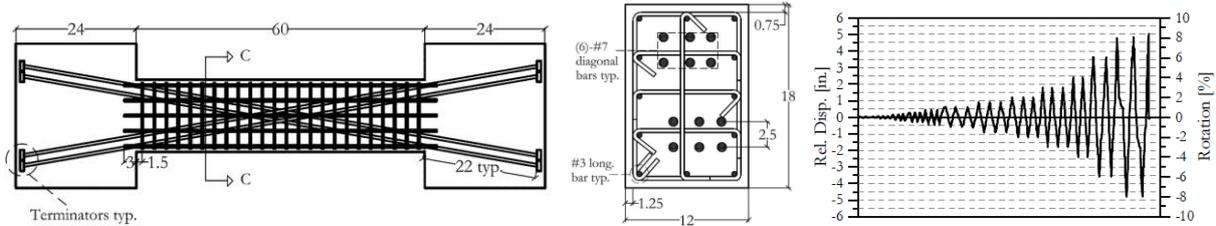
Figure 1. Characteristics and loading of the specimens CB24F and CB33F. (Naish, 2010)
