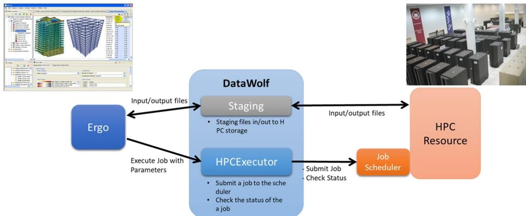
Figure 2. HPC Workflow
