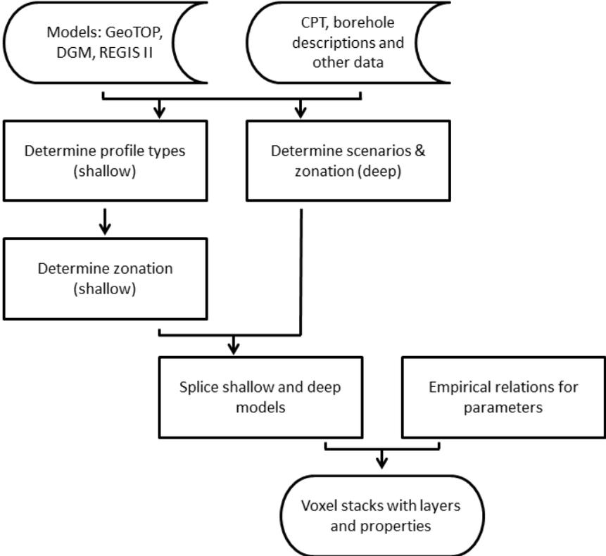
Figure 7. Flow chart of steps to obtain input for site response calculations.
