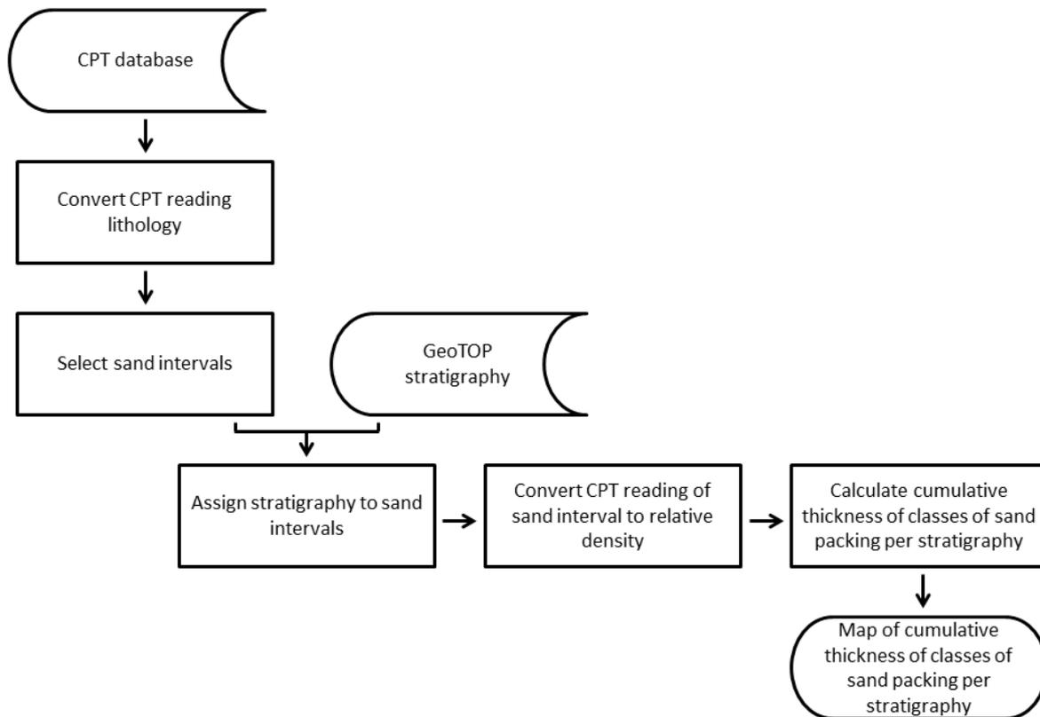
Figure 6. Flow chart of steps to obtain relative densities from CPTs for liquefaction potential analysis.
