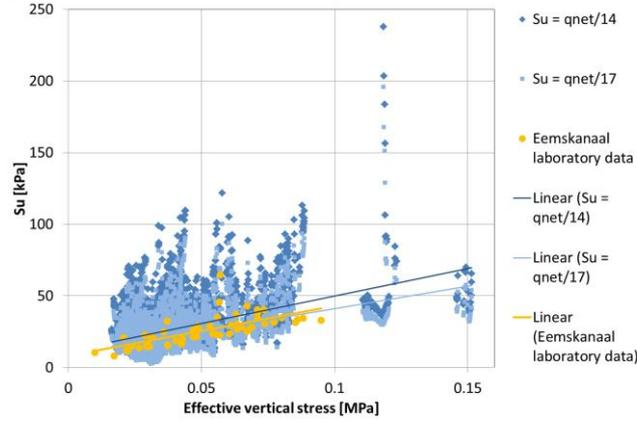
Figure 3. CPT derived and laboratory data for  $S_u$  for Naaldwijk clay, including linear regression lines.
