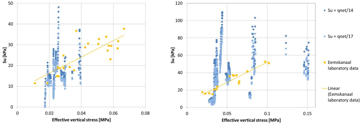
Figure 4. CPT derived (blue) and laboratory data (orange) for  $S_u$  including linear regression line. Left: for Holland peat. Right: for Basal peat.
