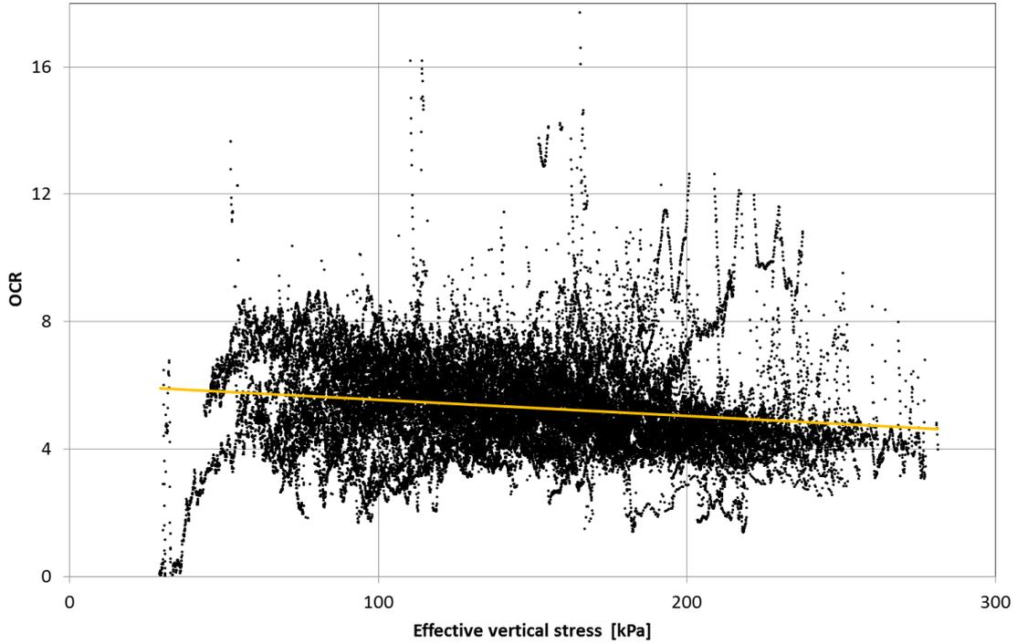
Figure 5 OCR for Peelo clay, derived from CPT data and related to effective vertical stress. The black dots are data points, the orange line is the linear regression line.
