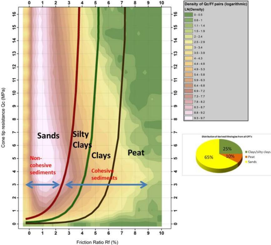
Figure 2. Density (logarithmic) of  $q_c$ - $R_f$  pairs in the Groningen CPT data base, representing all lithologies. The dividing lines between lithology types were adjusted from the nomogram of Douglas & Olson (1981) to fit the local conditions. The pie diagram shows that sandy lithologies dominate in this data set.
