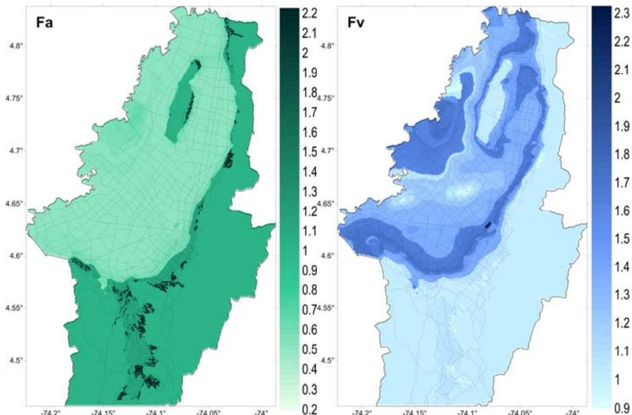
Figure 3. Maps of seismic design soil coefficients  $F_a$  and  $F_v$  (ACI 318) for Bogotá, Colombia, computed in SMS. From Cardona et al. (2016). After Cardona and Yamin (1997).
