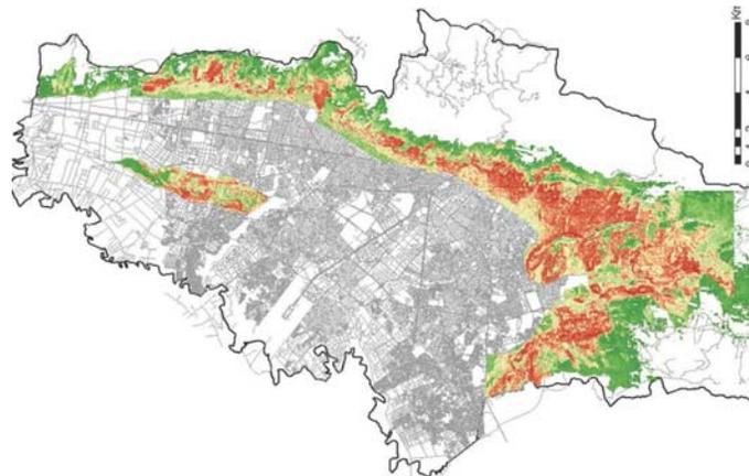
Figure 4. Landslide susceptibility for Bogotá, Colombia, calculated with LHM. From Cardona et al. (2016)
