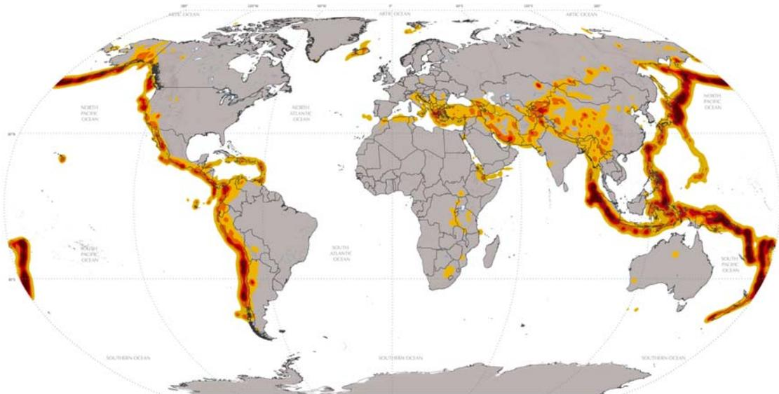
Figure 2. Seismic hazard map for the globe. PGA for 1000 years return period. Calculated with CRISIS 2015 for the Global Assessment Report, GAR, Atlas of Risk (UNISDR 2017; Marulanda et al. in these proceedings).
