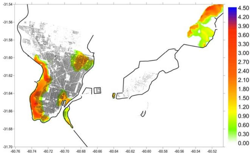
Figure 8. Flood hazard map of Santa Fe, Argentina. 100 years return period. Calculated with FA. The thick surrounding the city are dikes used for flood defense. (INGENIAR-CIMNE, 2015).
