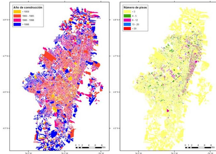
Figure 10. Maps of year of construction (left) and number of stories (right) of buildings in Bogotá, Colombia, from a database of 897,583 buildings created with Exposure Editor. From Cardona et al. (2016)
