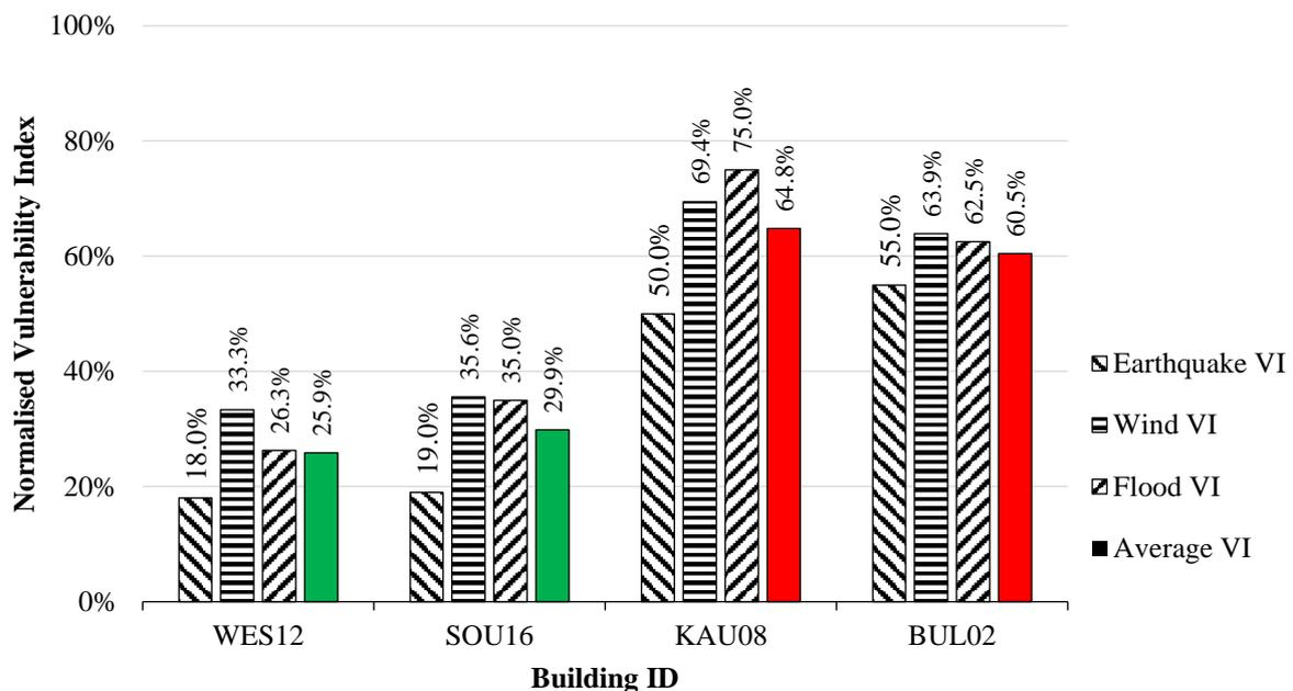
Figure 7. Evaluated vulnerability index of buildings based on the different hazards
