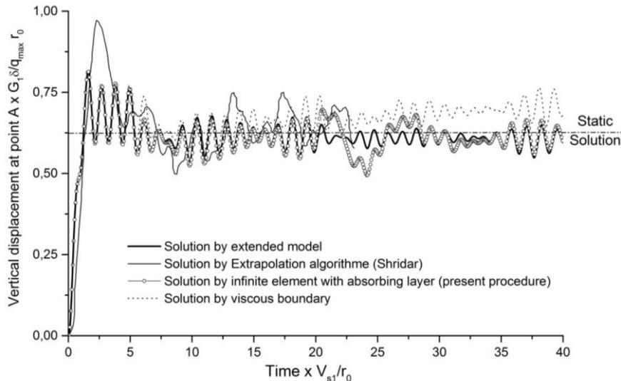
Figure 10. Comparison with responses obtained by extrapolation algorithm and by viscous boundary
