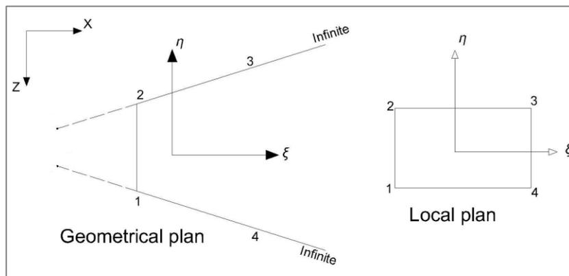
Figure 1. Local and global representation of an infinite element
