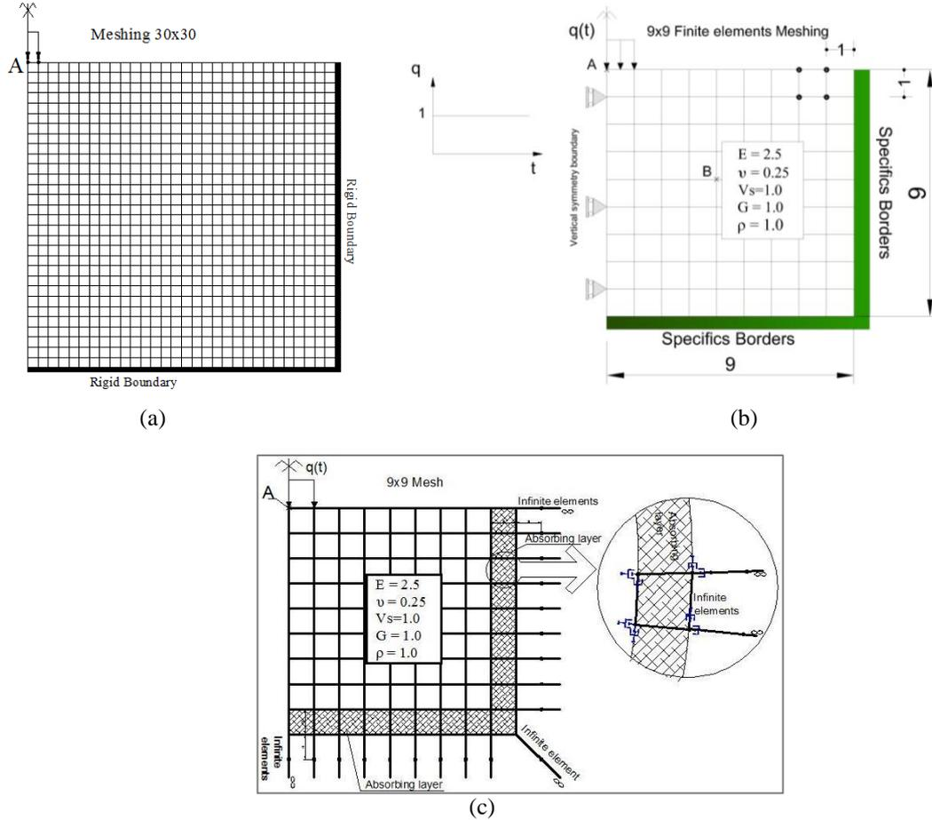
Figure 4. (a) The large model, (b) The used model, (c) model of method proposed
