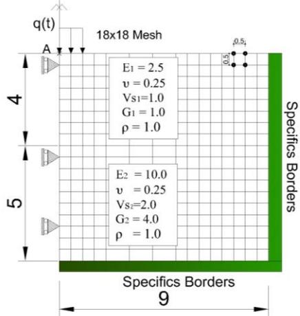
Figure 8. Two-layer model under a heavy side loading
