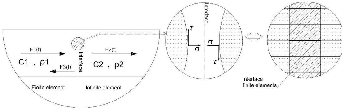
Figure 3. Absorbing interface schematization
