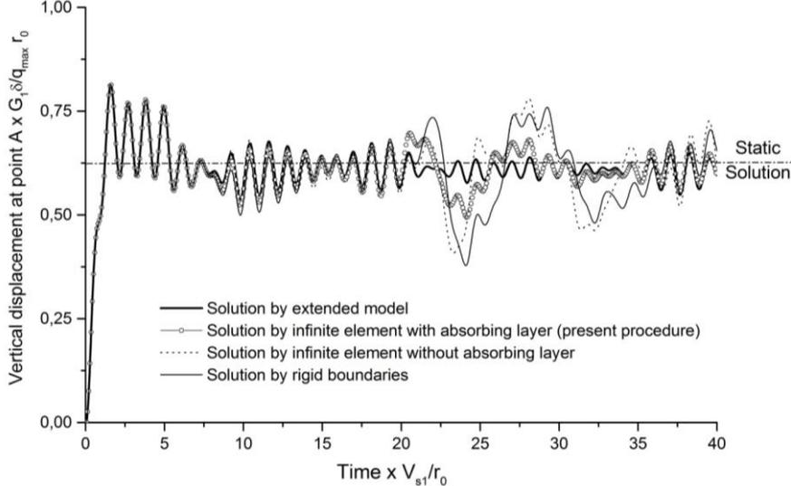
Figure 9. Comparison with responses obtained by direct infinite elements and rigid boundaries
