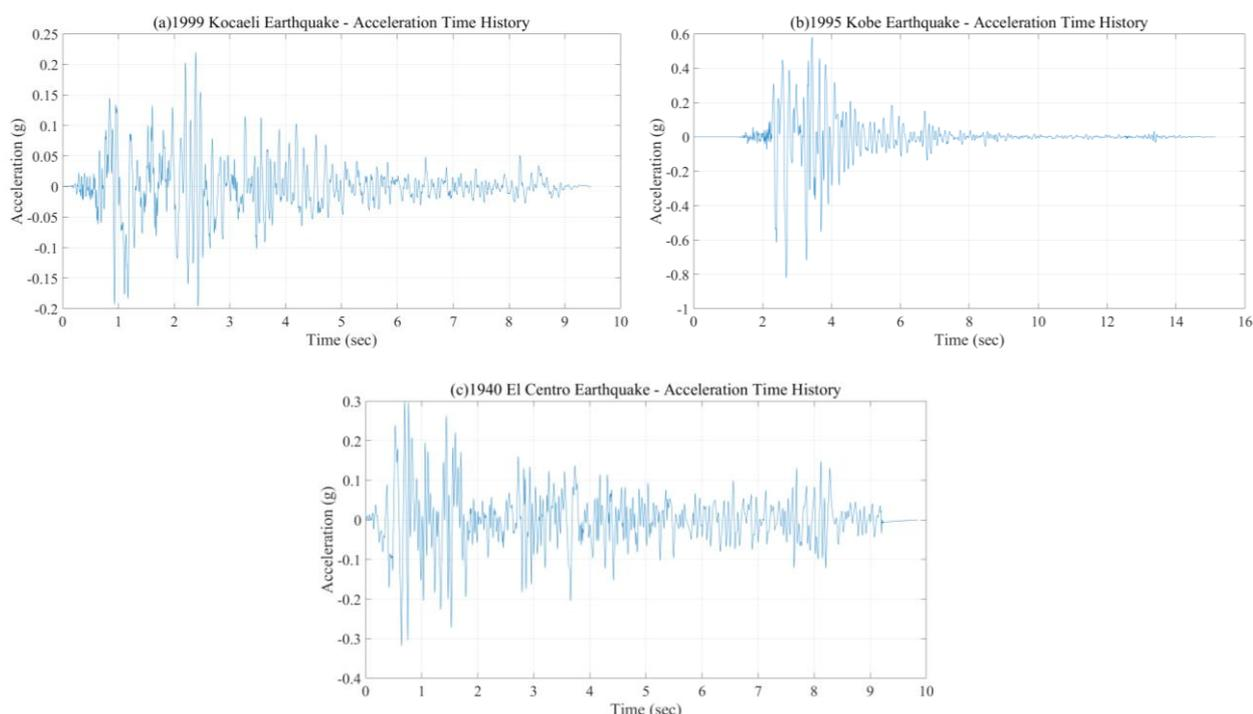
Figure 3. Scaled input motions (a) Kocaeli earthquake, (b) Kobe earthquake, (c) El Centro earthquake
