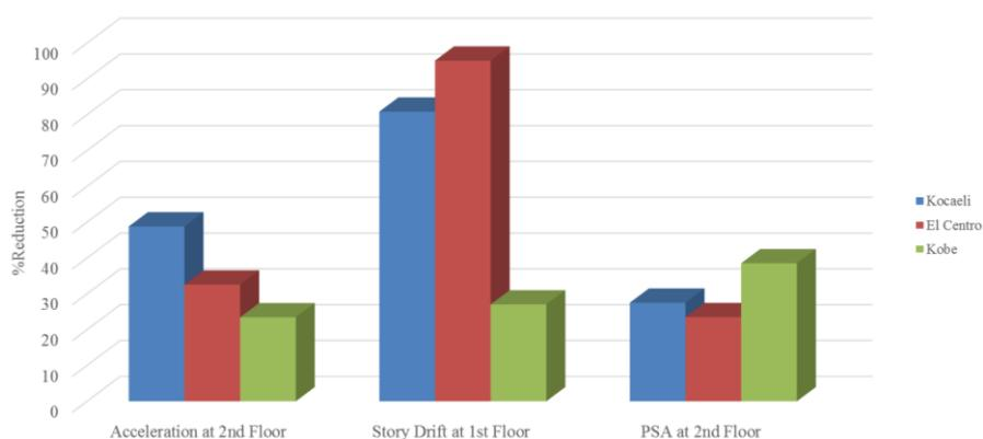
Figure 7. Reductions in acceleration, story drift and peak spectral acceleration values under three earthquakes
