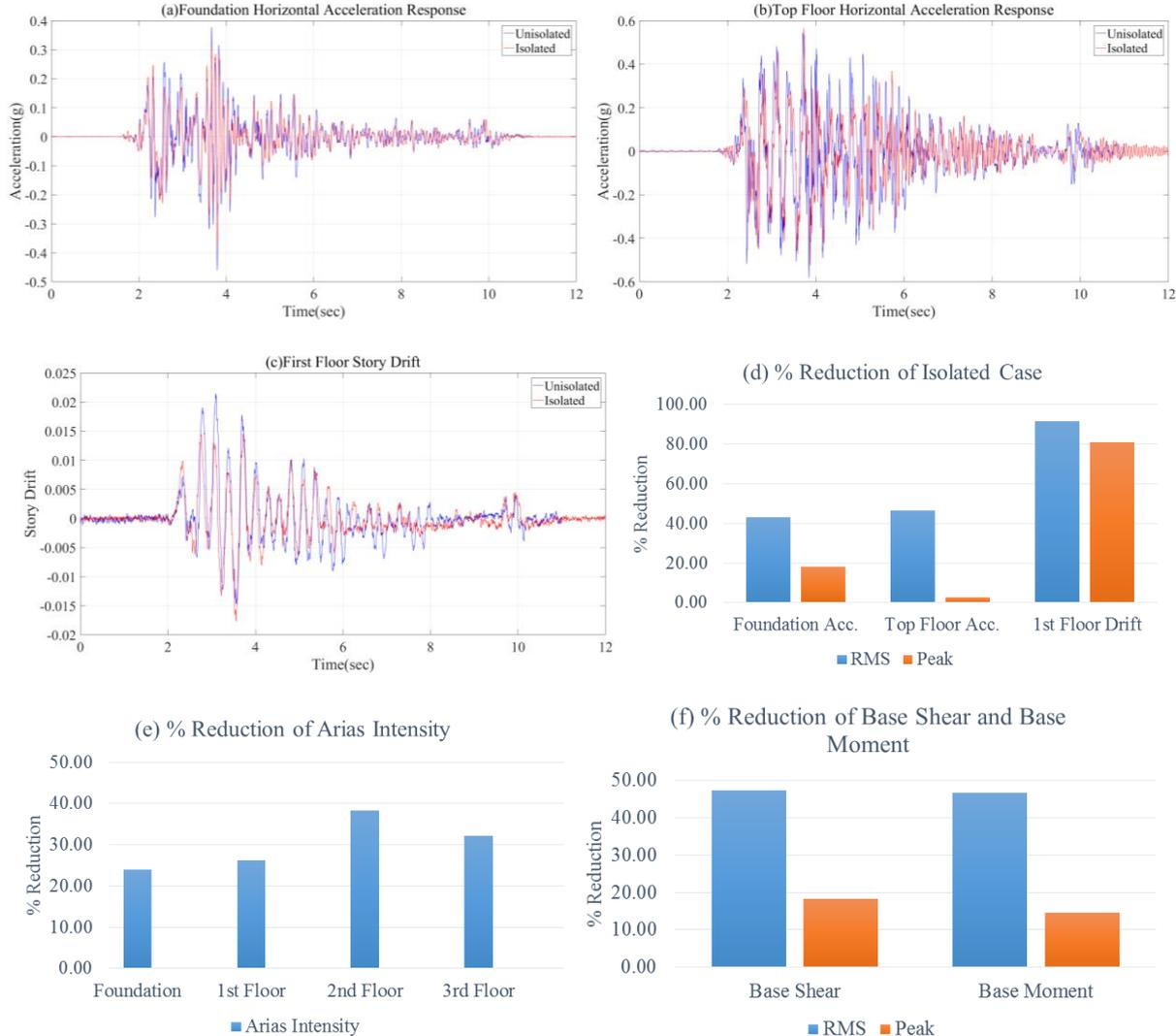
Figure 4. (a) Foundation acceleration response, (b) Top floor acceleration response, (c) First floor drift response, (d) % Reduction of isolated case, (e) % Reduction of Arias intensity, (f) % Reduction of base shear and base moment under Kocaeli Earthquake
