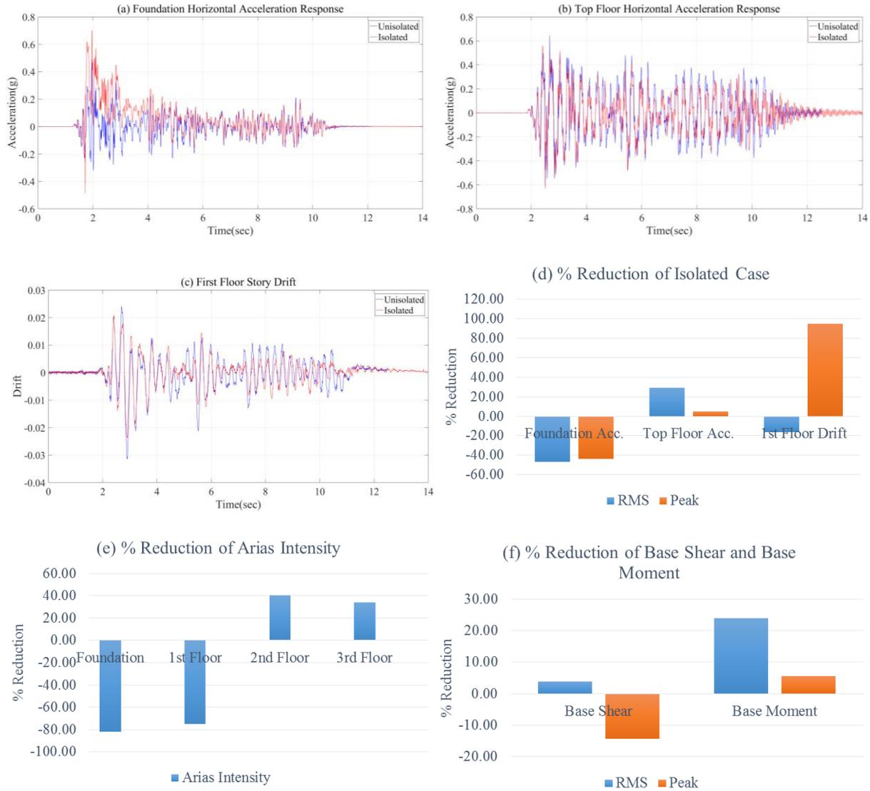
Figure 6. (a) Foundation acceleration response, (b) Top floor acceleration response, (c) First floor drift response, (d) % Reduction of isolated case, (e) % Reduction of Arias intensity, (f) % Reduction of base shear and base moment under El Centro Earthquake.
