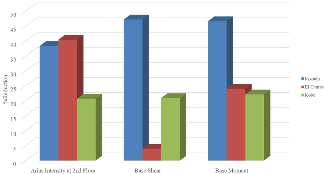
Figure 8. Reductions in Arias intensity, base shear and base moment values under three earthquakes
