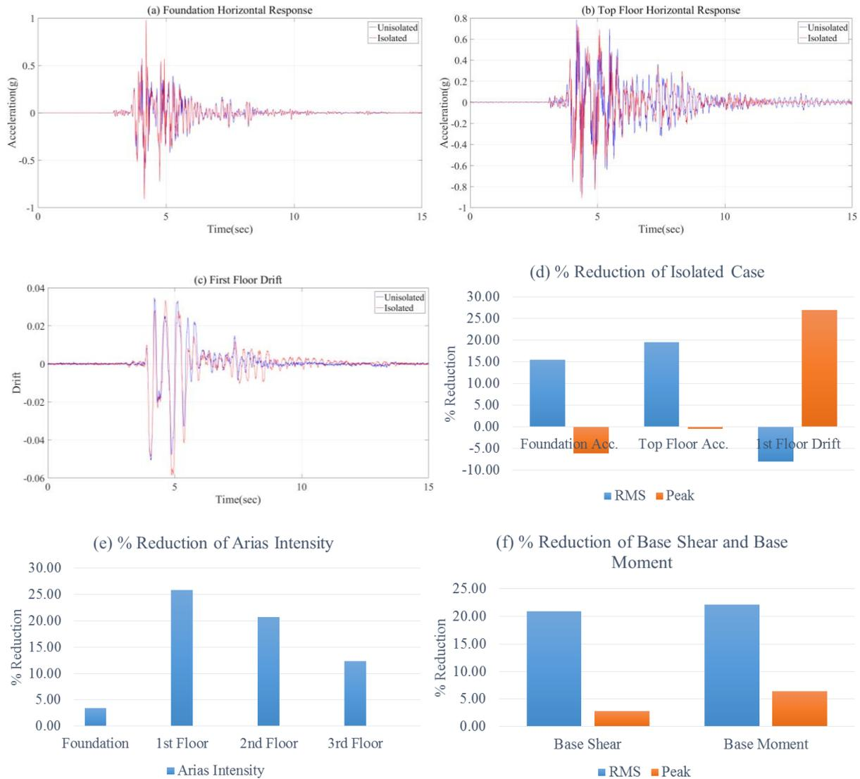
Figure 5. (a) Foundation acceleration response, (b) Top floor acceleration response, (c) First floor drift response, (d) % Reduction of isolated case, (e) % Reduction of Arias intensity, (f) % Reduction of base shear and base moment under Kobe Earthquake.
