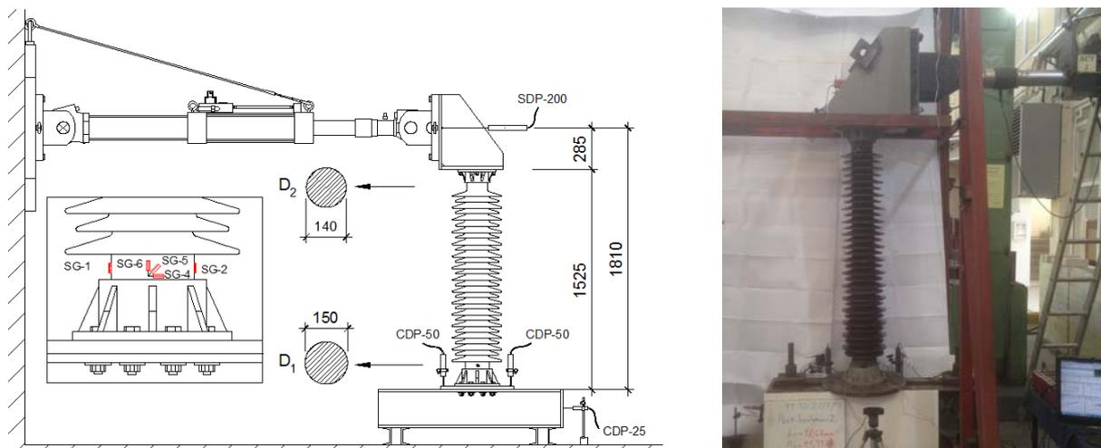
Figure 7. Specimen #2 testing set-up
