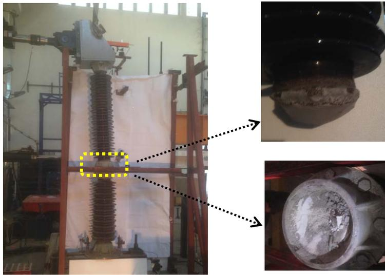
Figure 5. Specimen #1 failure mechanism
