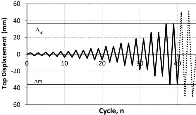
Figure 1. Cyclic displacement loading pattern
