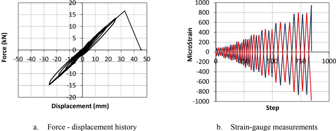
Figure 8. Specimen #2 force displacement hysteresis and bending strain measurements on bottom section
