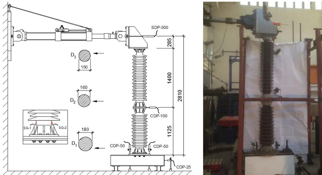
Figure 2. Specimen #1 testing set-up
