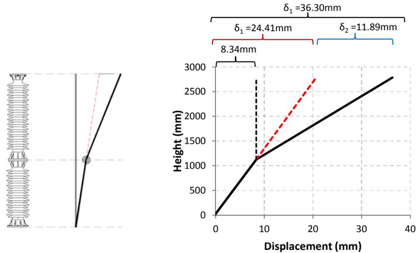
Figure 6. Displacement distribution of Specimen #1
