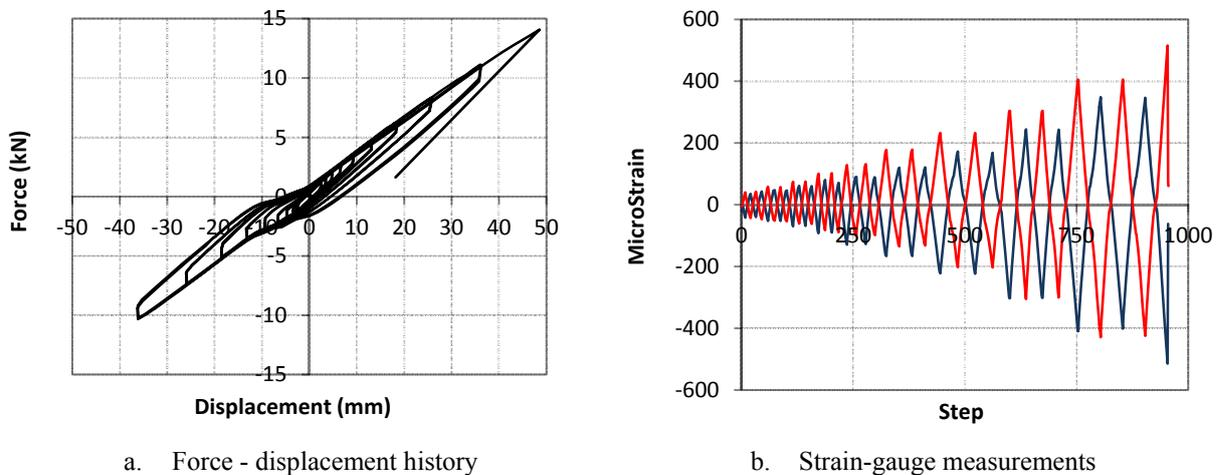
Figure 3. Specimen #1 force displacement hysteresis and strain-gauge measurements on the bottom section
