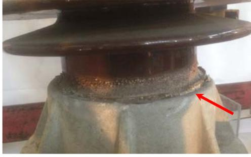
Figure 4. Grout failure between the porcelain and cap plate
