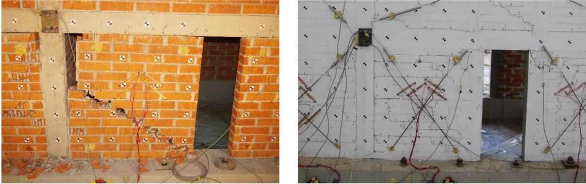
Figure 8. Observed damage to frame A on the first floor after the final tests in both series:
