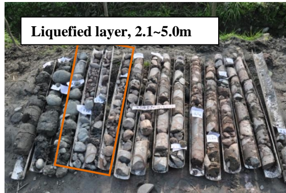
Figure 5 The extracted soil sample from the inspecting borehole in Jinxing village, Tangchang town
