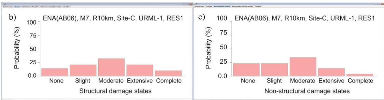
Fig. 4. Computation of seismic damage to single building in ER2: a) toolbar for input parameters and the standard 'summary report' form, and probability distribution of: b) structural and c) non-structural damage states
