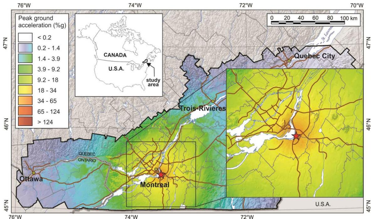
Figure 1. Peak ground acceleration for Montreal M6.0 point source scenario with depth of 10km
