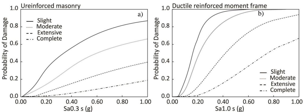
Figure 3. Fragility curves with closed form lognormal fit conditioned to spectral acceleration a)  $Sa_{0.3}$  for unreinforced masonry buildings and b)  $Sa_{1.0}$  for ductile moment frame low-rise buildings
