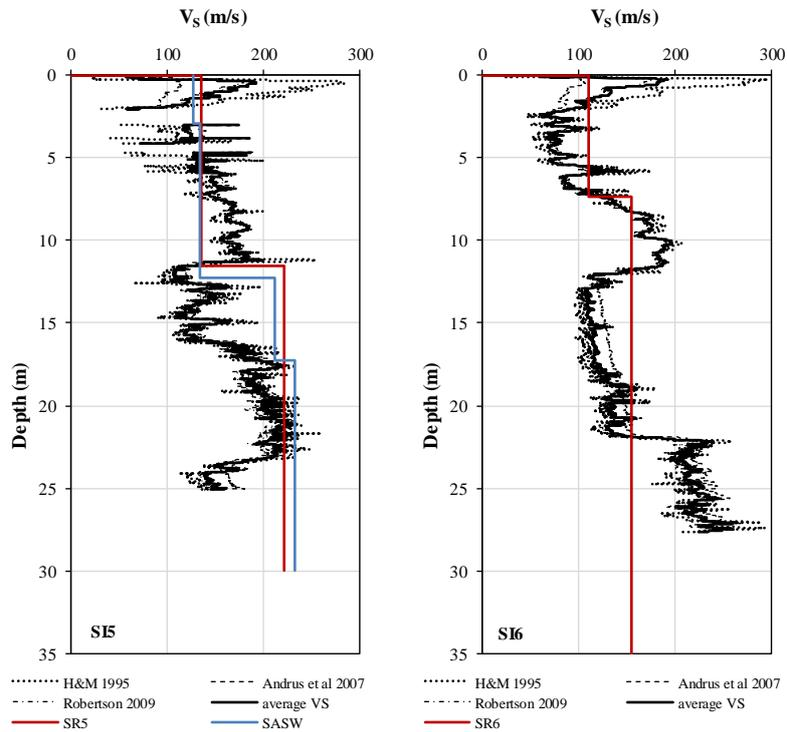
Figure 6. Estimated and measured  $V_s$  at SI5 (via CPT, SR, SASW) and SI6 (via CPT, SR)
