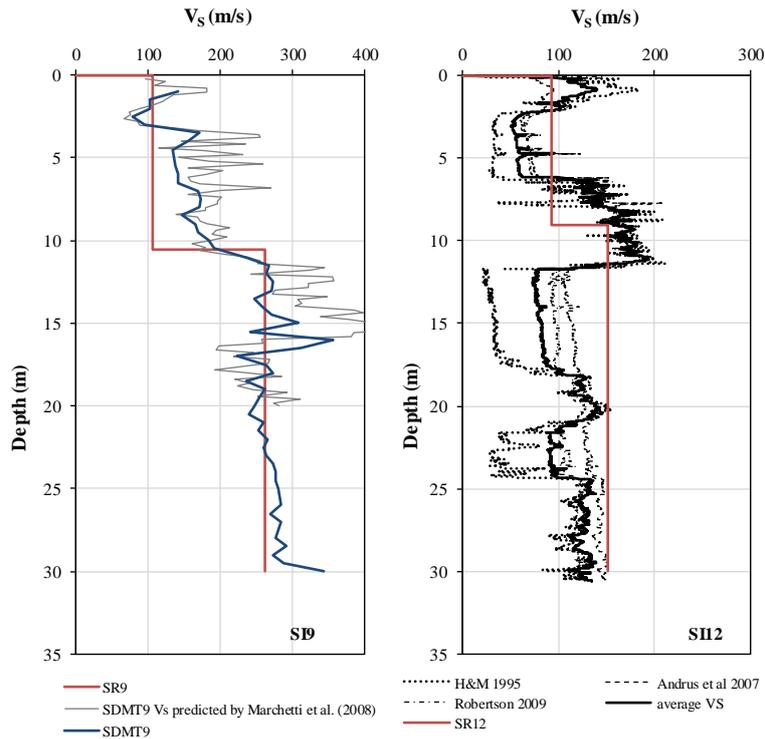
Figure 7. Estimated and measured  $V_s$  at SI9 (via DMT, SDMT, SR) and at SI12 (via CPT, SR)
