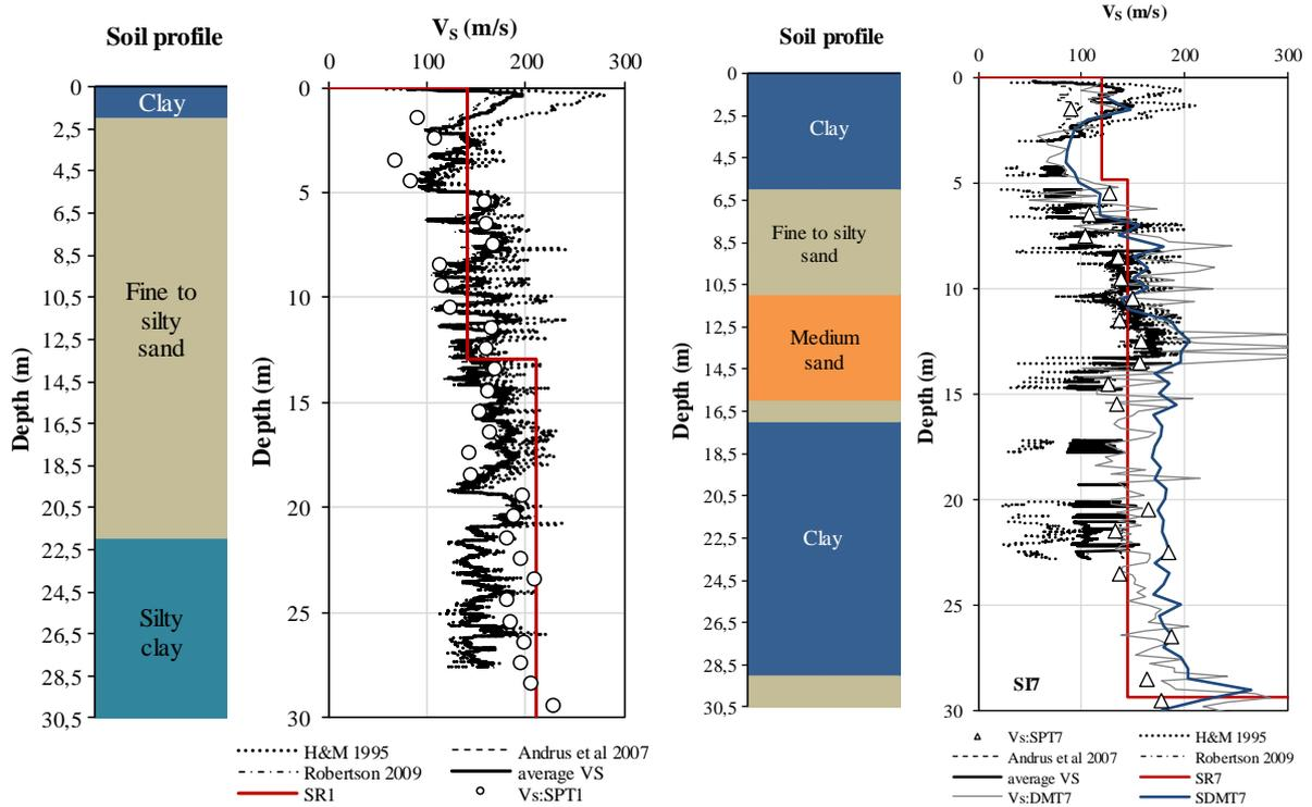
Figure 5. Estimated and measured  $V_s$  at SI1 (via SPT, CPTu, SR) and SI7 (via SPT, CPT, SR, SDMT)
