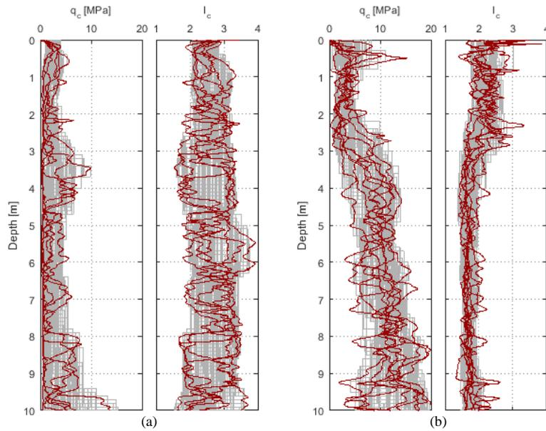
Figure 3. One hundred samples of randomized soil profiles (gray lines) for (a) Papanui and (b) Avondale. The red lines indicate the actual profiles used for the design and calibration of the probabilistic model in each sub-region.
