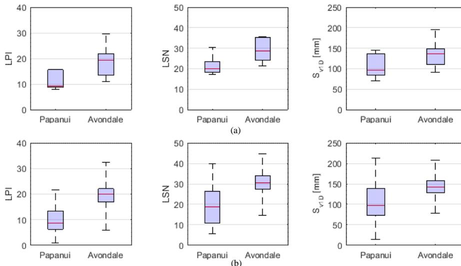
Figure 4. Comparison of the variation in liquefaction damage indices between (a) the actual soil profiles, and (b) the simulated soil profiles.
