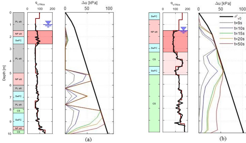
Figure 6. Evolution of excess pore water pressures for the (deterministic) soil profiles of Figure 2 under a CACS-based motion excitation: (a) Papanui site; (b) Avondale site.
