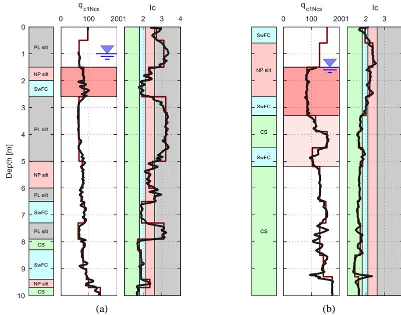
Figure 2. Typical  $q_{c1Ncs}$  and  $I_c$  profiles in (a) Papanui and (b) Avondale.
