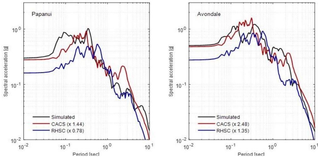
Figure 5. Acceleration response spectra of the base motions used in the probabilistic effective stress analyses.
