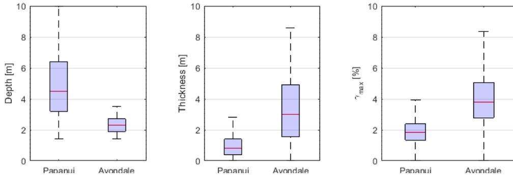
Figure 8. Variation in depth and thickness of the liquefied zone, and severity of liquefaction ( $\gamma_{max}$ ).
