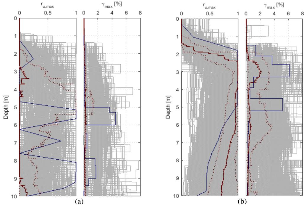
Figure 7. Variation in maximum excess pore pressure ratio  $r_{u,max}$  and maximum shear strain  $\gamma_{max}$  profiles for (a) Papanui and (b) Avondale. The solid red lines indicate the median response profiles whereas the dotted red lines indicate the 25<sup>th</sup> and 75<sup>th</sup> percentiles. The solid blue lines indicate the response profiles from the deterministic analysis (section 5.2).
