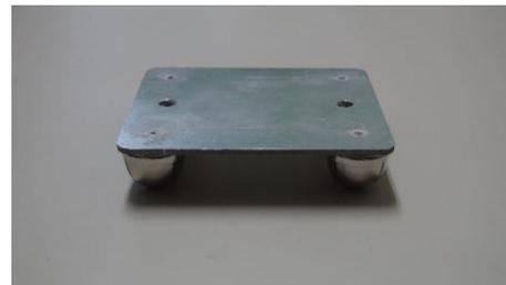
Figure 4. Base of accelerometer
