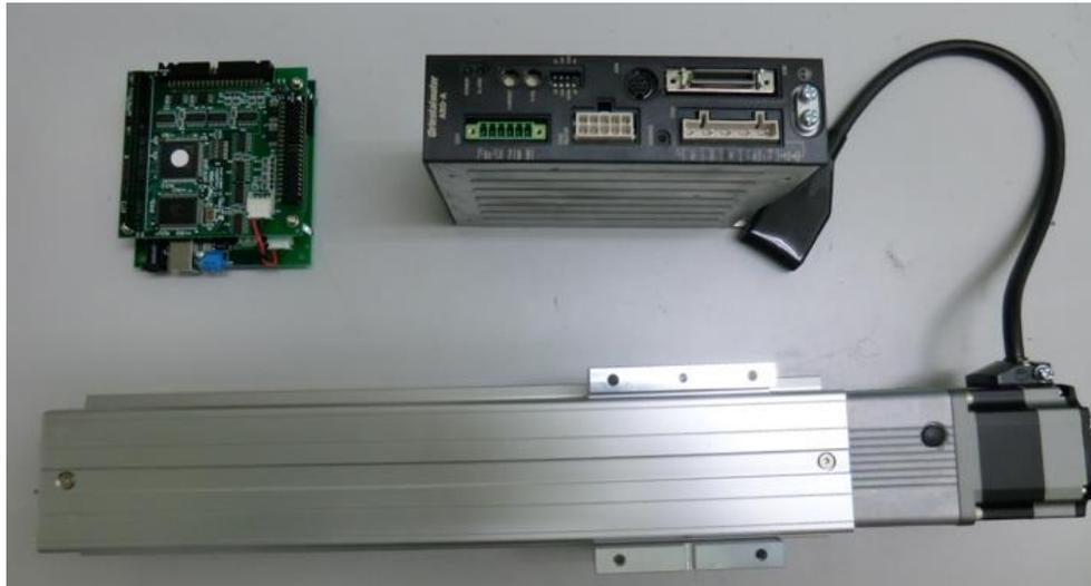
Figure 2. Motion controller (upper left), driver (upper right) and actuator (lower)
