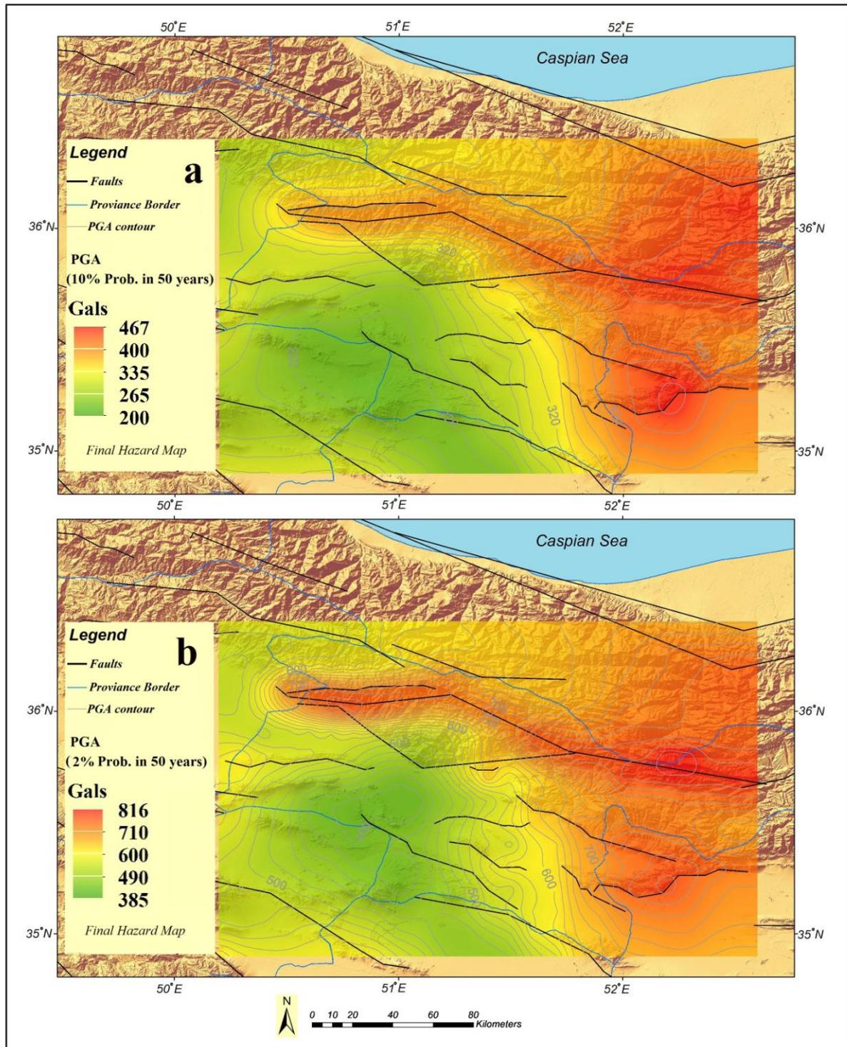
Figure 3. Final seismic hazard maps for PGA (in gal) obtained by combining background seismic activity and time-dependent characteristic earthquakes emanate from faults corresponding to a return period of (a) 475 and (b) 2475 year
