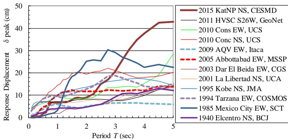
Fig. 5 Inelastic Response Displacement Spectra of 2015 Nepal Earthquake and other records ( $q_{Cy}=0.1, h=0.05$ )
