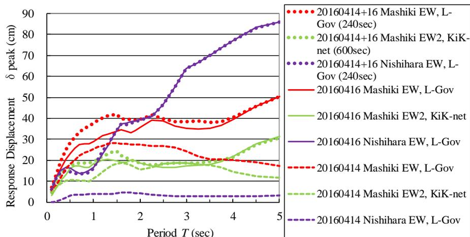
Fig. 4 Inelastic Response Displacement Spectra of 2016 Kumamoto Earthquake Main shock and Foreshock, 2016 Main shock or 2016 Foreshock ( $q_{Cy}=0.2, h=0.05$ )
