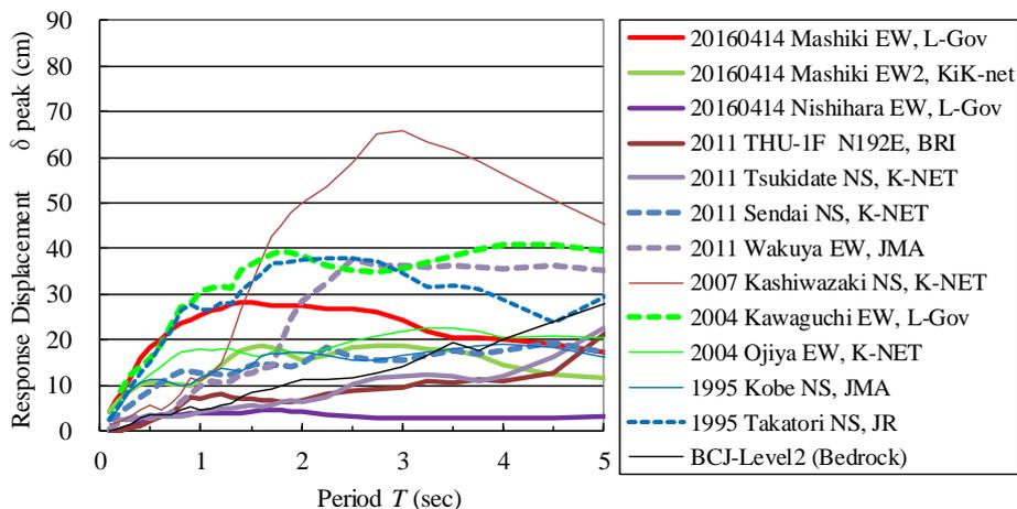
Fig. 3 Inelastic Response Displacement Spectra of 2016 Kumamoto Earthquake Foreshock and other records ( $q_{Cy}=0.2, h=0.05$ )
