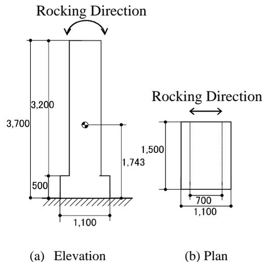
Fig.7 Rocking Specimen (Reinforced concrete column on concrete slab)
