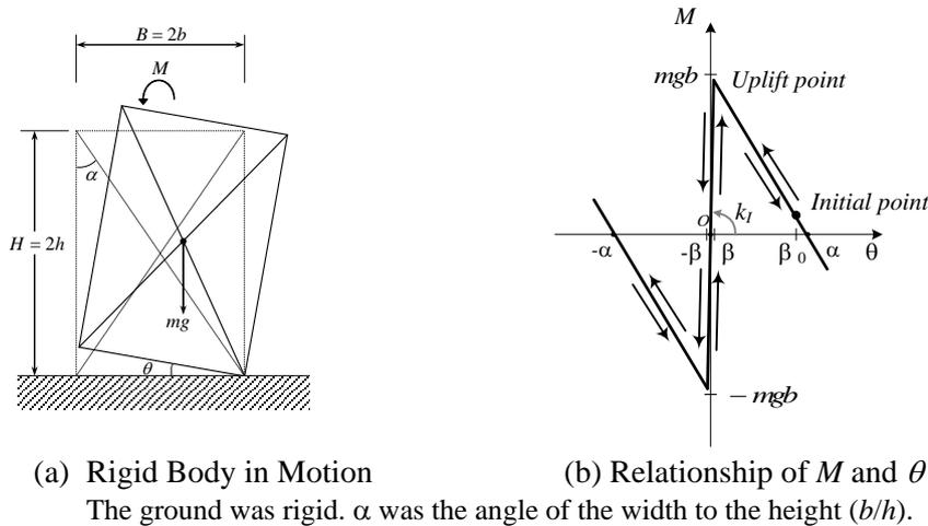
Fig. 6 Rigid Body in Motion and the Relationship between the internal moment  $M$  of the centre of the gravity and the rotation angle of rocking  $\theta$  when the ground was rigid
