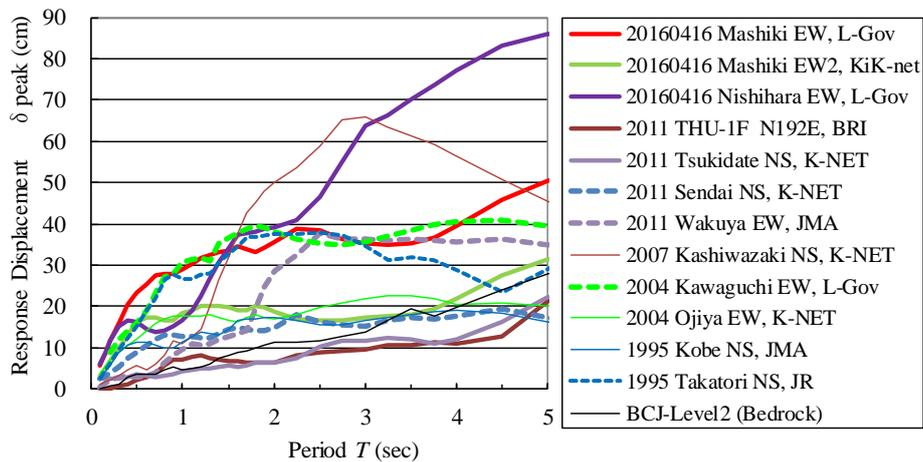
Fig. 2 Inelastic Response Displacement Spectra of 2016 Kumamoto Earthquake Main shock and other records ( $q_{Cy}=0.2, h=0.05$ )
