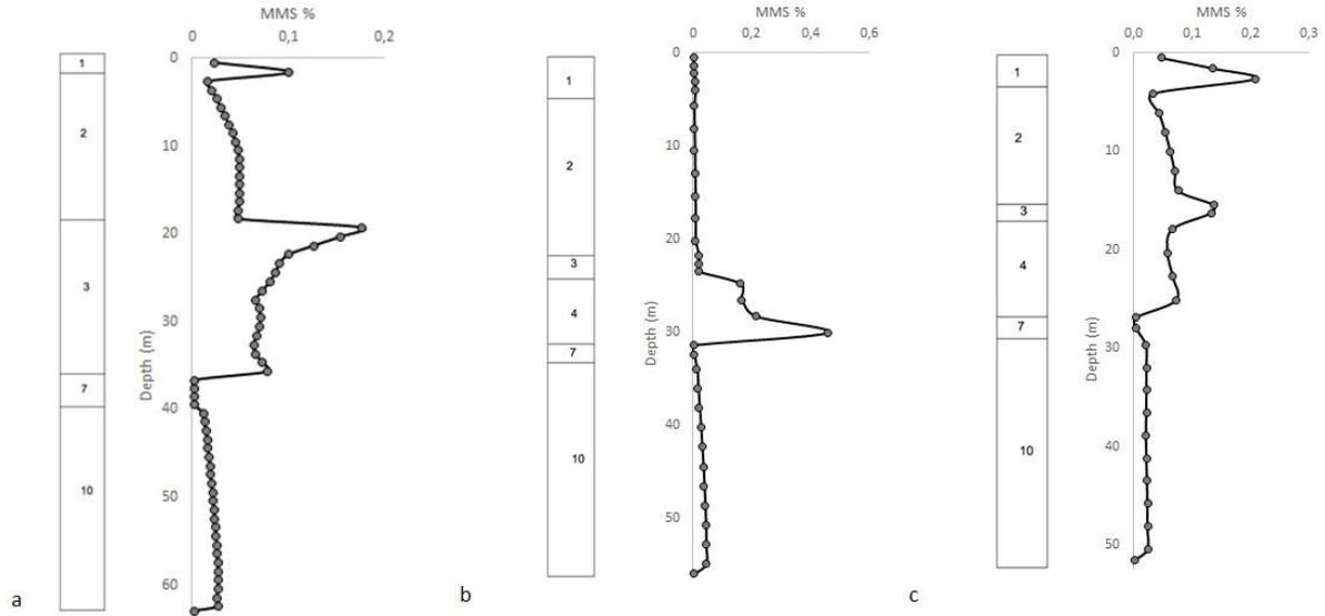
Figure 3. Distributions of the MSS versus depth assuming 1D condition in three of the 56 modelled soil columns. Plots on the left of each MSS curve show the distribution of soil materials along depth for each soil column. Refer to Fig. 2 and Table 1 for the description of the various lithologies.
