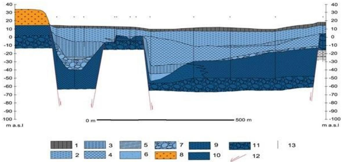
Figure 2. Geological cross section considered in this paper. Legend: AL deposits: from 1 to 7. VL deposits: 8. PT deposits: from 9 to 11. 12) Fault. 13) Borehole (modified from Bozzano et al. 2016). Refer to Table 1 below for further explanations on the various lithologies composing the cross section.
