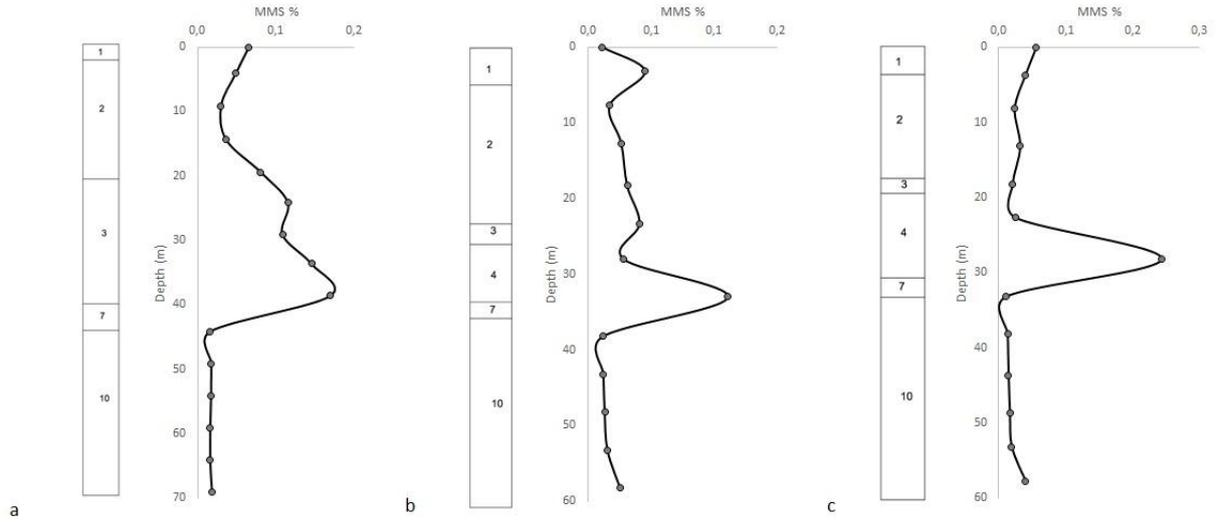
Figure 4. Distribution of the MSS versus depth assuming 2D condition in three of the 56 modelled soil columns.
