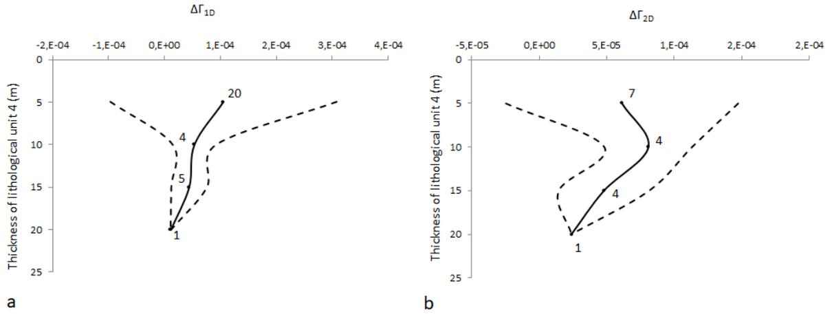
Figure 5.  $\Delta\Gamma$  distributions vs. thickness of lithological unit 4 in 1D (a) and 2D (b) models. Black line indicates the average values; dotted lines indicate the computed standard deviations. The number of data available for computing the average is also shown in the plots.
